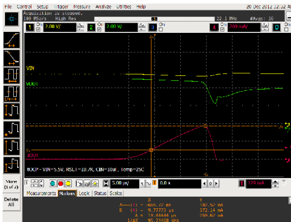
Figure 11. t_{OCP} Response Time
