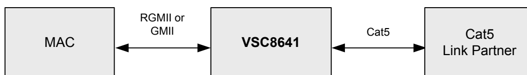
Figure 3. RGMII or GMII to Cat5 Block Diagram
