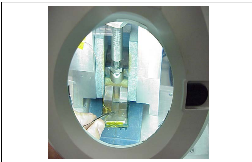
Figure 7-29. Moving Solder back onto Thermocouple Bead
