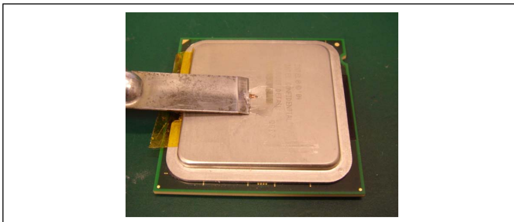
Figure 7-35. Removing Excess Adhesive from IHS
