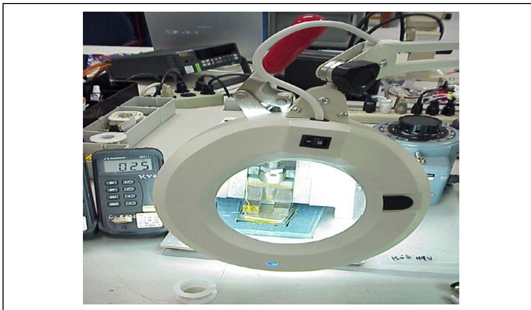
Figure 7-29. Moving Solder back onto Thermocouple Bead
