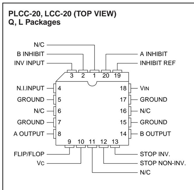
Note: All four ground pins must be connected to a common ground.
