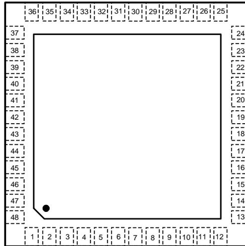
**Figure 1. 48 WQFN Package (Top View)
