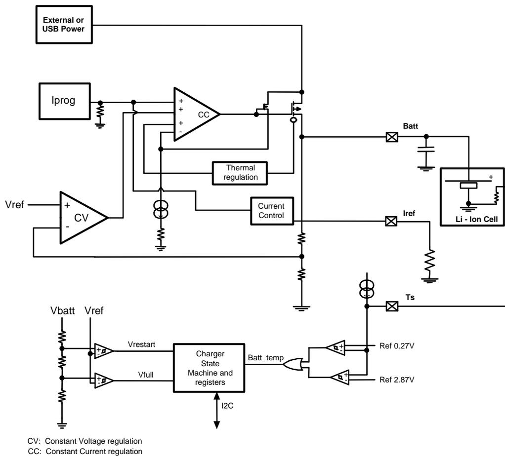
The charger module is a linear charger with constant current pre-qualification, constant current (“CC”) full-rate charging and constant voltage (“CV”) charging. CC and CV regulation is performed using an internal Power FET Q2 with reverse current blocking. The termination voltage is controlled to within  $\pm 0.35\%$  at room temperature.
