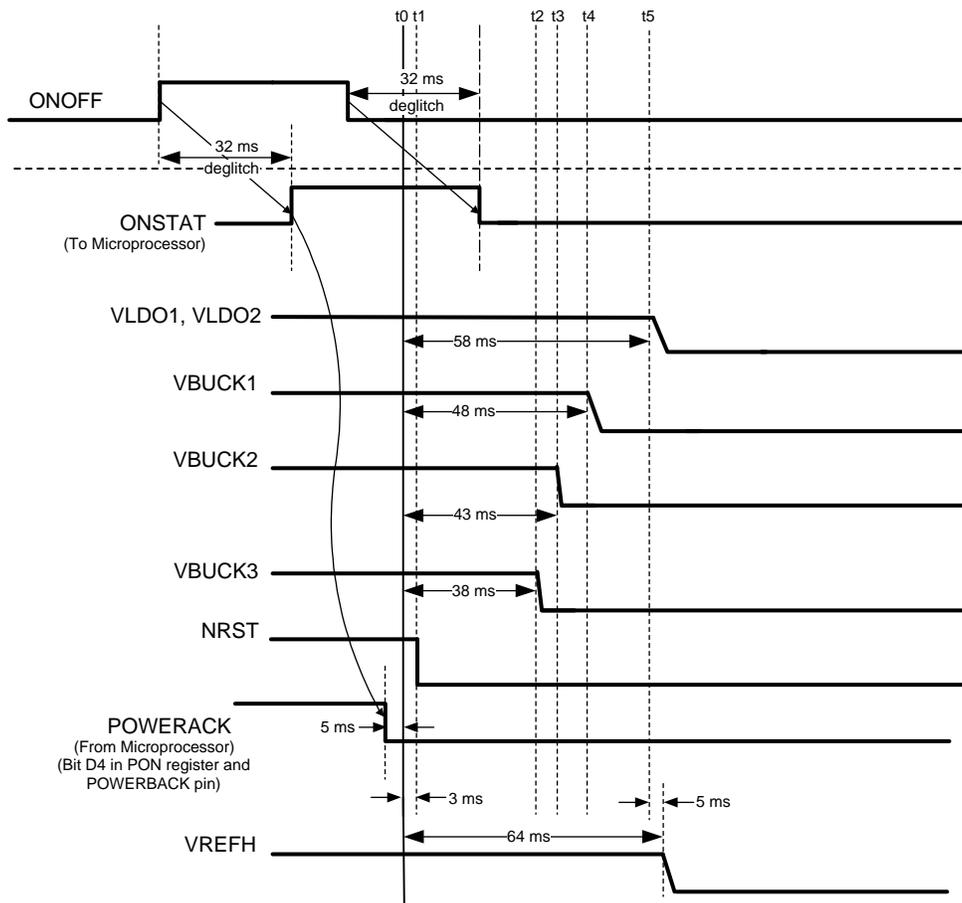
**Transition from Active to Standby Mode Due to Expiring POWERACK Deadline**
