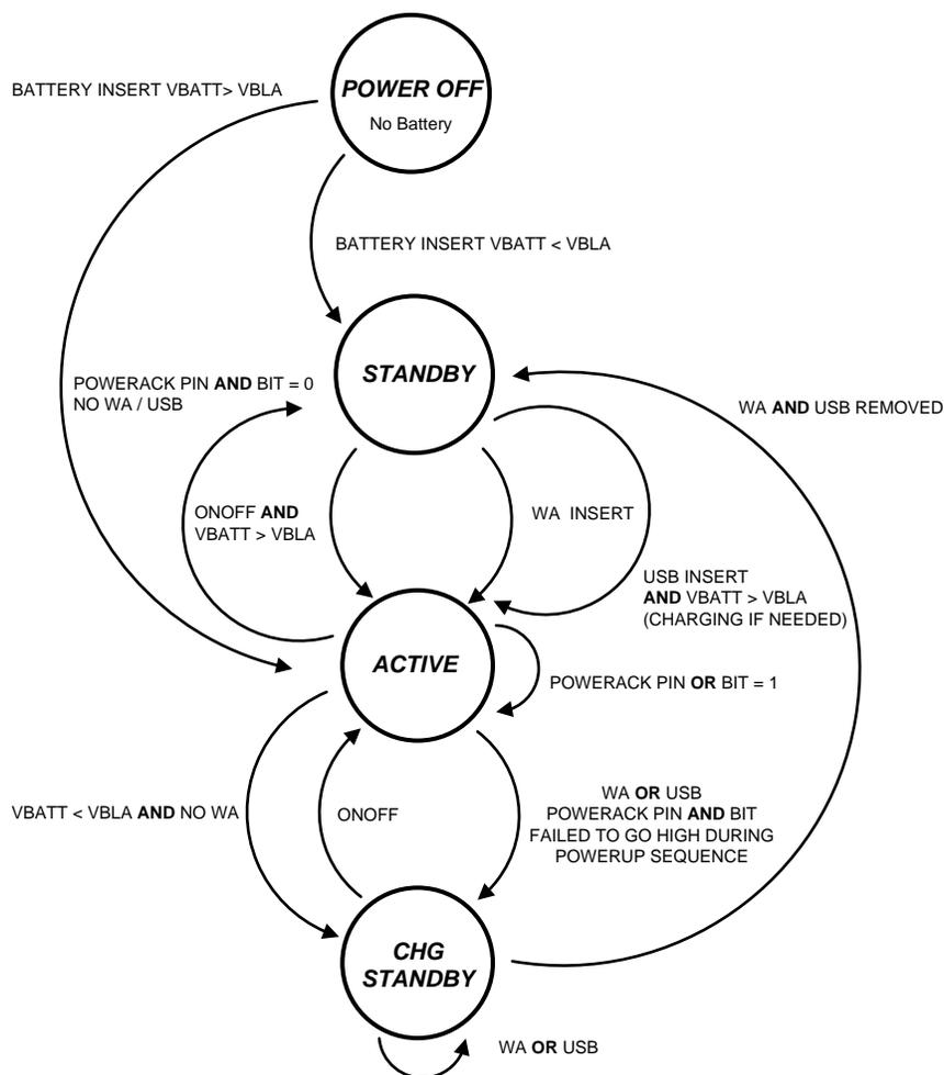
Figure 53. Operating Mode State Diagram
