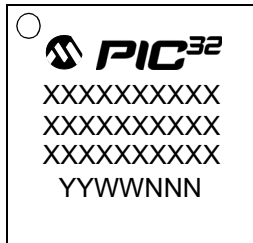
64-Lead TQFP (10x10x1 mm)
