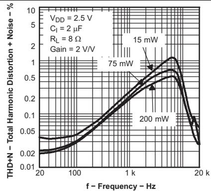
Figure 18. Total Harmonic Distortion + Noise vs Frequency
