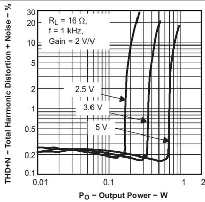
Figure 15. Total Harmonic Distortion + Noise vs Output Power
