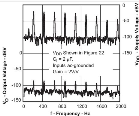
Figure 29. GSM Power Supply Rejection vs Frequency
