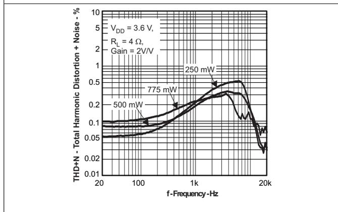
Figure 21. Total Harmonic Distortion + Noise vs Frequency
