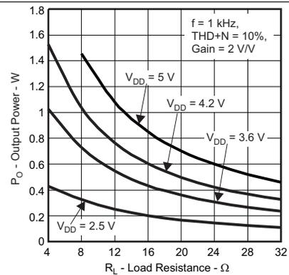
Figure 12. Output Power vs Load Resistance
