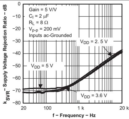
Figure 25. Supply Voltage Rejection Ratio vs Frequency 25
