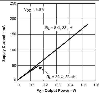
Figure 5. Supply Current vs Output Power
