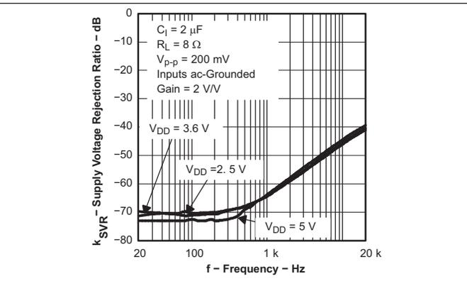
Figure 24. Supply Voltage Rejection Ratio vs Frequency
