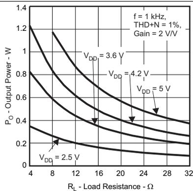
Figure 11. Output Power vs Load Resistance
