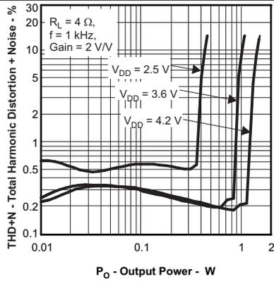
Figure 13. Total Harmonic Distortion + Noise vs Output Power
