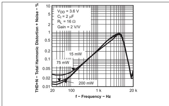
Figure 19. Total Harmonic Distortion + Noise vs Frequency
