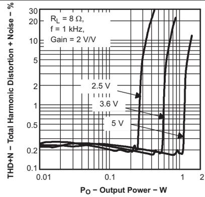
Figure 14. Total Harmonic Distortion + Noise vs Output Power
