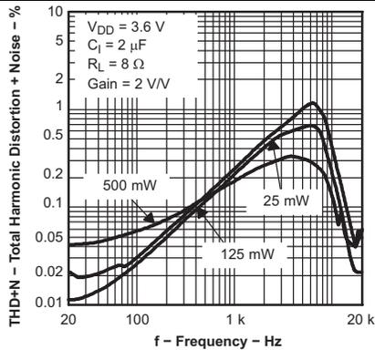
Figure 17. Total Harmonic Distortion + Noise vs Frequency
