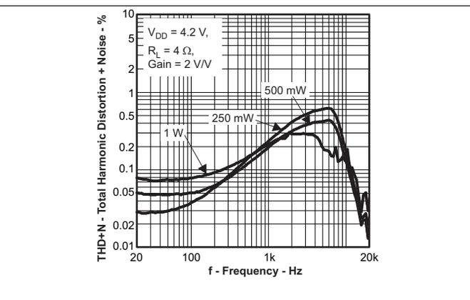
Figure 20. Total Harmonic Distortion + Noise vs Frequency
