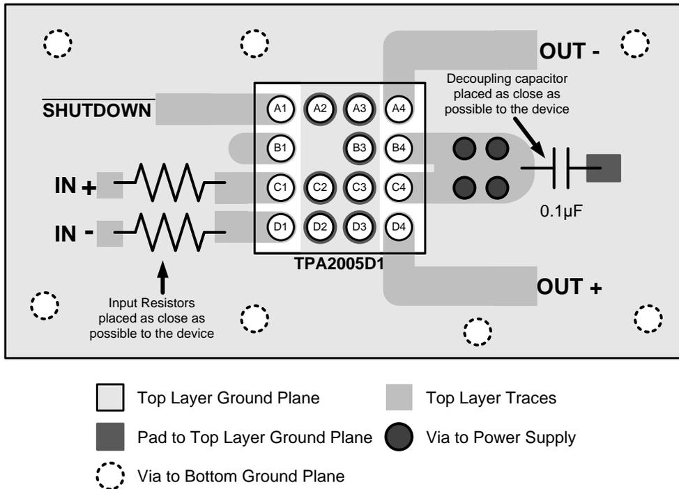
Figure 45. TPA2005D1 MicroStar Junior™ BGA Package Layout Example
