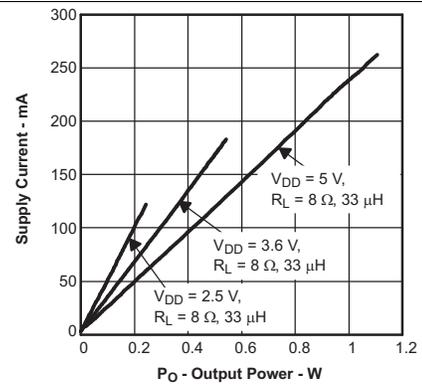
Figure 6. Supply Current vs Output Power
