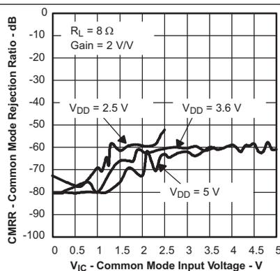
Figure 31. Common-mode Rejection Ratio vs Common-mode Input Voltage
