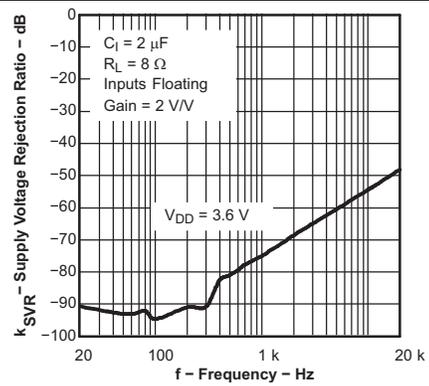
Figure 26. Supply Voltage Rejection Ratio vs Frequency
