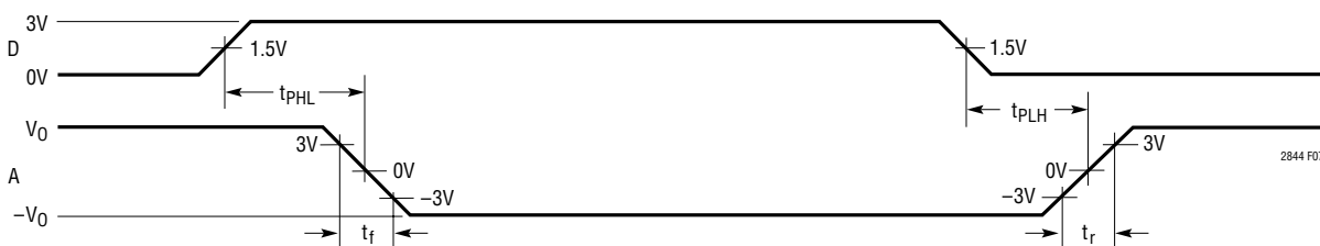
Figure 7. V.10, V.28 Driver Propagation Delays
