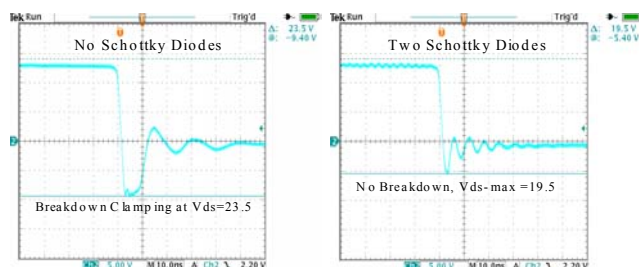
FIGURE 40. EFFECT OF ADDING TWO SCHOTTKY DIODES ON THE VDS OF THE HIGH SIDE SWITCH
