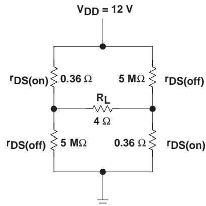
**Figure 9. Output Transistor Simplification for Conduction Loss Calculation**
