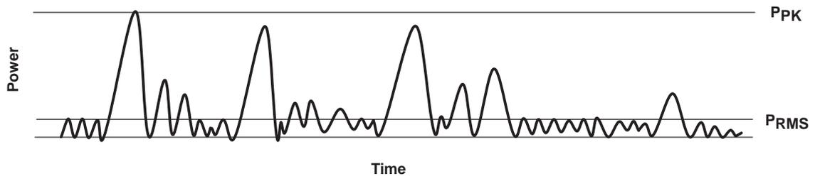
**Figure 11. Audio Signal Showing Peak and RMS Power**
