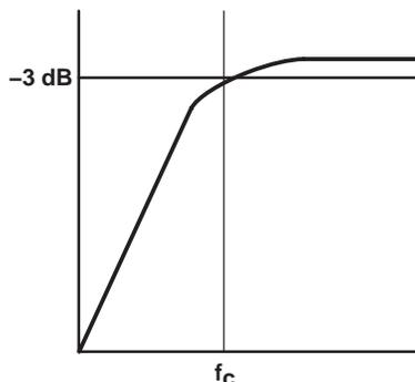
The value of  $C_1$  is important to consider as it directly affects the bass (low frequency) performance of the circuit. Consider the example where the specification calls for a flat bass response down to 40 Hz. Equation 8 is reconfigured as equation 9.
