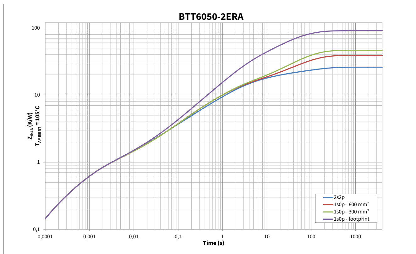
Figure 6 Typical Thermal Impedance - 2s2p set-up according to Figure 4
