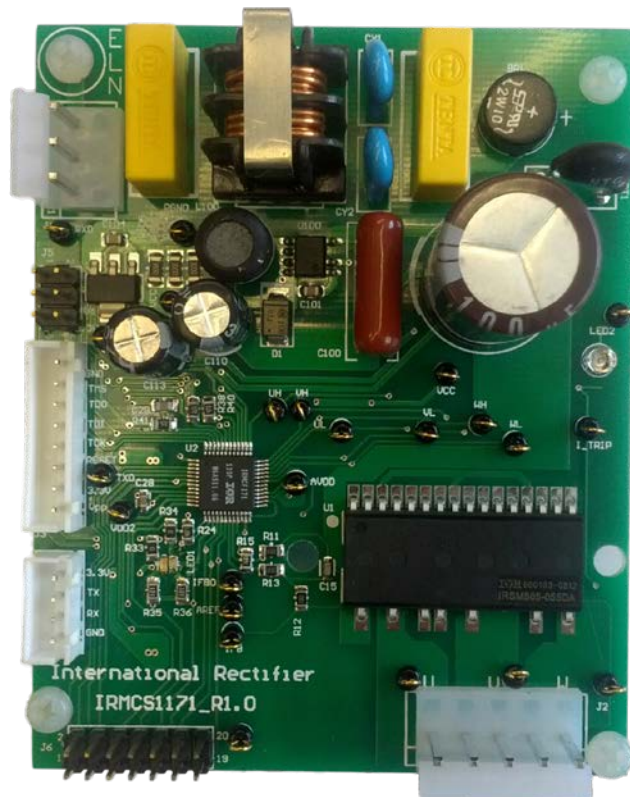
Figure 4: Reference design board featuring the µPM™-DIP module and the iMotion™ IRMCF171 digital control IC
