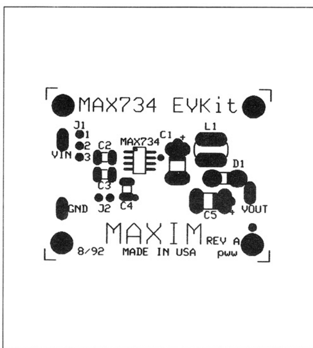
Figure 5. Component Placement Diagram (1x Scale)
