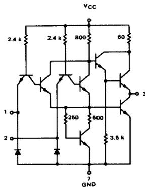
This device consists of four 2-input NOR gates. Each gate may be used as an inverter, or two gates may be cross-coupled to form bistable circuits.
