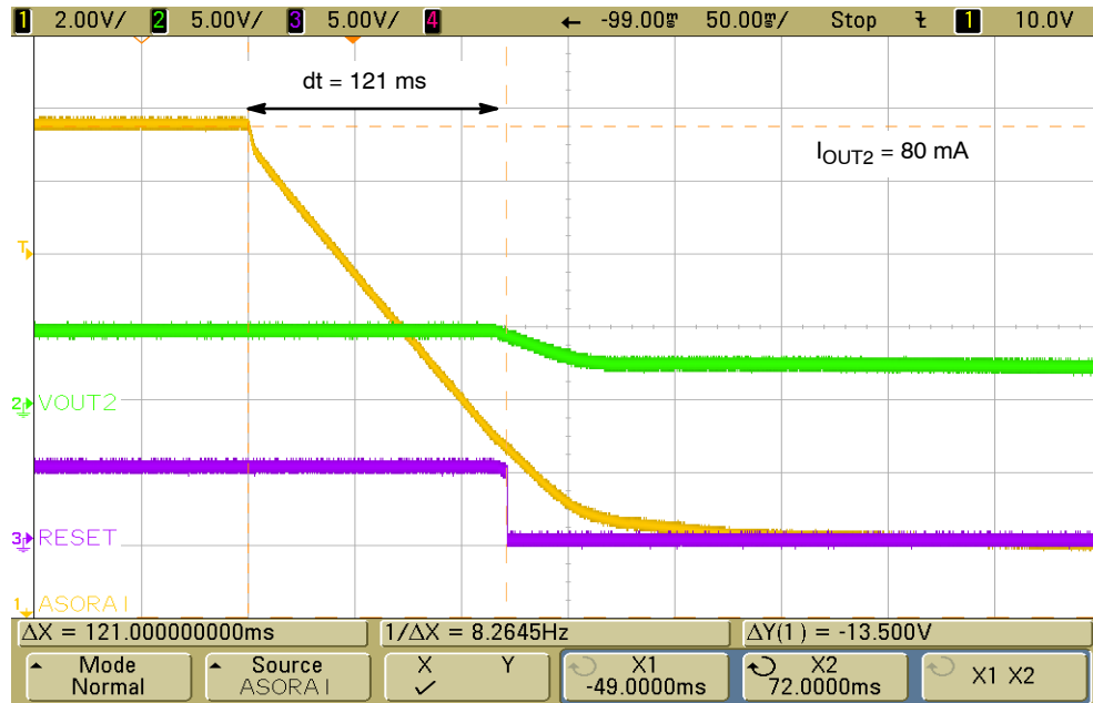
Figure 27. Output Response of LDO2 to Loss of Vin-B
