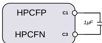
Figure 41: Charge pump flying capacitor
