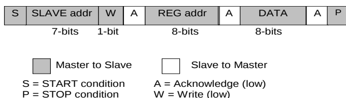
Figure 27: I 2 C byte write (SDA signal)
