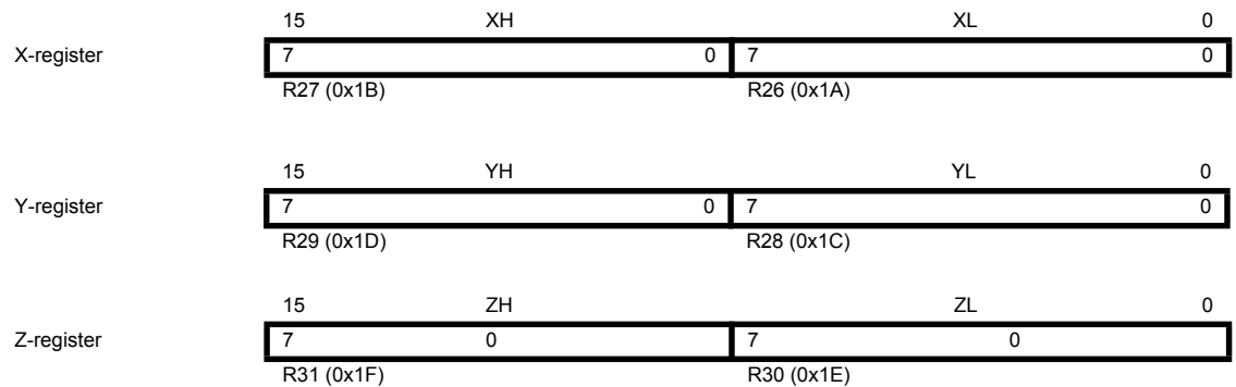
Figure 6-3. The X-, Y-, and Z-registers
