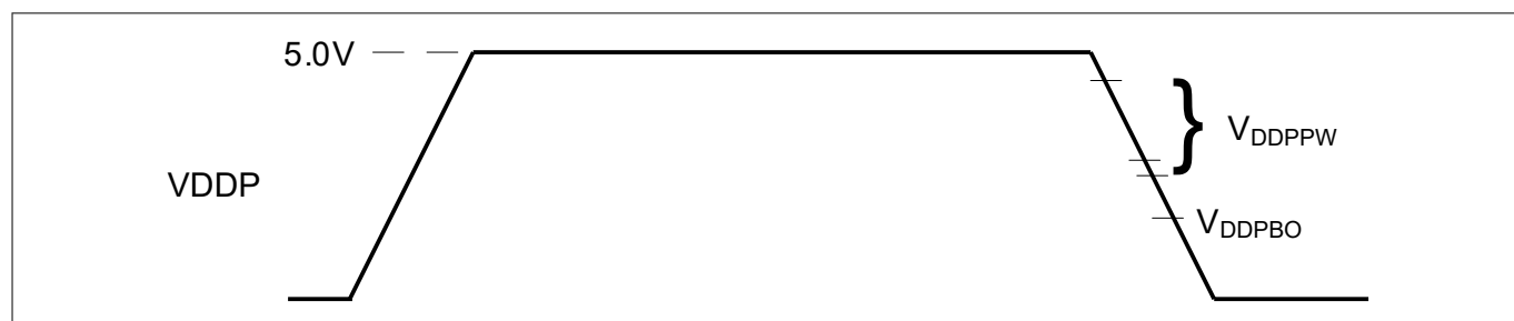
Figure 16 Supply Threshold Parameters
