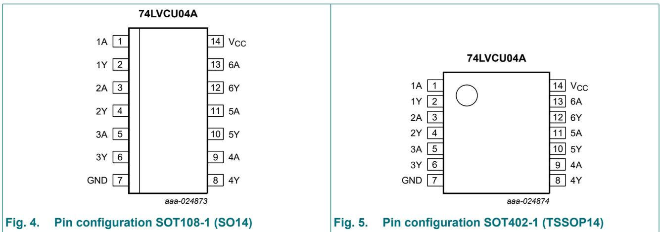
Fig. 4. Pin configuration SOT108-1 (SO14)
