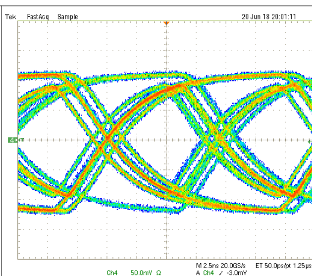
Figure 6-12. Typical 50 Mbps Back Channel Output Waveform
