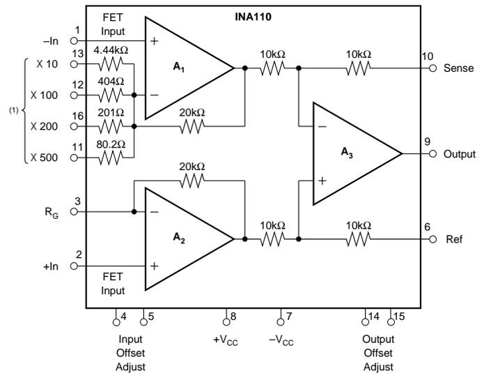
NOTE: (1) Connect to  $R_G$  for desired gain.
