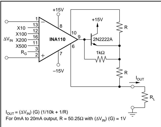
FIGURE 17. Differential Input FET Buffered Current Source.
