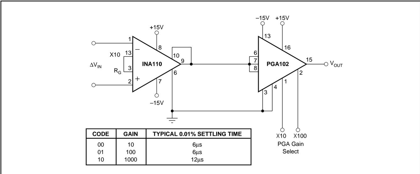
FIGURE 16. Digitally-Controlled Fast-Settling Programmable Gain Instrumentation Amplifier.
