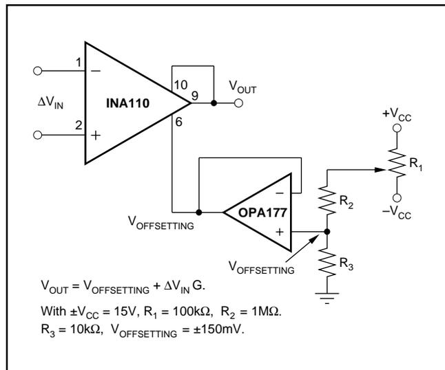
FIGURE 3. Output Offsetting.
