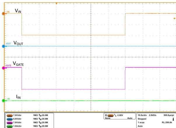
Figure 9-9. Reverse Input Voltage -14 V for 60 s
