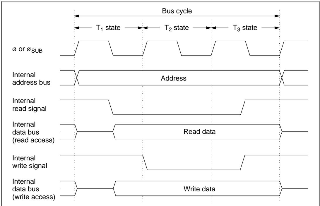
**Figure 2.13 On-Chip Peripheral Module Access Cycle (3-State Access)**
