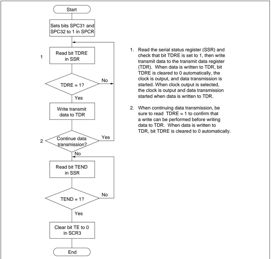
1. Read the serial status register (SSR) and check that bit TDRE is set to 1, then write transmit data to the transmit data register (TDR). When data is written to TDR, bit TDRE is cleared to 0 automatically, the clock is output, and data transmission is started. When clock output is selected, the clock is output and data transmission started when data is written to TDR.
