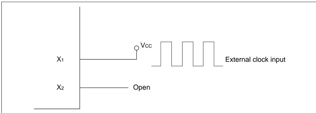
**Figure 4.10 Pin Connection when Inputting External Clock**
