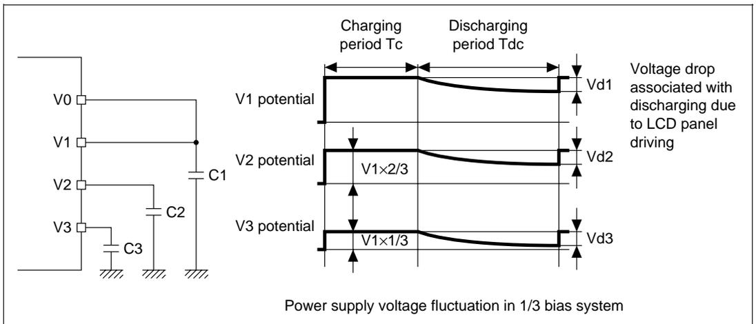
**Figure 13.14 Example of Low-Power-Consumption LCD Drive Operation**
