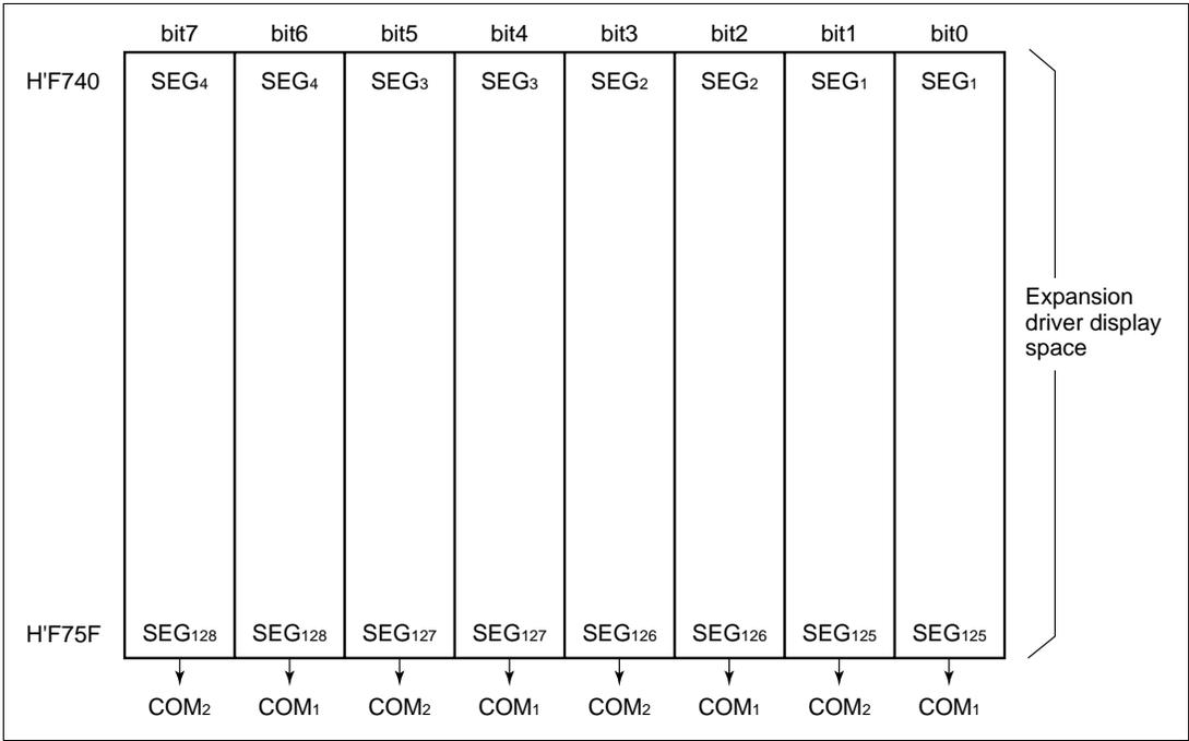
**Figure 13.11 LCD RAM Map when Using Segment External Expansion
