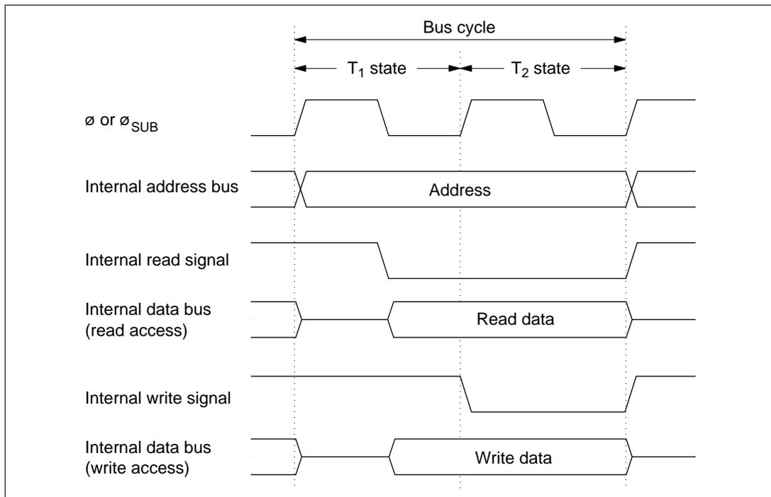
**Figure 2.12 On-Chip Peripheral Module Access Cycle (2-State Access)**
