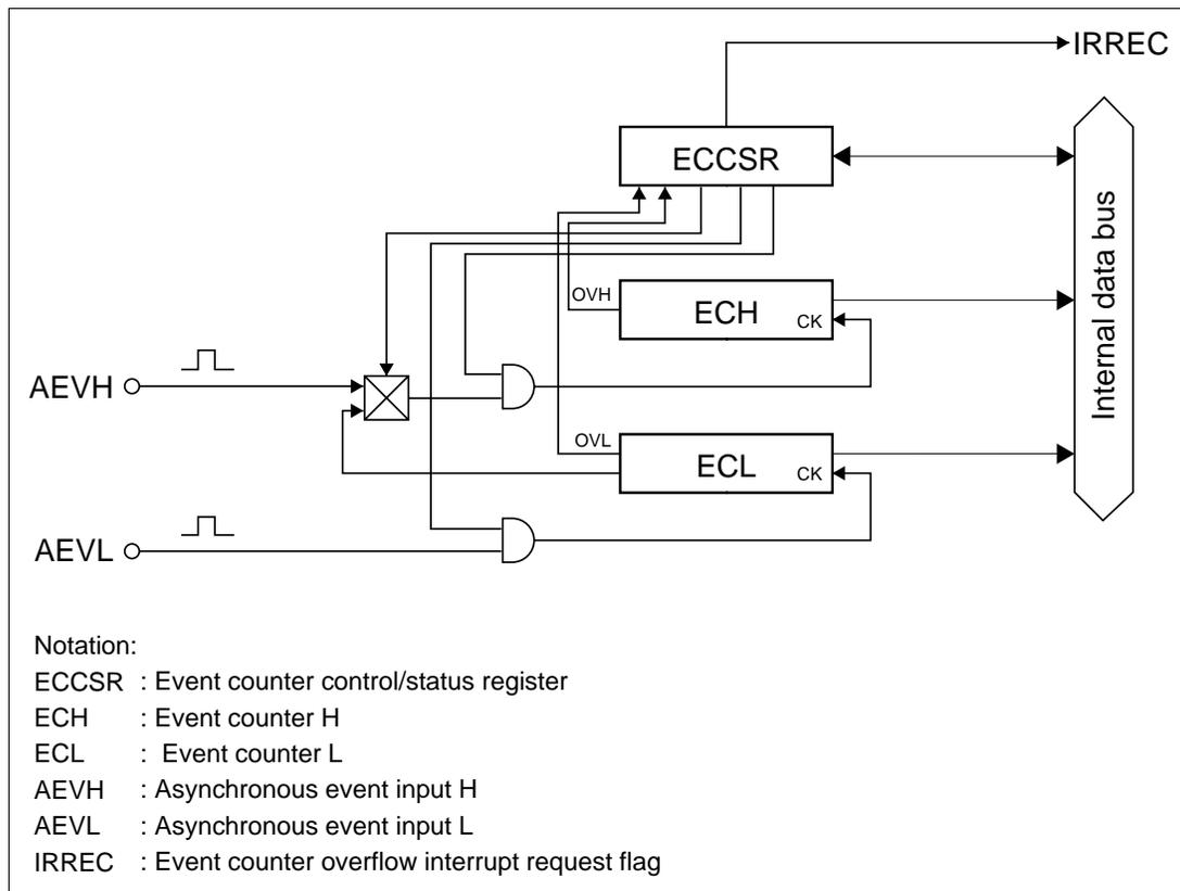
**Figure 9.18 Block Diagram of Asynchronous Event Counter**
