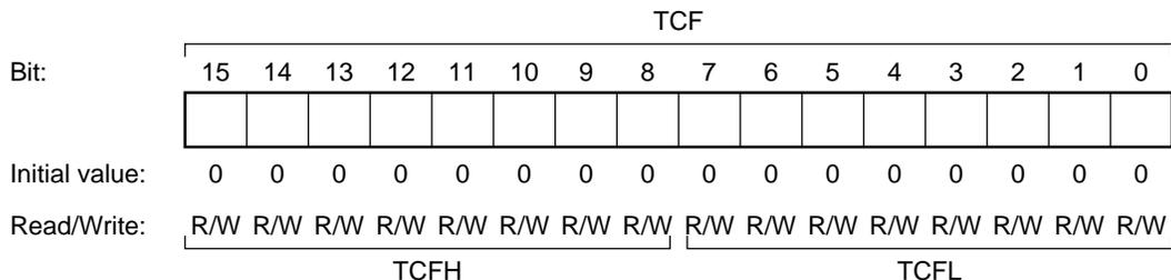
TCF is a 16-bit read/write up-counter configured by cascaded connection of 8-bit timer counters TCFH and TCFL. In addition to the use of TCF as a 16-bit counter with TCFH as the upper 8 bits and TCFL as the lower 8 bits, TCFH and TCFL can also be used as independent 8-bit counters.
