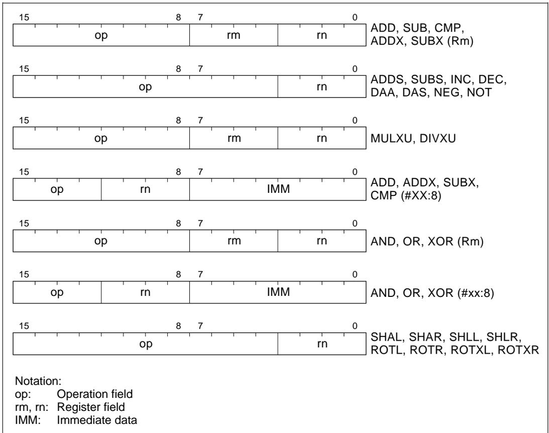
**Figure 2.6 Arithmetic, Logic, and Shift Instruction Codes**
