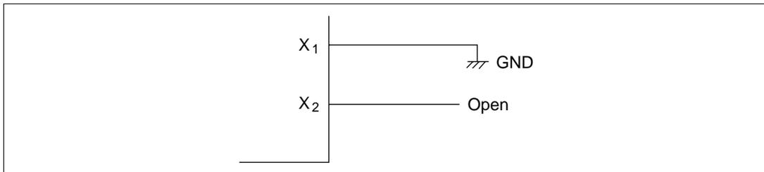
**Figure 4.9 Pin Connection when not Using Subclock**
