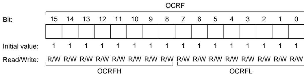
OCRF is a 16-bit read/write register composed of the two registers OCRFH and OCRFL. In addition to the use of OCRF as a 16-bit register with OCRFH as the upper 8 bits and OCRFL as the lower 8 bits, OCRFH and OCRFL can also be used as independent 8-bit registers.
