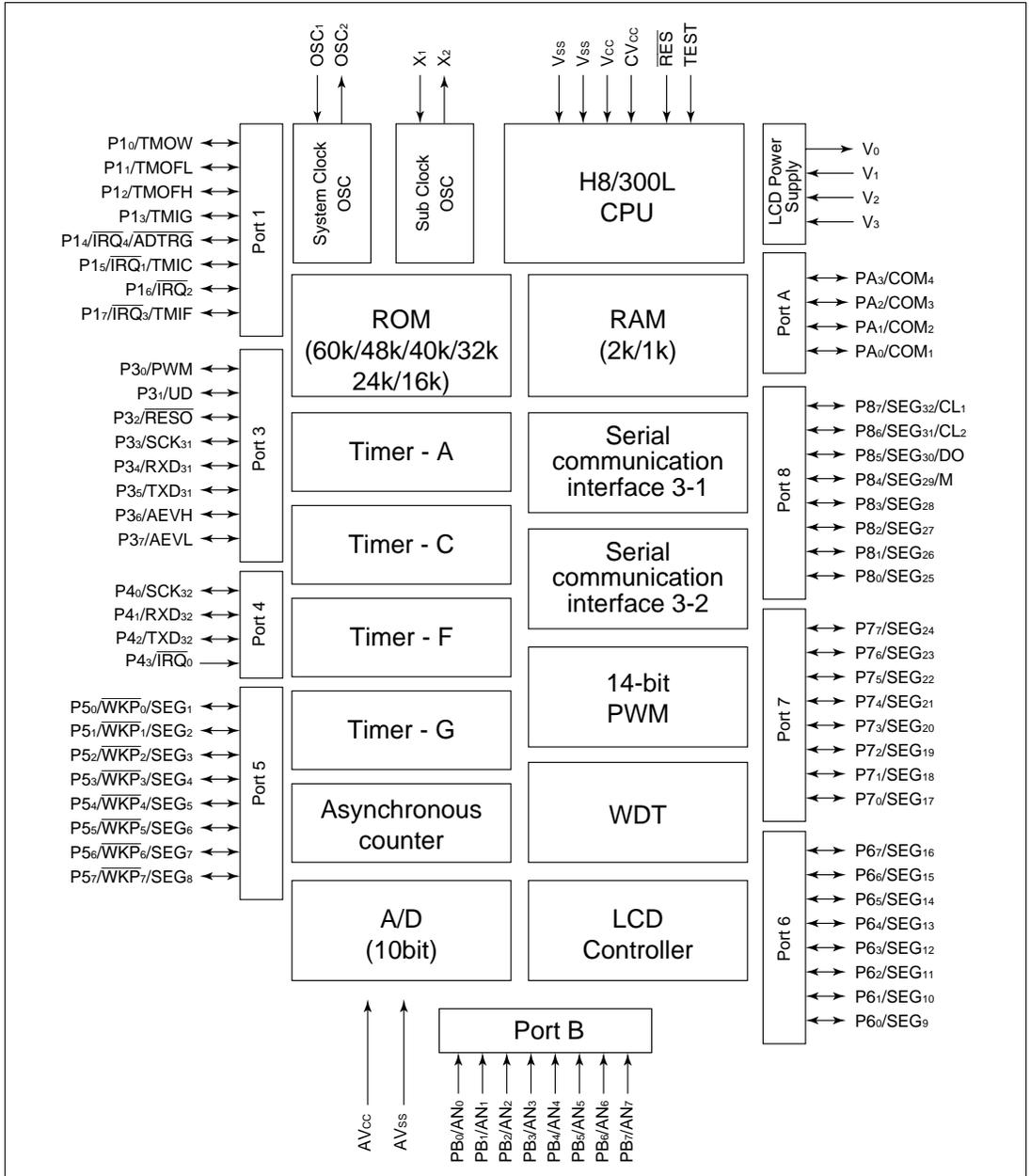
Figure 1.1 Block Diagram
