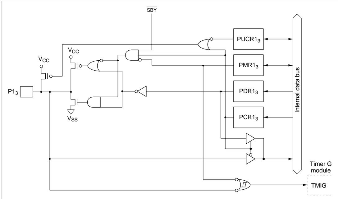
**Figure C.1 (b) Port 1 Block Diagram (Pin P1<sub>3</sub>)**
