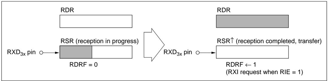
**Figure 10.2 (a) RDRF Setting and RXI Interrupt**
