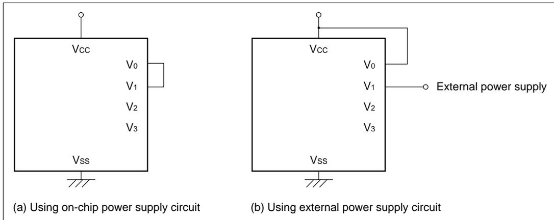
**Figure 13.4 Examples of LCD Power Supply Pin Connections**
