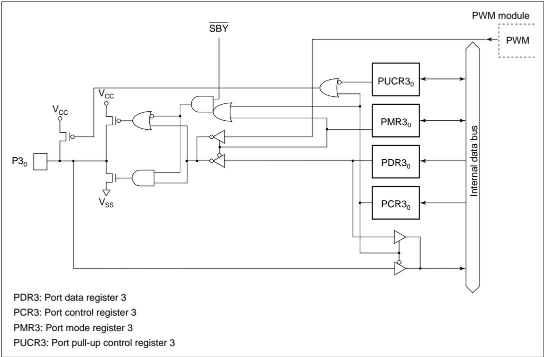
**Figure C.2 (g) Port 3 Block Diagram (Pin P3<sub>0</sub>)**
