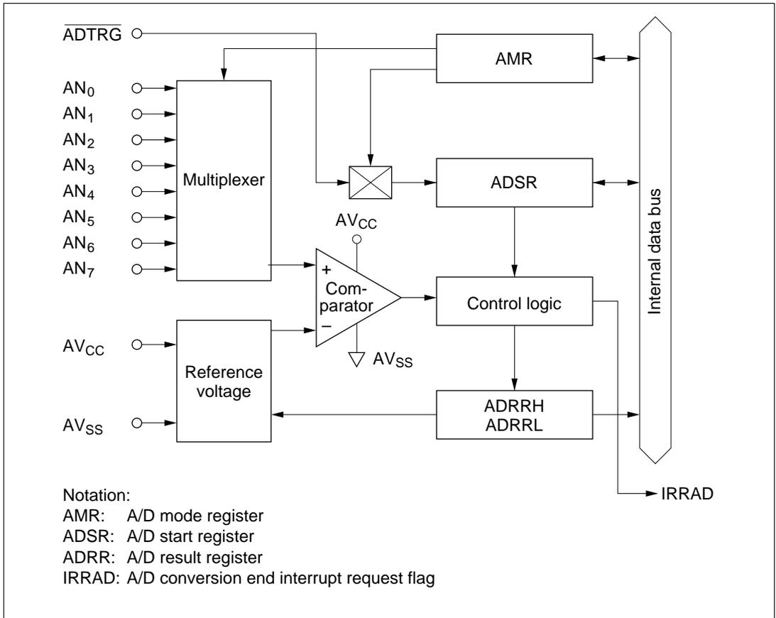
**Figure 12.1** Block Diagram of the A/D Converter
