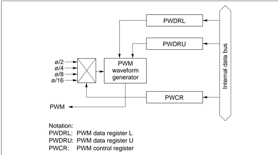
**Figure 11.1 Block Diagram of the 14-bit PWM**
