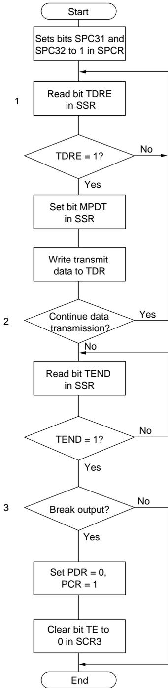
1. Read the serial status register (SSR) and check that bit TDRE is set to 1, then set bit MPBT in SSR to 0 or 1 and write transmit data to the transmit data register (TDR). When data is written to TDR, bit TDRE is cleared to 0 automatically.
