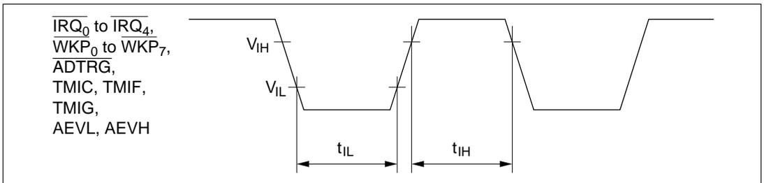
Figure 15.3 Input Timing
