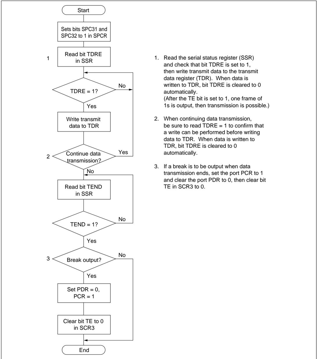
1. Read the serial status register (SSR) and check that bit TDRE is set to 1, then write transmit data to the transmit data register (TDR). When data is written to TDR, bit TDRE is cleared to 0 automatically.
