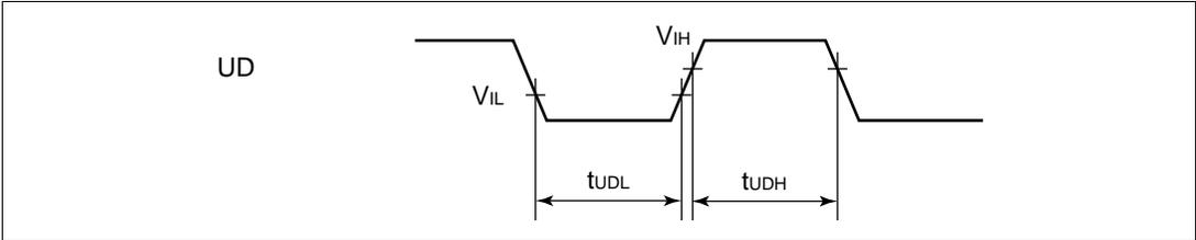
**Figure 15.4 UD Pin Minimum Modulation Width Timing**
