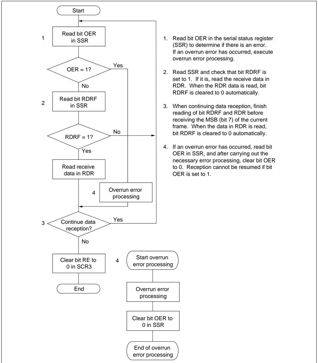
Figure 10.13 Example of Data Reception Flowchart (Synchronous Mode)
