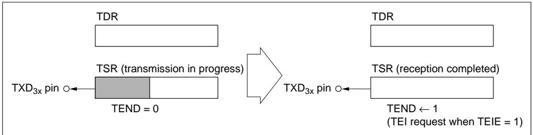
**Figure 10.2 (c) TEND Setting and TEI Interrupt**
