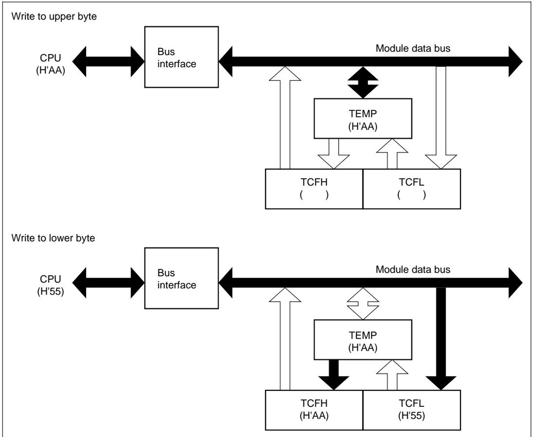
**Figure 9.4 Write Access to TCF (CPU  $\neq$  TCF)**
