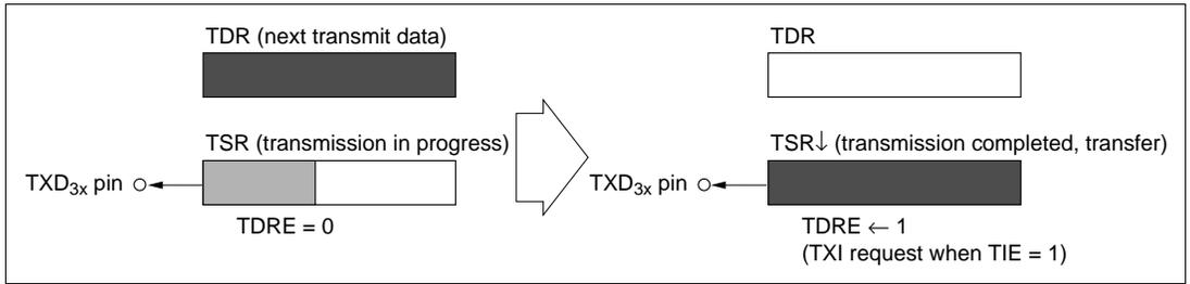
**Figure 10.2 (b) TDRE Setting and TXI Interrupt**
