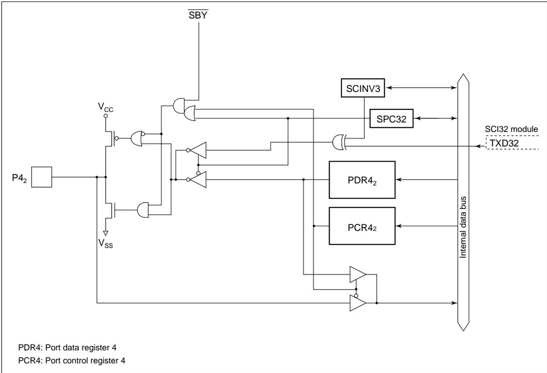
**Figure C.3 (b) Port 4 Block Diagram (Pin P4<sub>2</sub>)**
