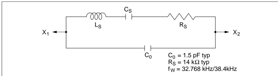
**Figure 4.8 Equivalent Circuit of 32.768-kHz/38.4 kHz Crystal Oscillator**
