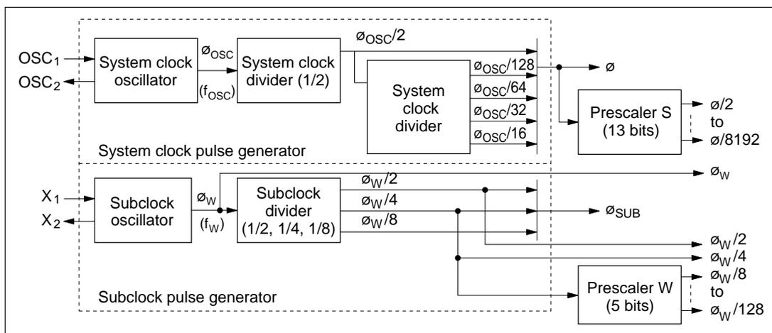
**Figure 4.1** Block Diagram of Clock Pulse Generators
