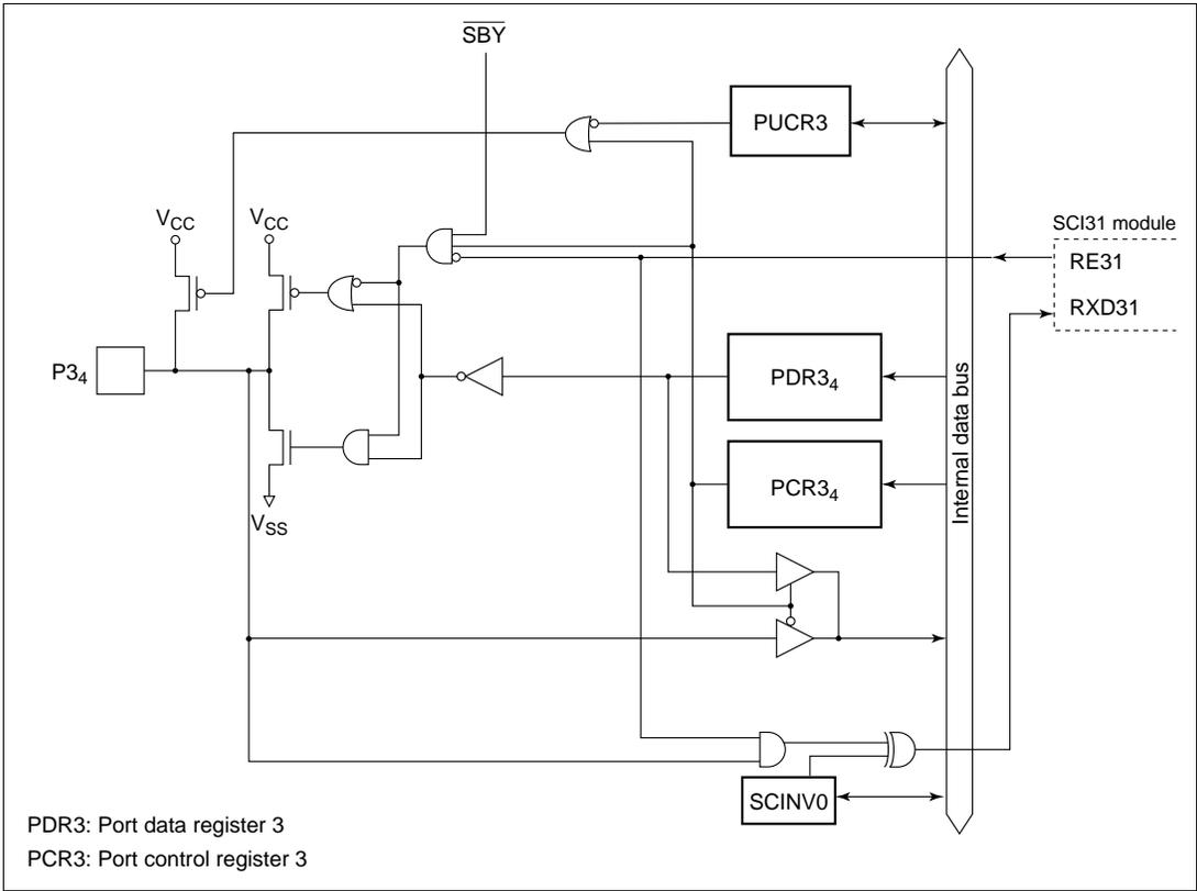
**Figure C.2 (c) Port 3 Block Diagram (Pin P34)**
