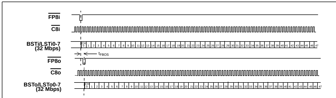
Figure 7 - Input and Output (Generated) Frame Pulse Alignment
