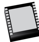
4mm x 5mm x 0.9mm DFN SMT Package
