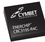
4mm x 5mm x 0.9mm DFN SMT Package
