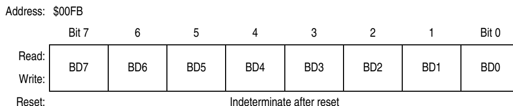
Figure 15-16. BDLC Data Register (BDR)
