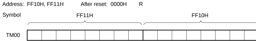
Figure 6-2. Format of 16-Bit Timer Counter 00 (TM00)
