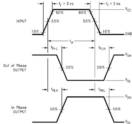
Figure 6. AC Waveforms
