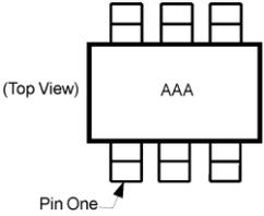
**Figure 4. Pin 1 Orientation**
