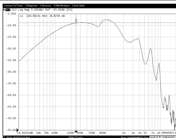
Figure 8-32. Off-State Data-Switch Isolation vs Frequency (TPS25830-Q1)
