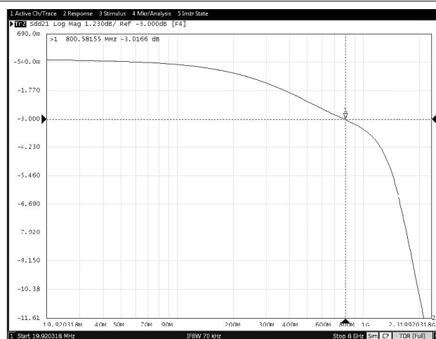
Figure 8-31. Data Transmission Characteristics vs Frequency (TPS25830-Q1)
