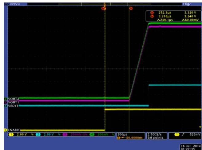
Figure 15: Loop 1 & Loop 2 start together with 0.25ms delay from Enable
