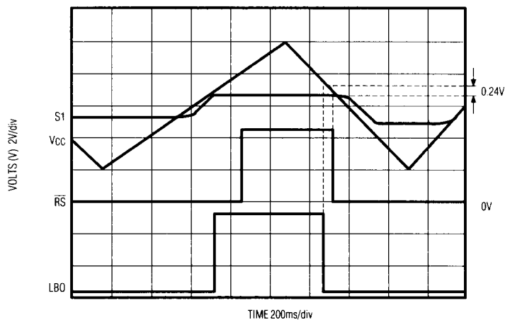
BACKUP-BATTERY SWITCHING AND WARNING FLAGS
