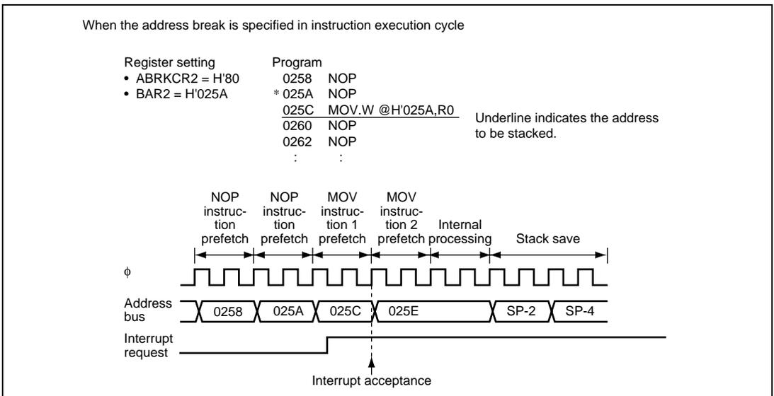
**Figure 23.2 Address Break Interrupt Operation Example (1)**
