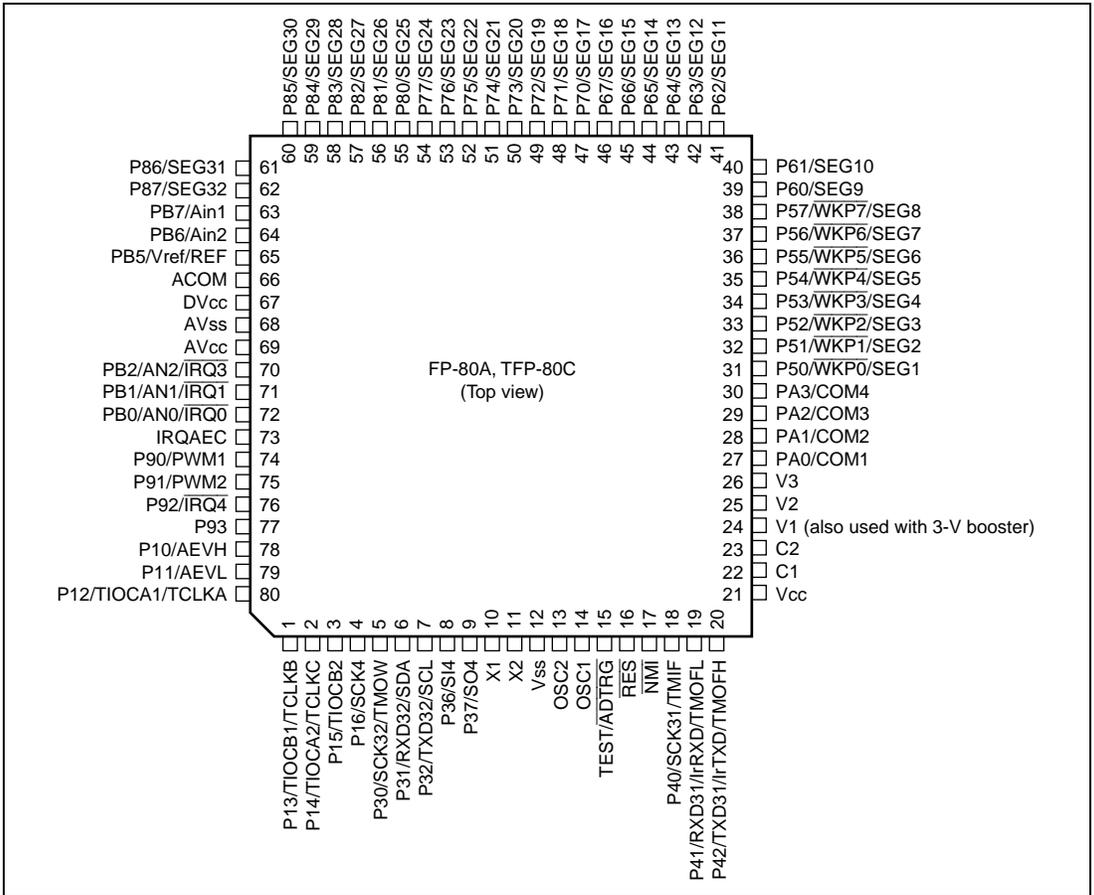
Figure 1.2 Pin Assignment of H8/38086R Group (FP-80A, TFP-80C)
