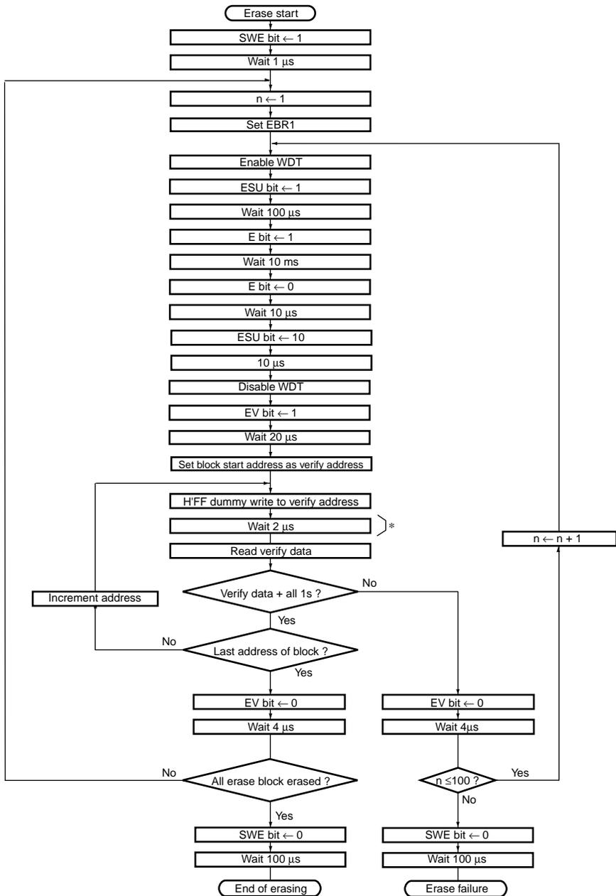
Note: \* The RTS instruction must not be used during a period between dummy writing of H'FF to a verify address and verify data reading.
