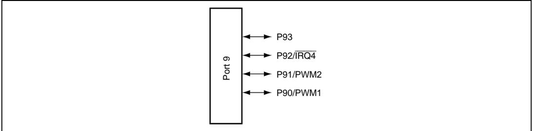
**Figure 9.8 Port 9 Pin Configuration**
