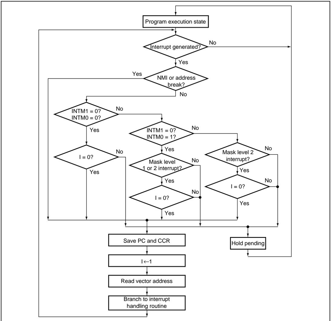
Figure 4.2 Flowchart of Procedure Up to Interrupt Acceptance
