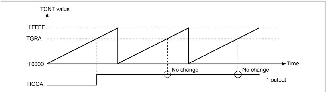
**Figure 12.9 Example of 0 Output/1 Output Operation**
