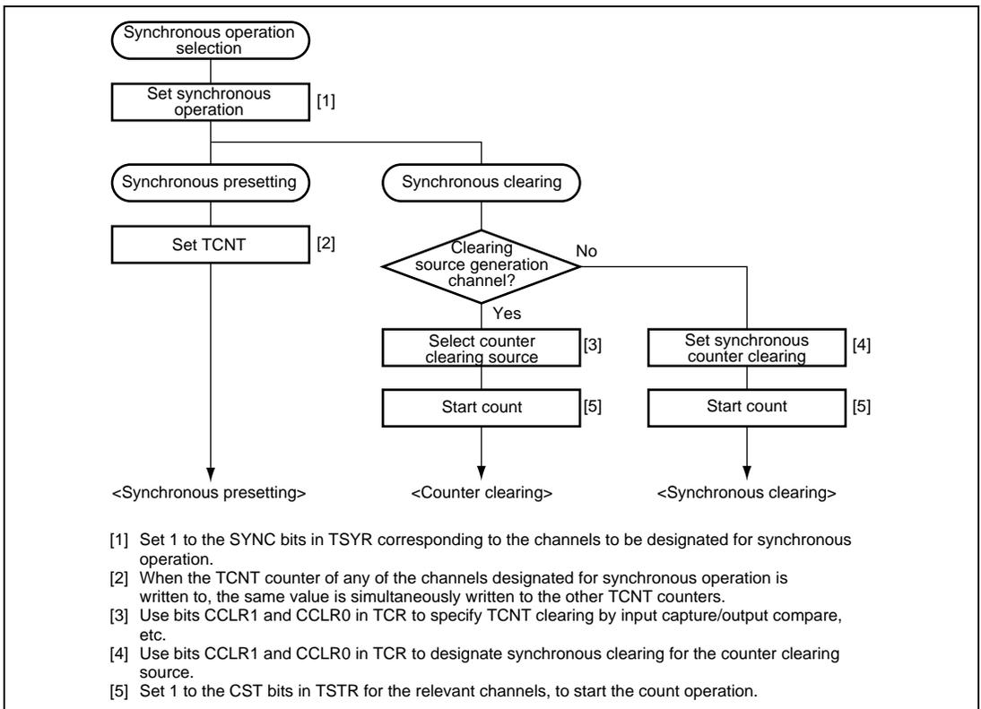
**Figure 12.13 Example of Synchronous Operation Setting Procedure**
