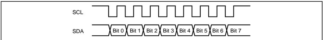
**Figure 21.13 Clocked Synchronous Serial Transfer Format**
