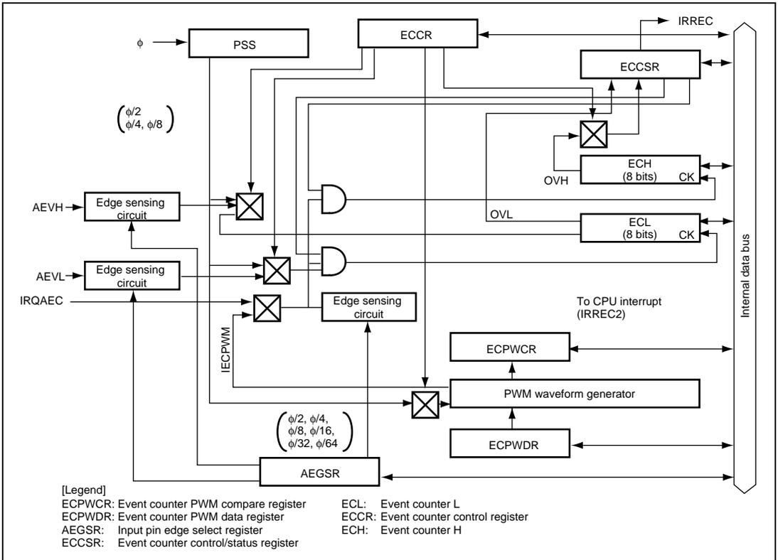
Figure 13.1 Block Diagram of Asynchronous Event Counter
