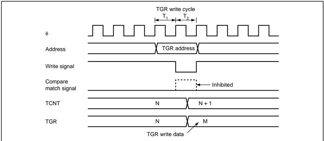
**Figure 12.33 Contention between TGR Write and Compare Match**
