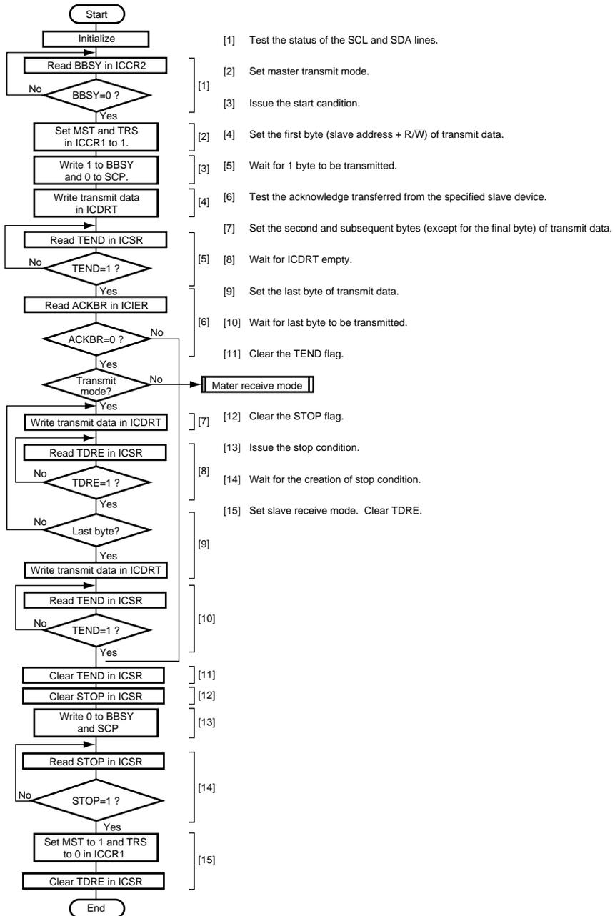
Figure 21.17 Sample Flowchart for Master Transmit Mode
