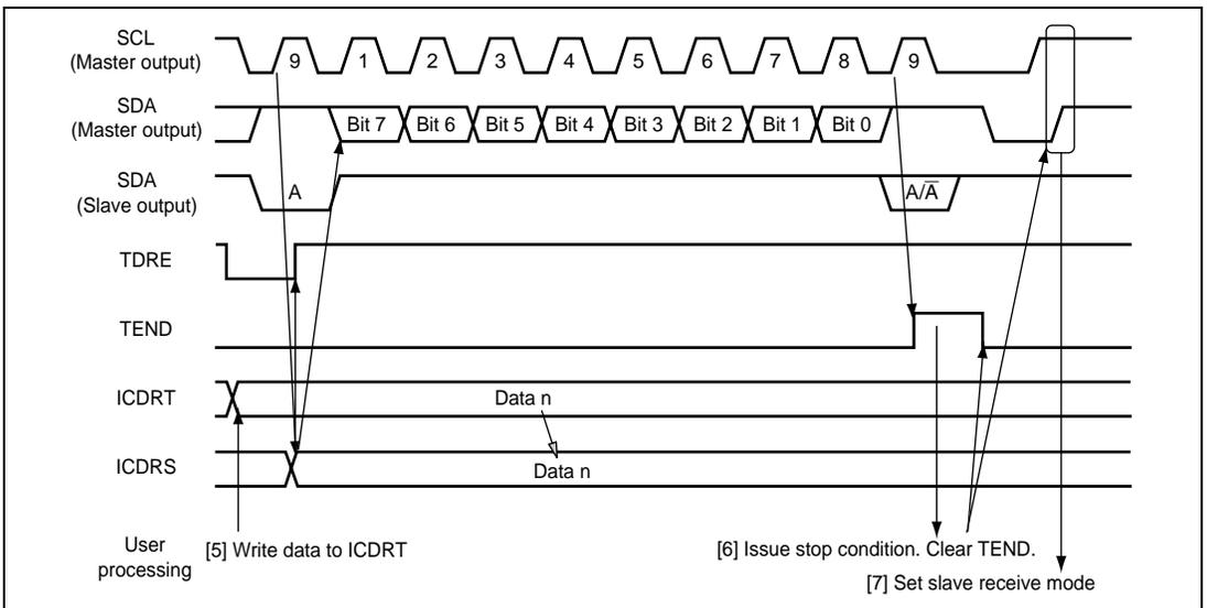
**Figure 21.6 Master Transmit Mode Operation Timing (2)**
