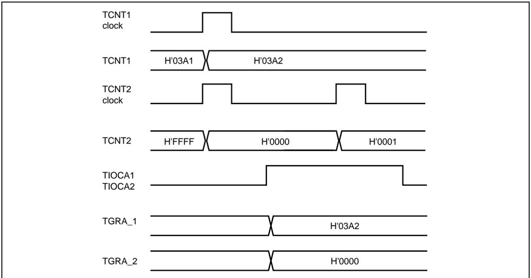
**Figure 12.16 Example of Operation with Cascaded Connection**
