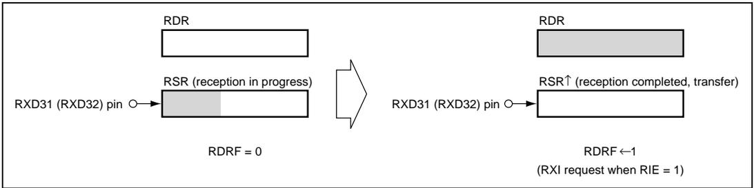
**Figure 15.17 (a) RDRF Setting and RXI Interrupt**
