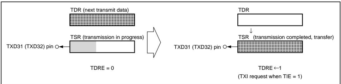
**Figure 15.17 (b) TDRE Setting and TXI Interrupt**
