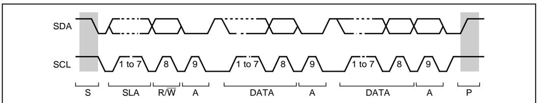
Figure 21.4 I<sup>2</sup>C Bus Timing
