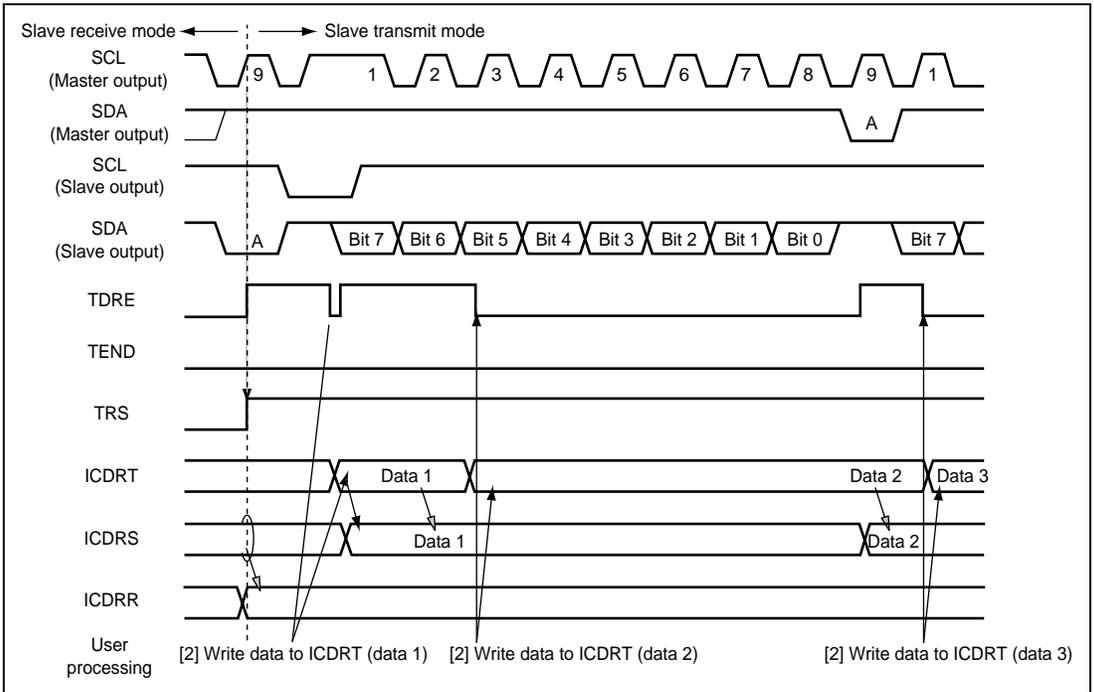
**Figure 21.9 Slave Transmit Mode Operation Timing (1)**
