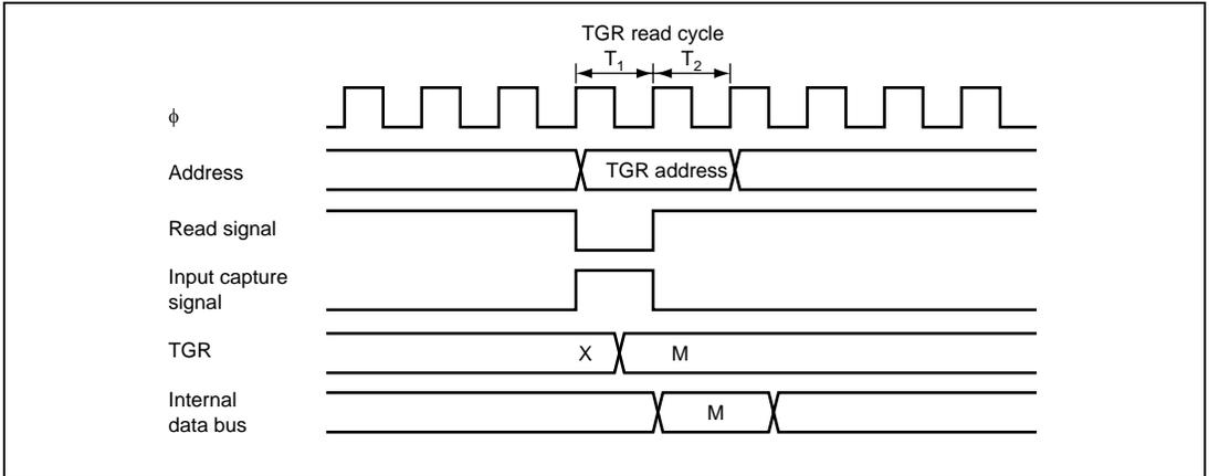
**Figure 12.34 Contention between TGR Read and Input Capture**
