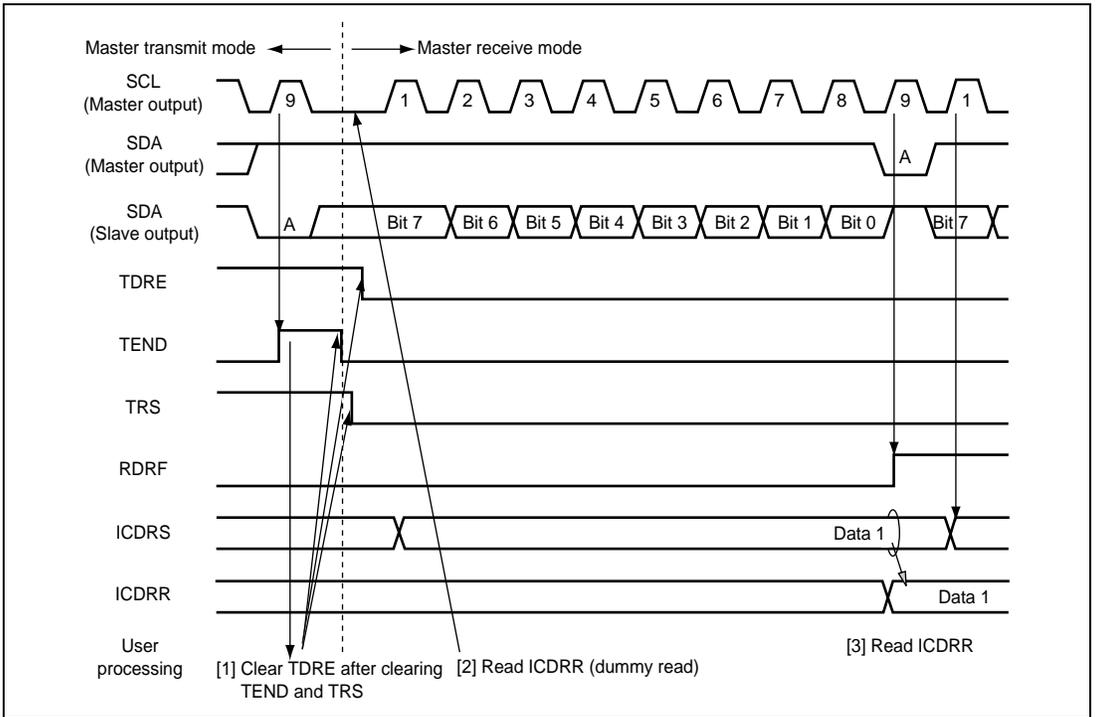
**Figure 21.7 Master Receive Mode Operation Timing (1)**
