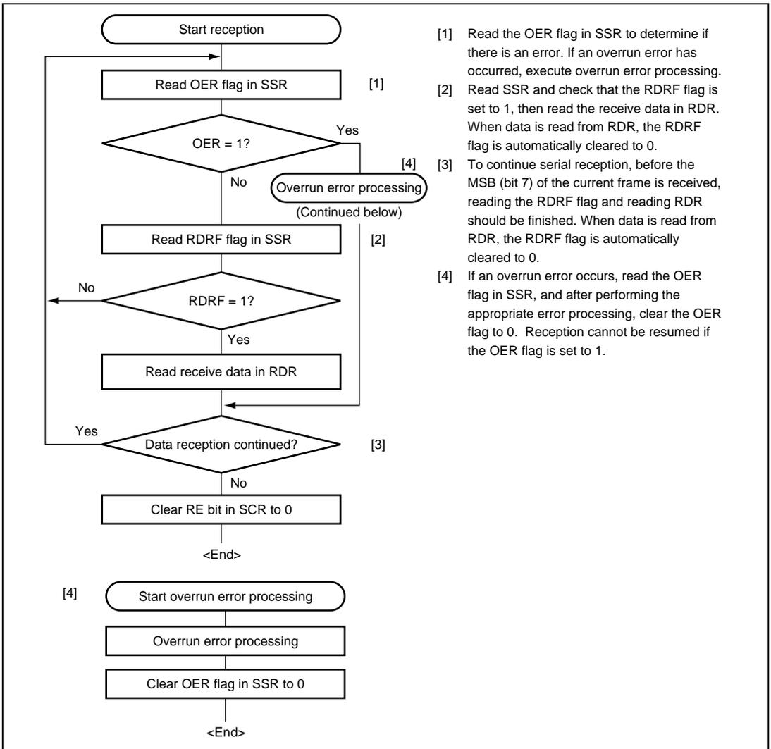
**Figure 15.13 Sample Serial Reception Flowchart (Clocked Synchronous Mode)**
