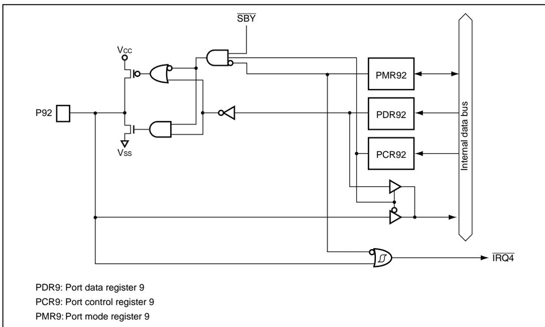
**Figure B.8 (b) Port 9 Block Diagram (P92)**
