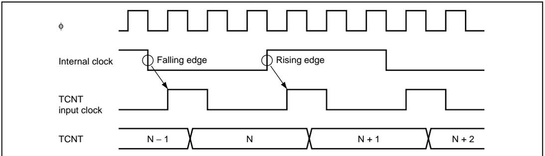
**Figure 12.21 Count Timing in Internal Clock Operation**
