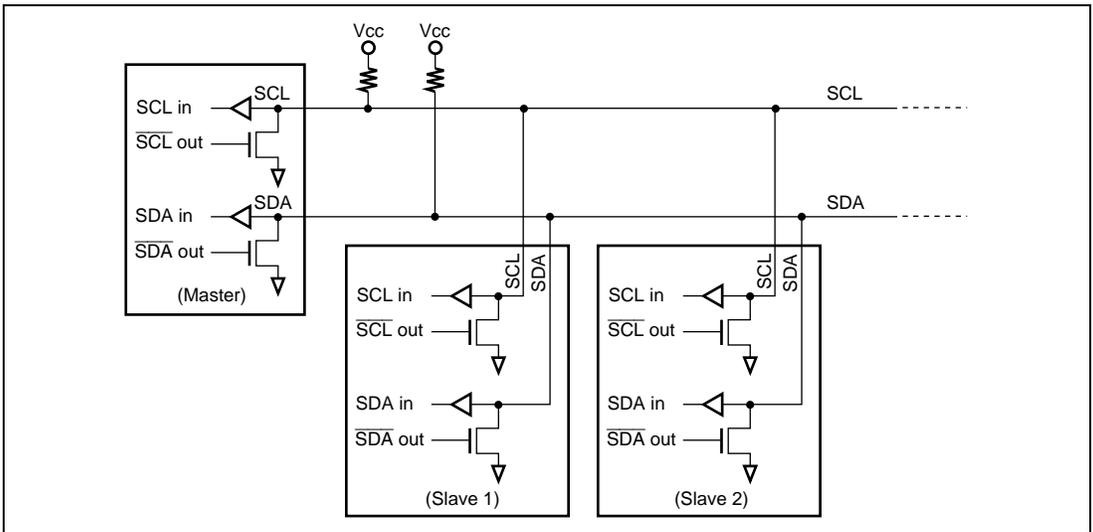
**Figure 21.2 External Circuit Connections of I/O Pins**
