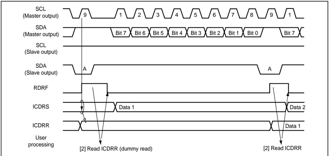
**Figure 21.11 Slave Receive Mode Operation Timing (1)**
