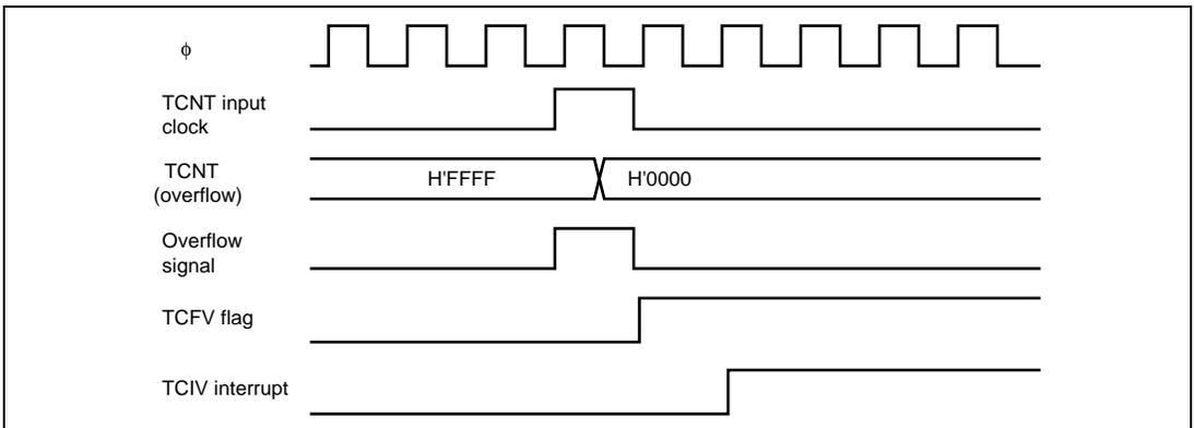
**Figure 12.29 TCIV Interrupt Setting Timing**
