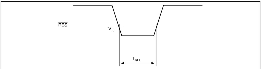
**Figure 25.3  $\overline{\text{RES}}$  Low Width Timing**
