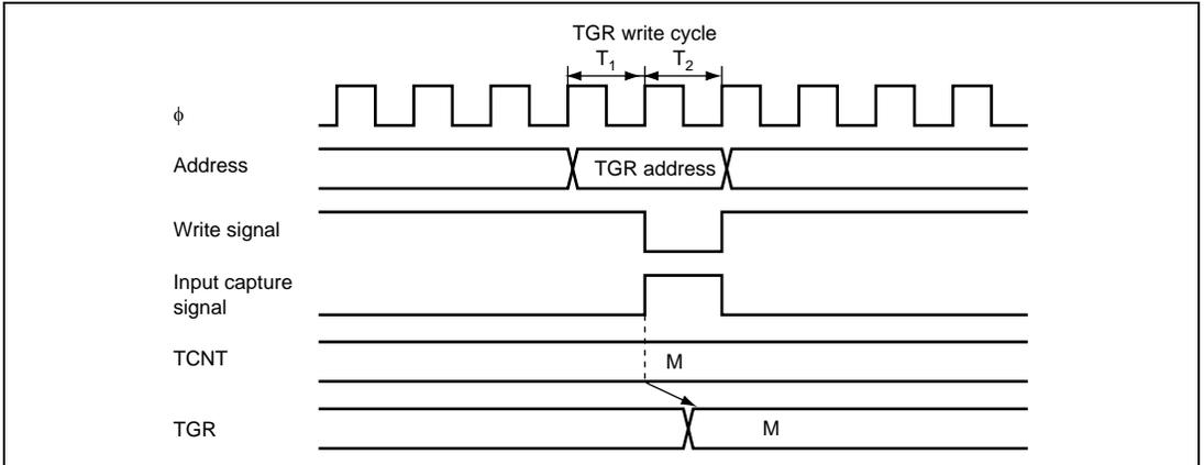
**Figure 12.35 Contention between TGR Write and Input Capture**
