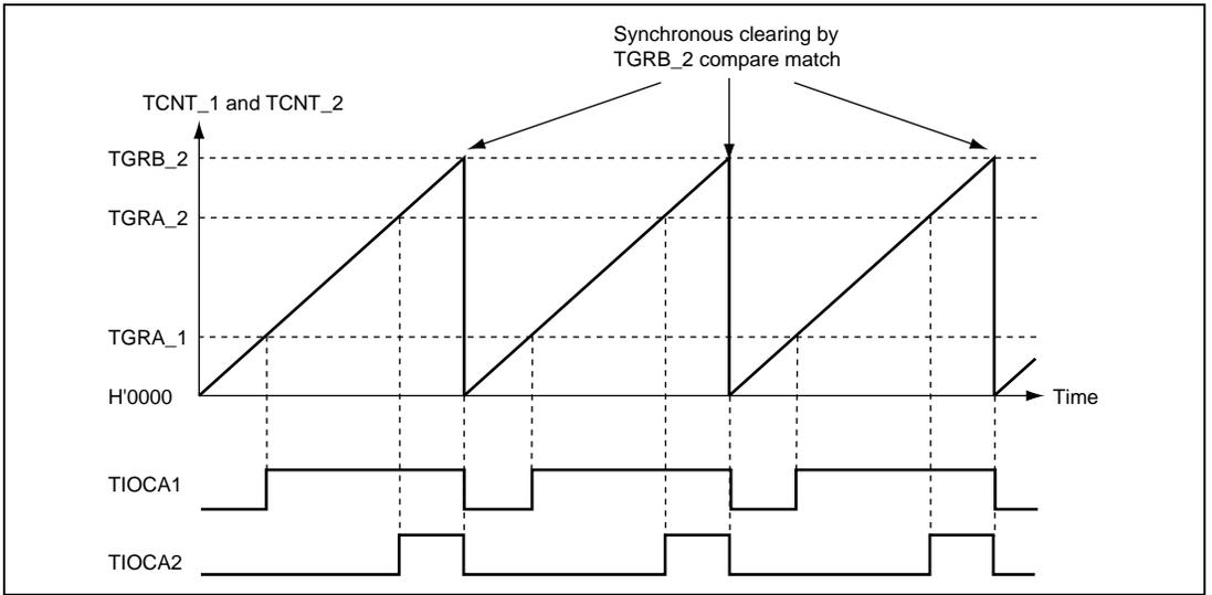
**Figure 12.19 Example of PWM Mode Operation (2)**
