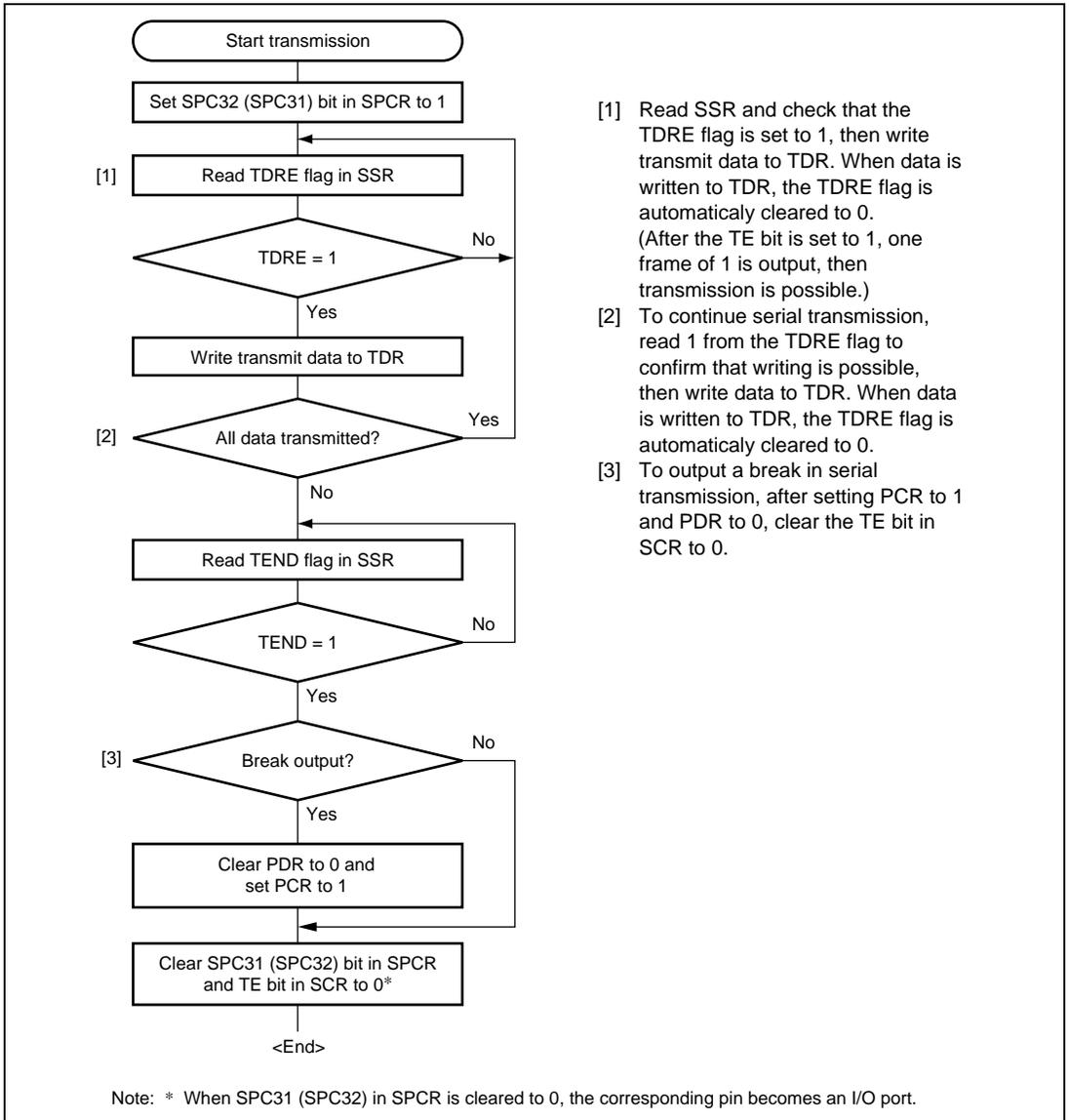
**Figure 15.6 Sample Serial Transmission Flowchart (Asynchronous Mode)**
