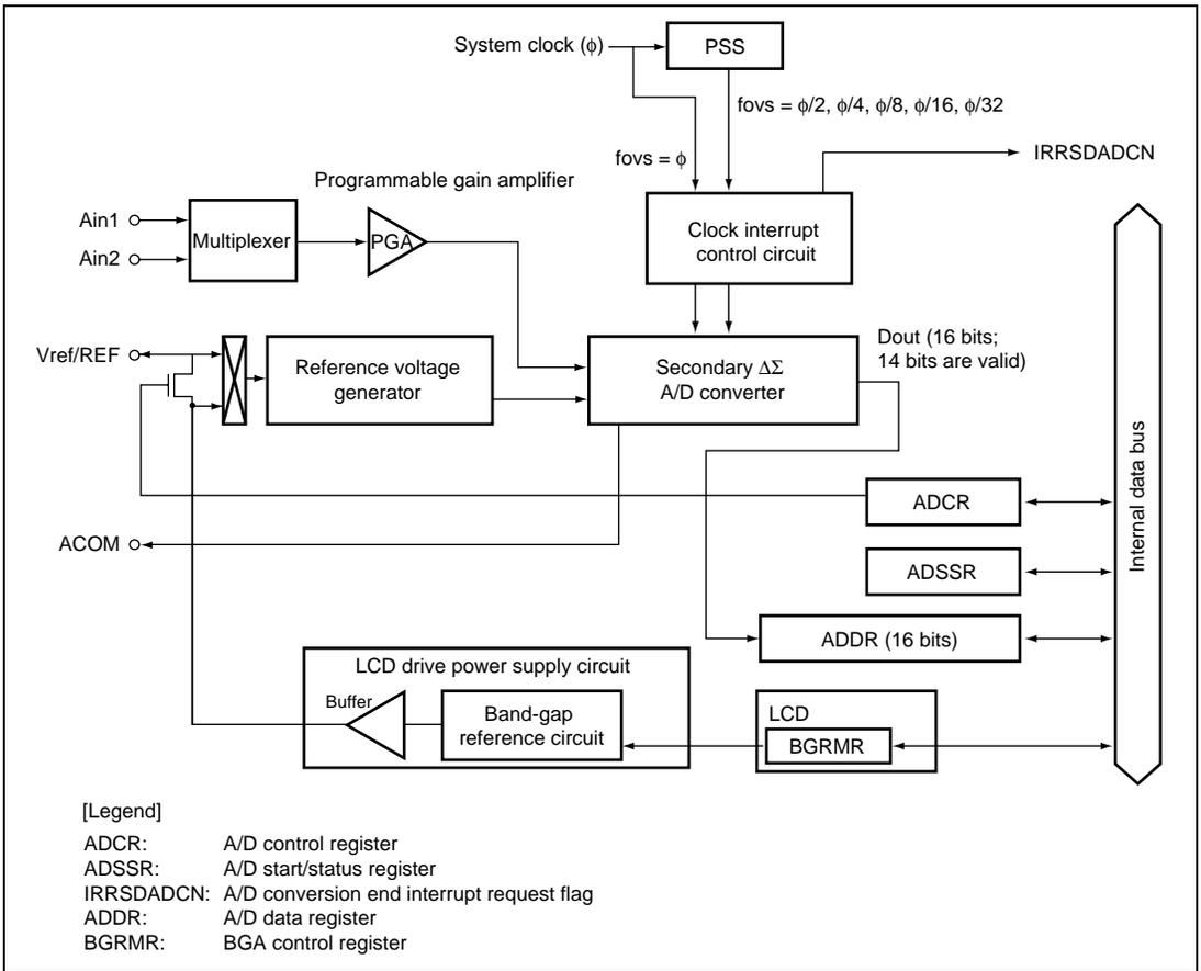
**Figure 19.1 Block Diagram of  $\Delta\Sigma$  A/D Converter**
