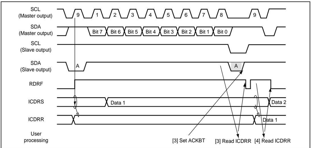
**Figure 21.12 Slave Receive Mode Operation Timing (2)**
