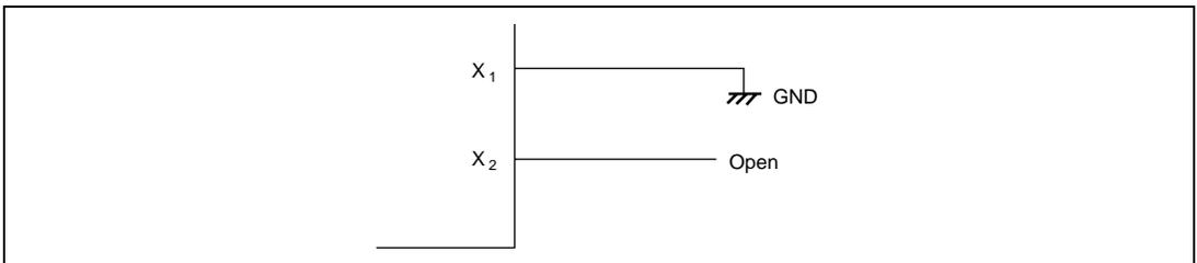
**Figure 5.7 Pin Connection when not Using Subclock**
