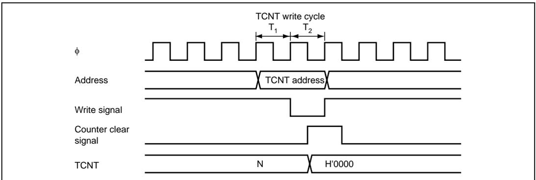
**Figure 12.31 Contention between TCNT Write and Clear Operation**
