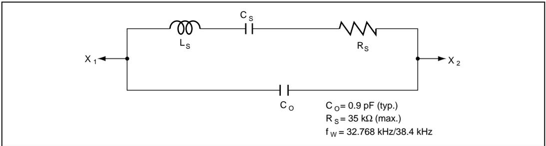
**Figure 5.6 Equivalent Circuit of 32.768-kHz/38.4-kHz Crystal Resonator**
