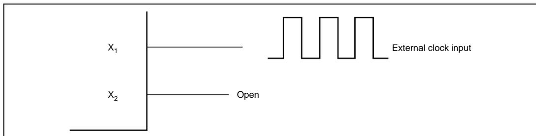
**Figure 5.8 Pin Connection when Inputting External Clock**
