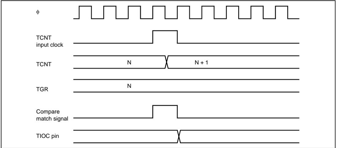
**Figure 12.23 Output Compare Output Timing**
