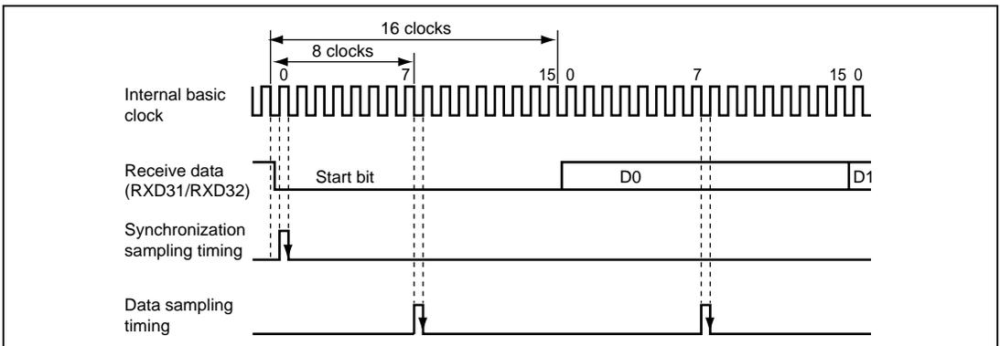
**Figure 15.18 Receive Data Sampling Timing in Asynchronous Mode**
