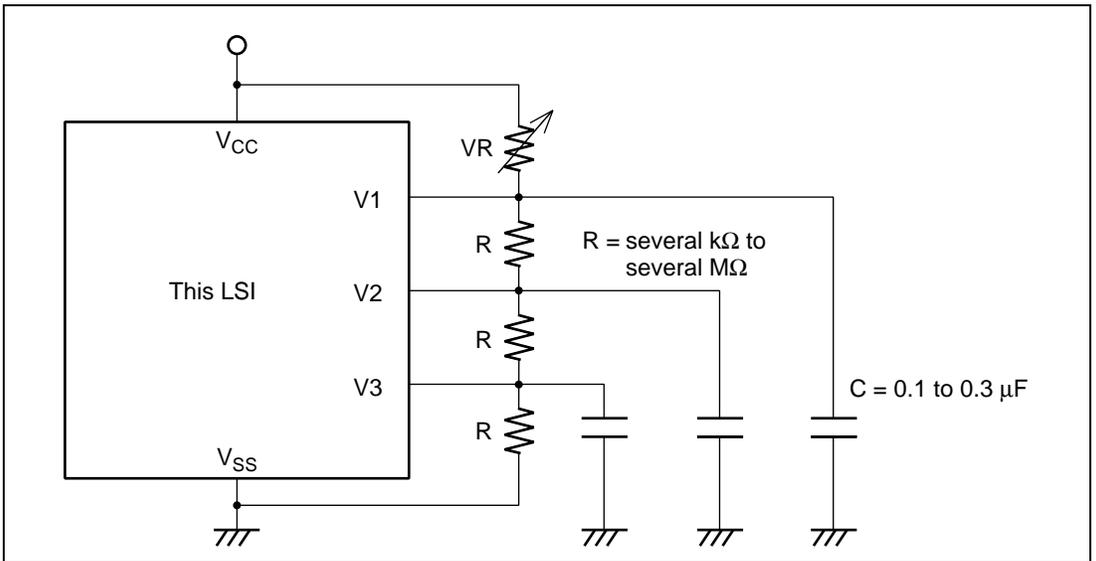
**Figure 20.10 Connection of External Split Resistor**
