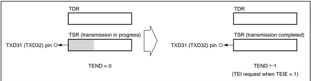
**Figure 15.17 (c) TEND Setting and TEI Interrupt**
