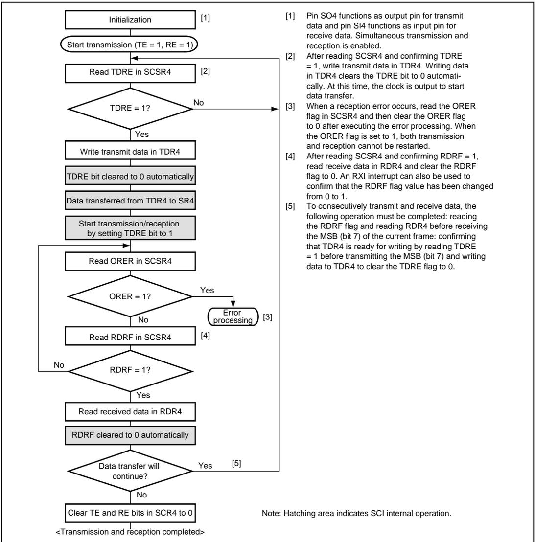
**Figure 16.8 Flowchart Example of Simultaneous Transmission and Reception**
