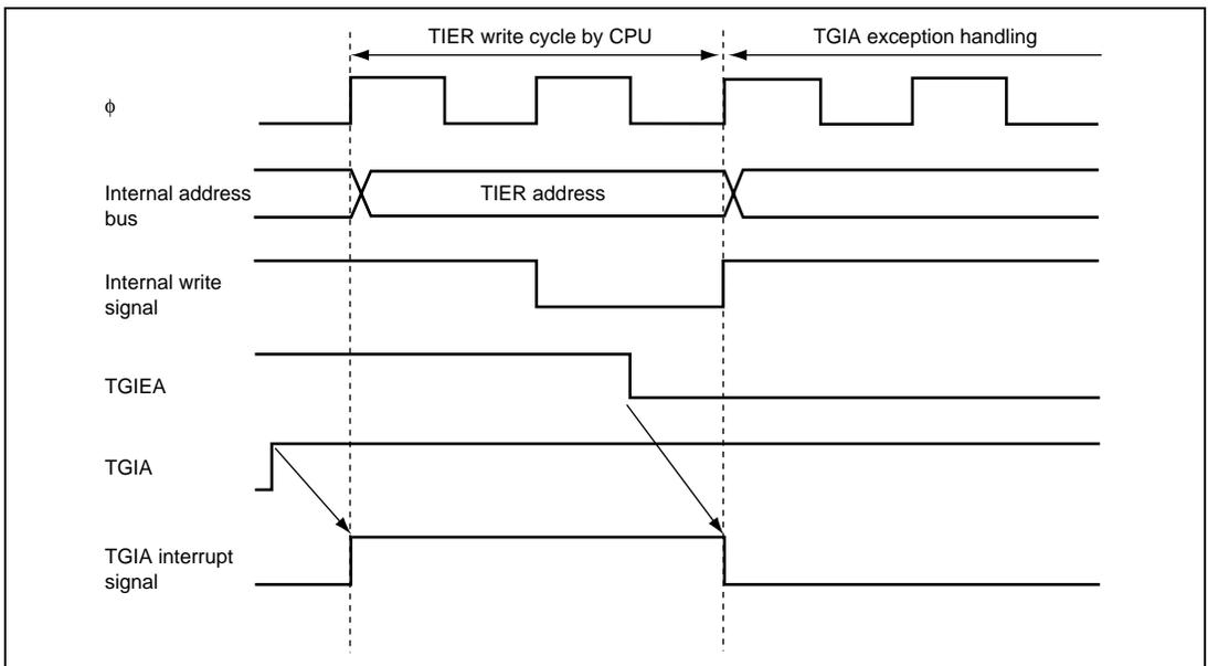
**Figure 4.4 Contention between Interrupt Generation and Disabling**
