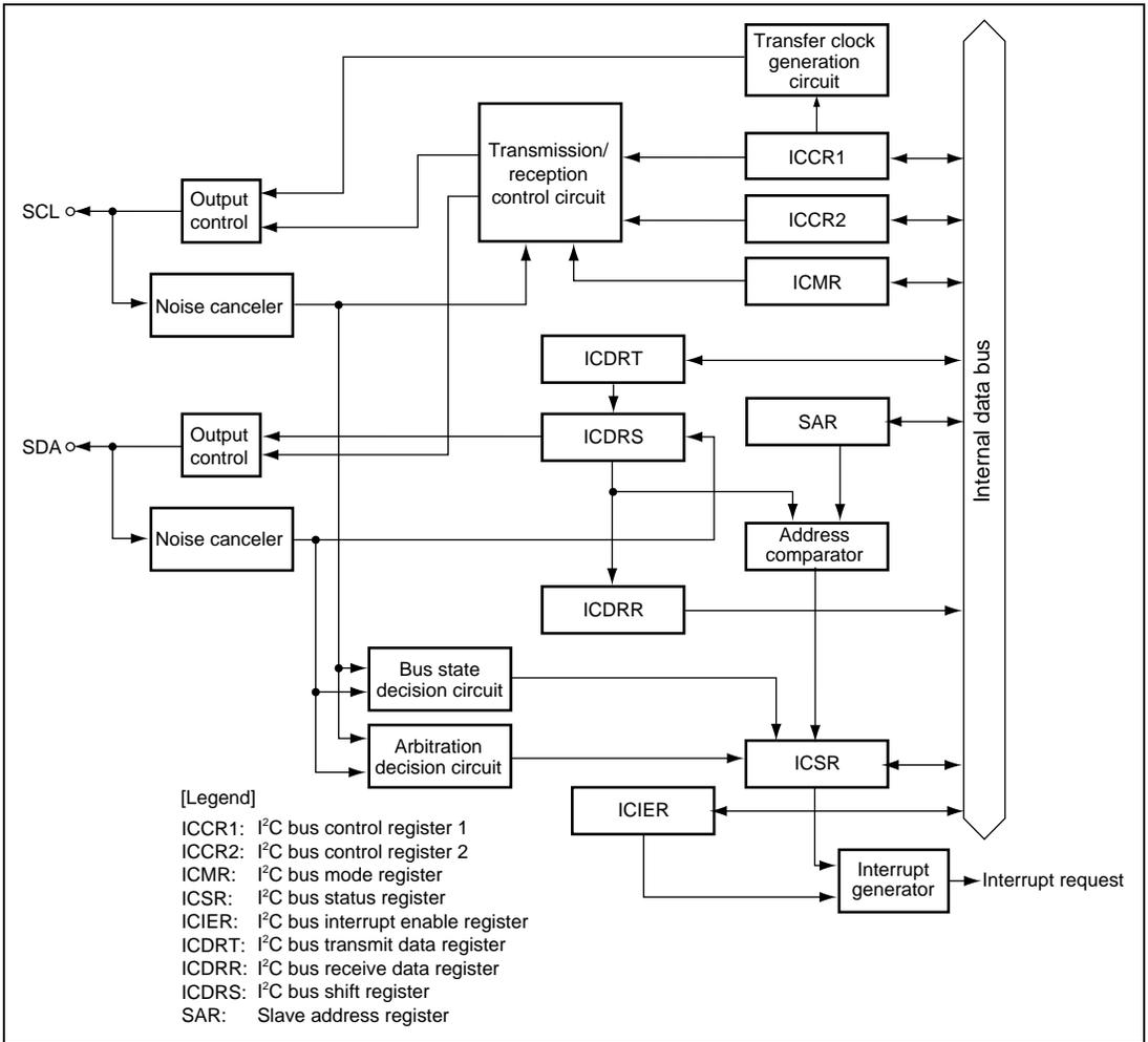
Figure 21.1 Block Diagram of I<sup>2</sup>C Bus Interface 2
