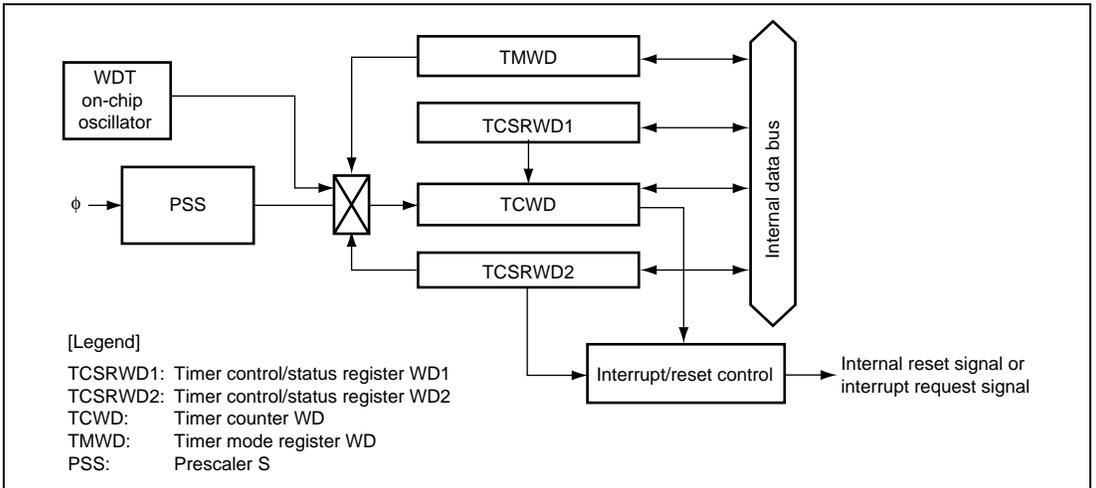
**Figure 14.1 Block Diagram of Watchdog Timer**
