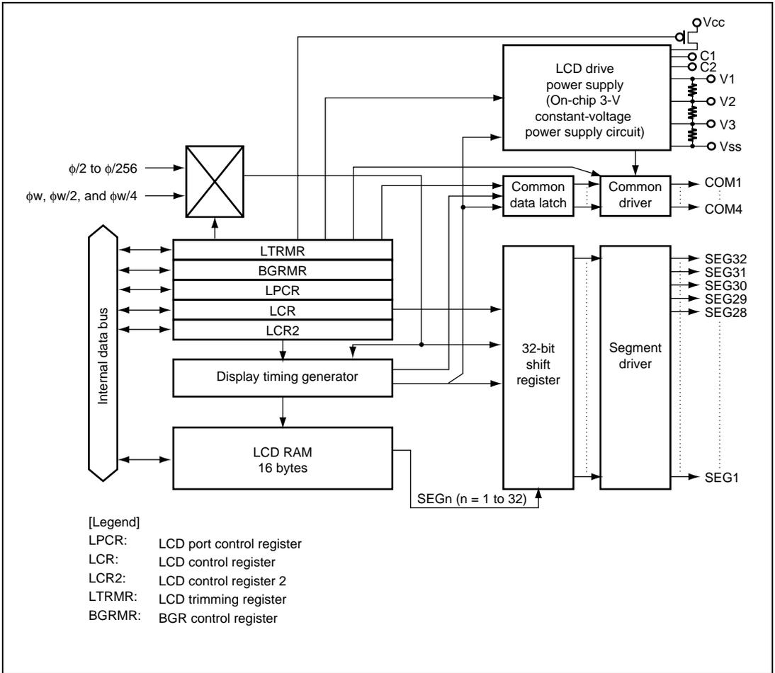
Figure 20.1 Block Diagram of LCD Controller/Driver
