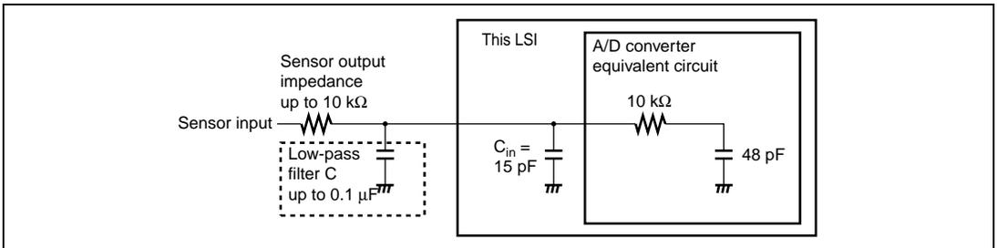
Figure 18.8 Example of Analog Input Circuit
