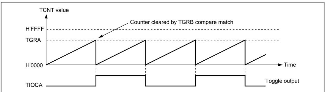
**Figure 12.10 Example of Toggle Output Operation**
