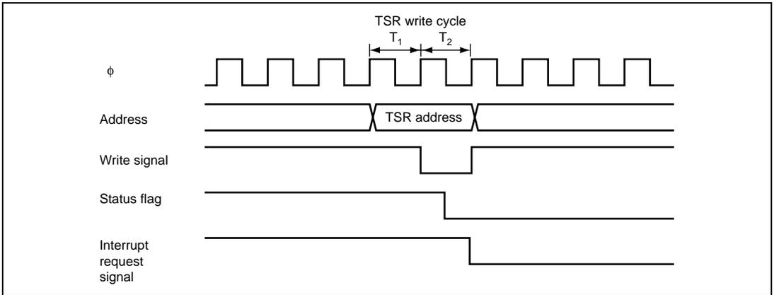
Figure 12.30 Timing for Status Flag Clearing by CPU
