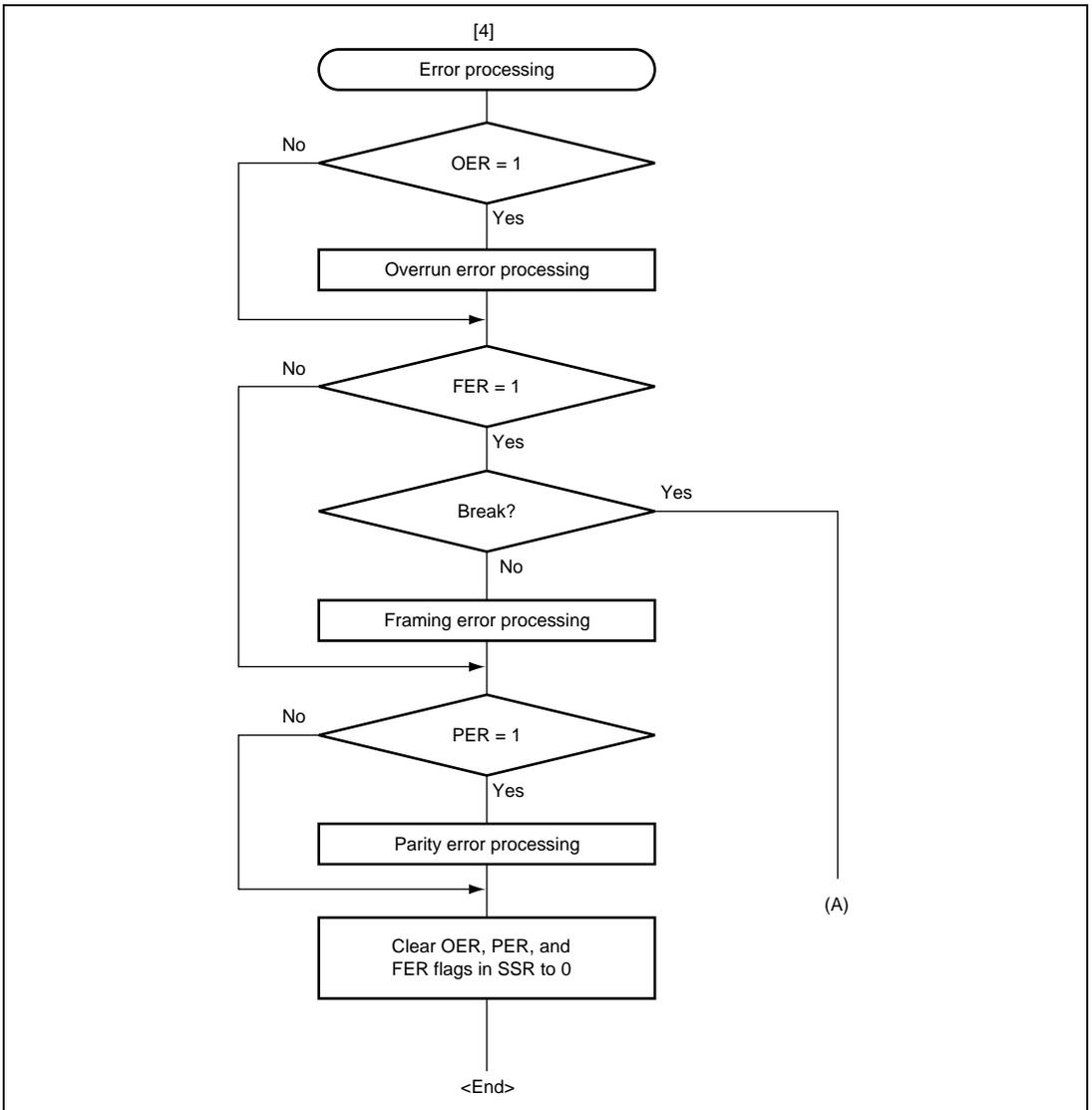
**Figure 15.8 Sample Serial Data Reception Flowchart (Asynchronous Mode) (2)**
