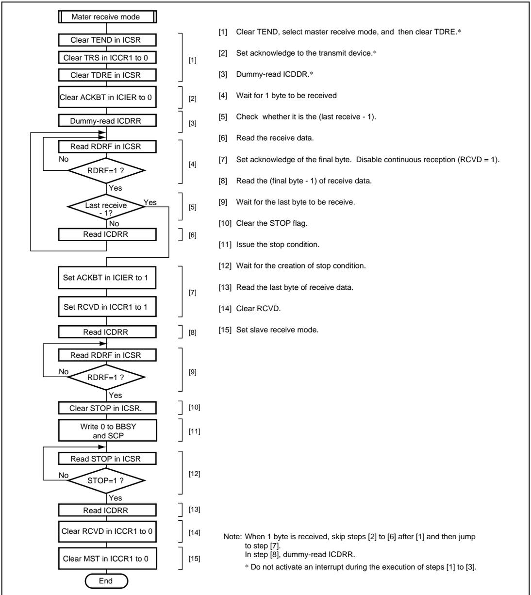
**Figure 21.18 Sample Flowchart for Master Receive Mode**
