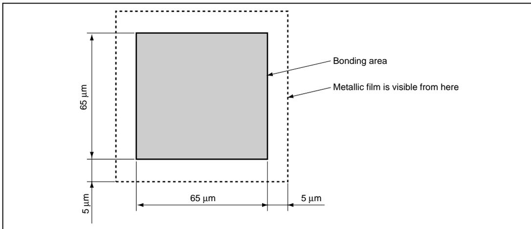
**Figure F.1 Bonding Pad Form**
