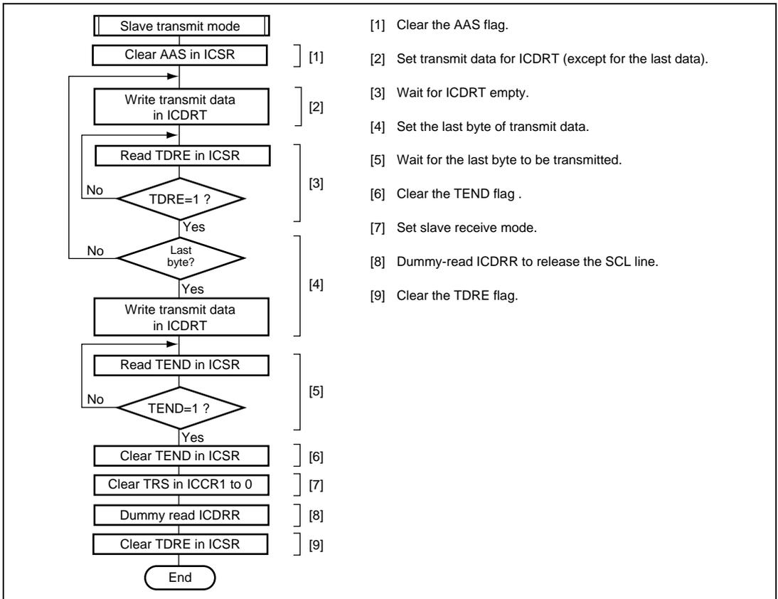
**Figure 21.19 Sample Flowchart for Slave Transmit Mode**
