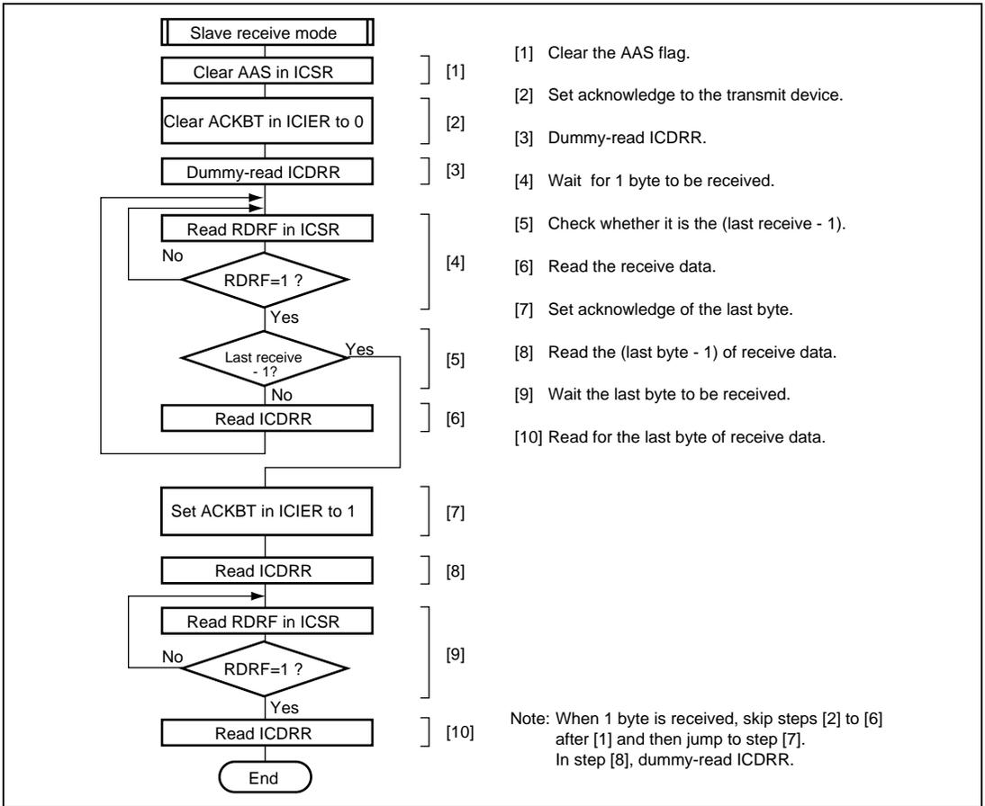
**Figure 21.20 Sample Flowchart for Slave Receive Mode**
