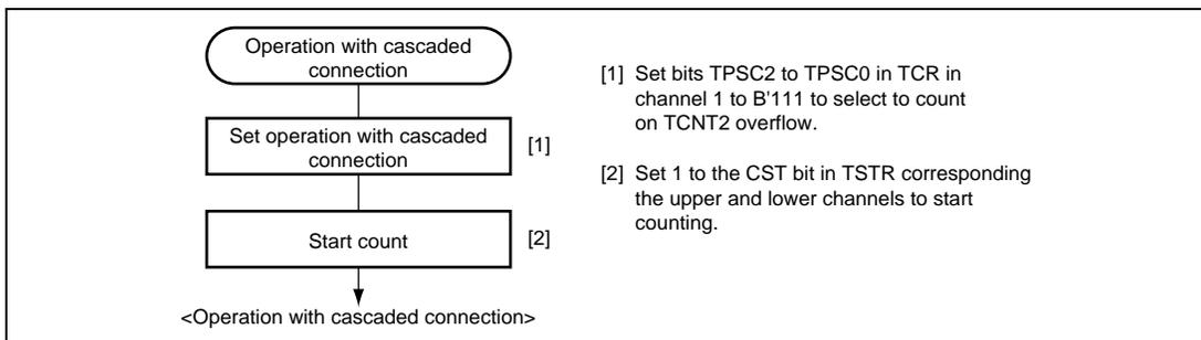
**Figure 12.15 Setting Procedure for Operation with Cascaded Operation**
