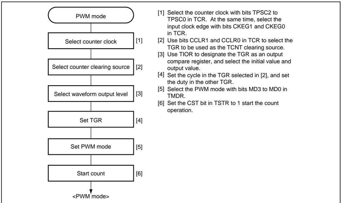
**Figure 12.17 Example of PWM Mode Setting Procedure**
