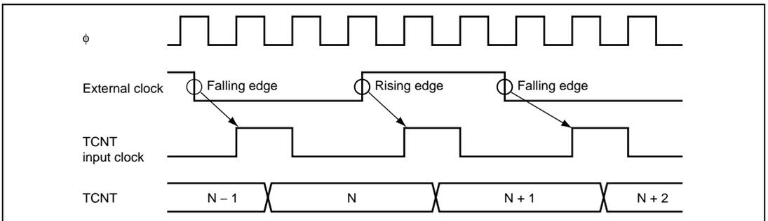
**Figure 12.22 Count Timing in External Clock Operation**
