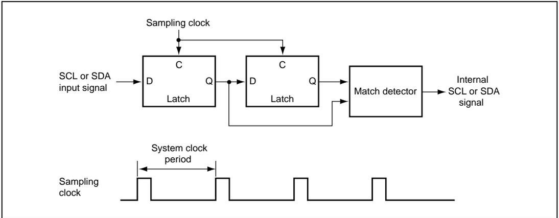
**Figure 21.16 Block Diagram of Noise Canceler**
