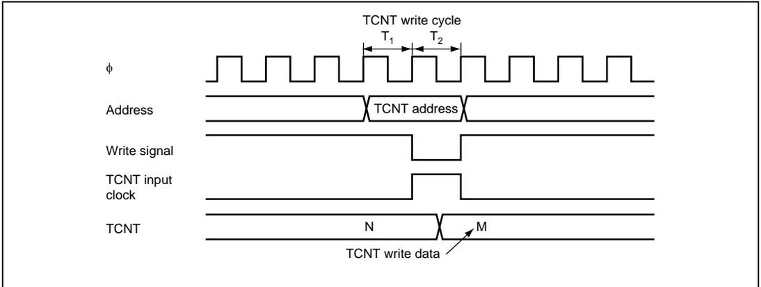
**Figure 12.32 Contention between TCNT Write and Increment Operation**
