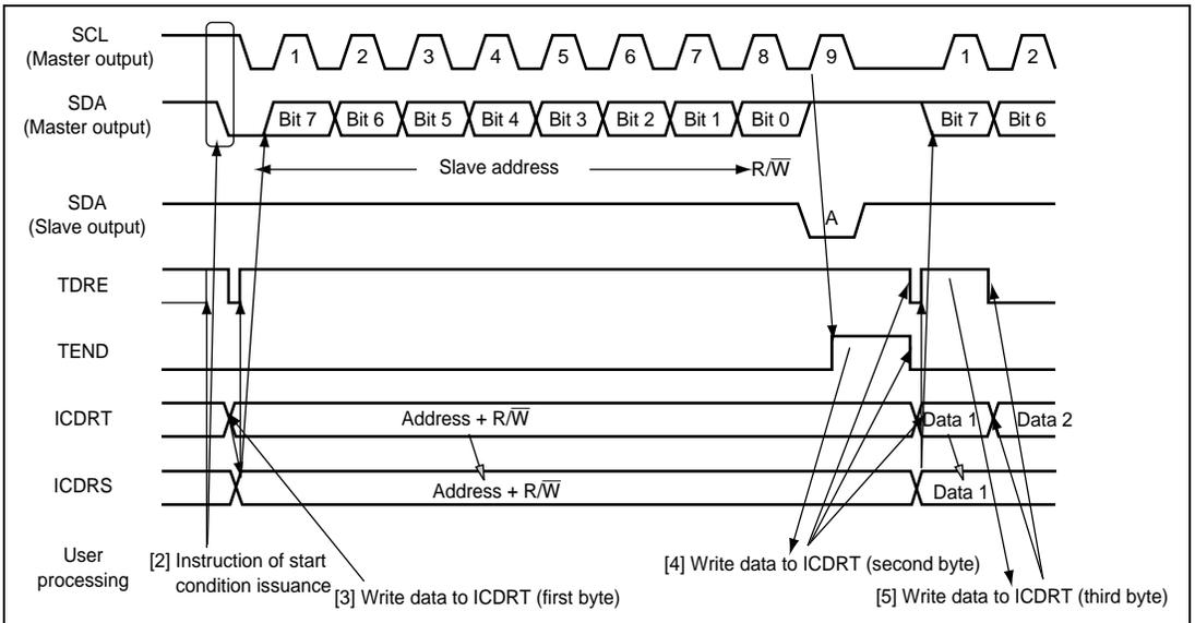
**Figure 21.5 Master Transmit Mode Operation Timing (1)**
