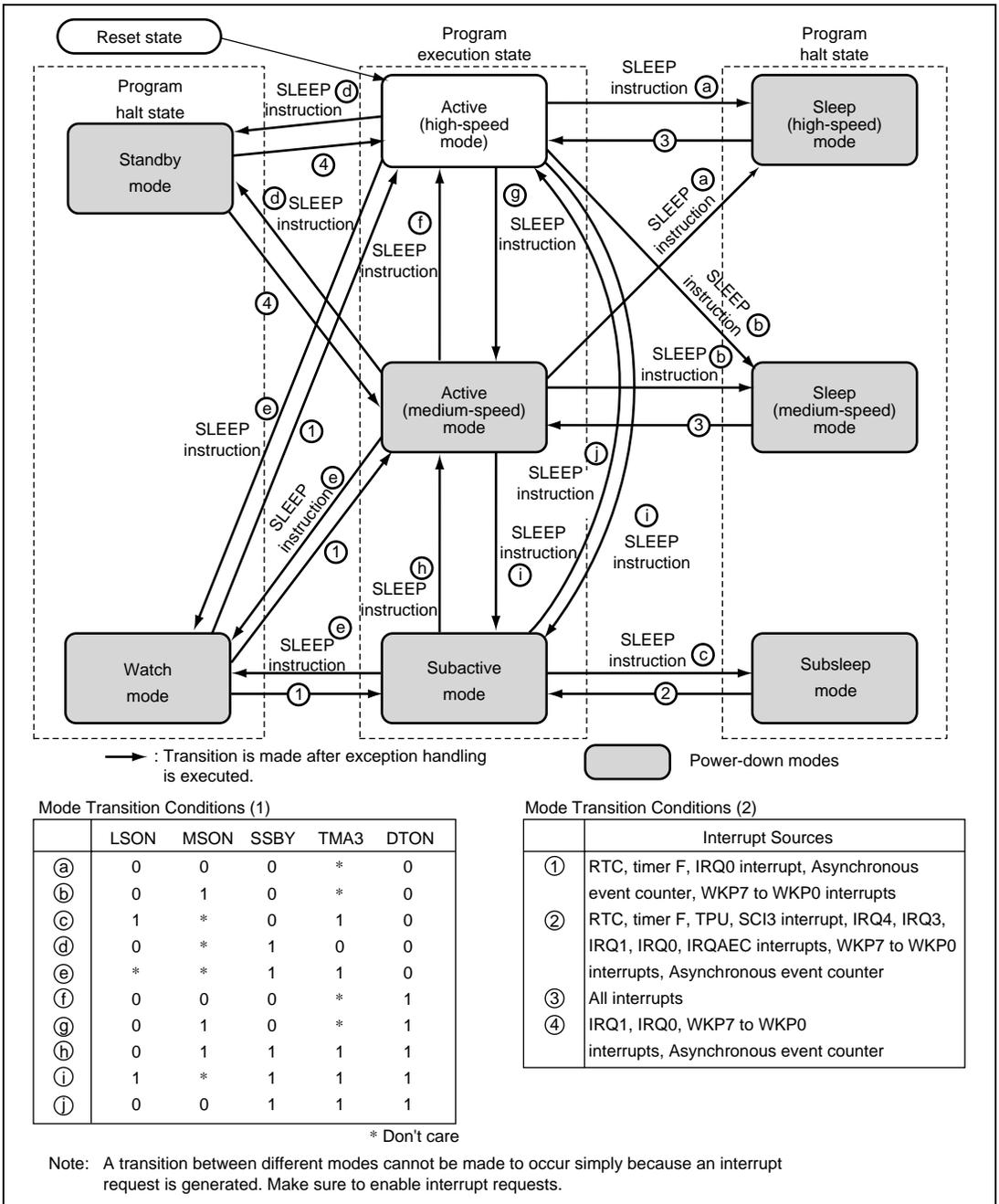
Figure 6.1 Mode Transition Diagram
