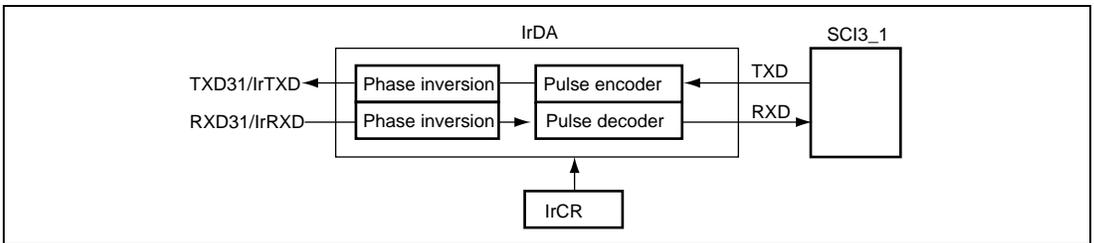
**Figure 15.15 IrDA Block Diagram**
