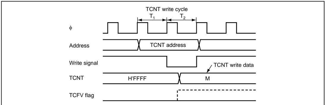
**Figure 12.37 Contention between TCNT Write and Overflow**
