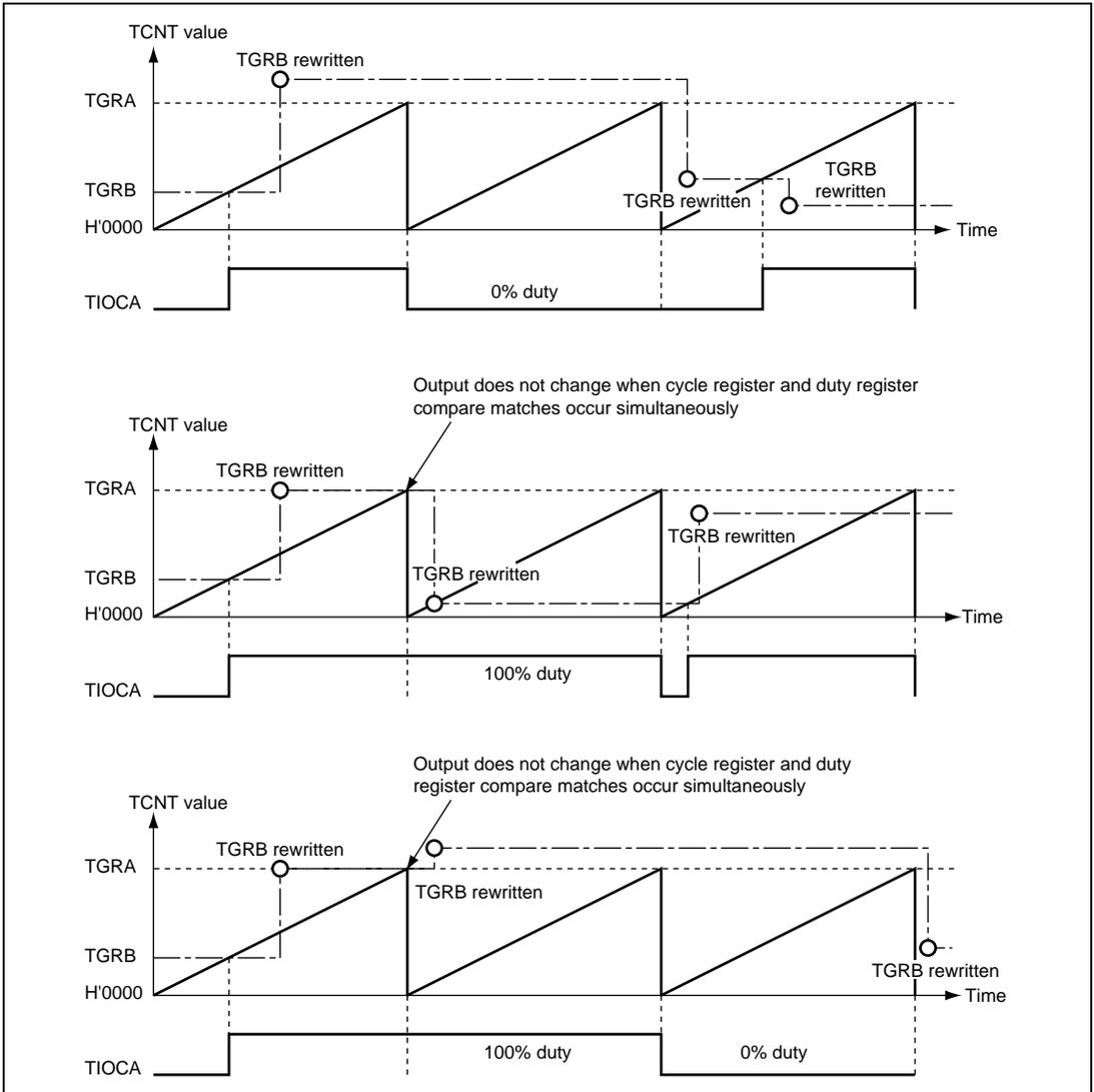
**Figure 12.20 Example of PWM Mode Operation (3)**
