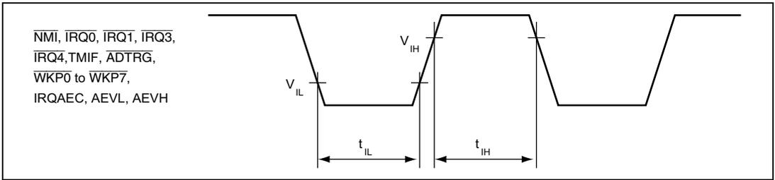
Figure 25.4 Input Timing
