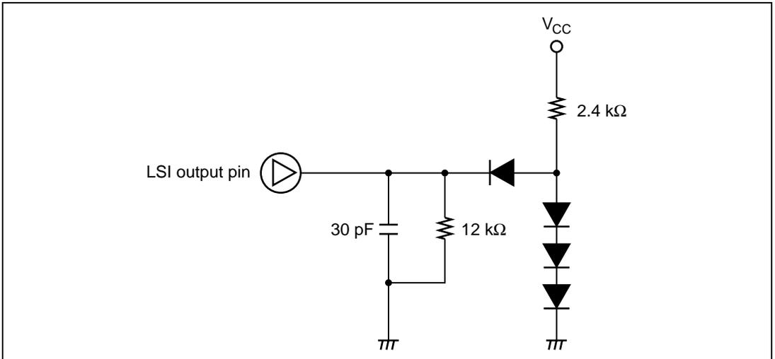
Figure 25.9 Output Load Condition
