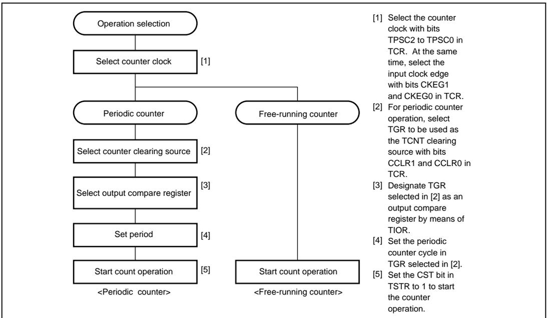
**Figure 12.5 Example of Counter Operation Setting Procedure**
