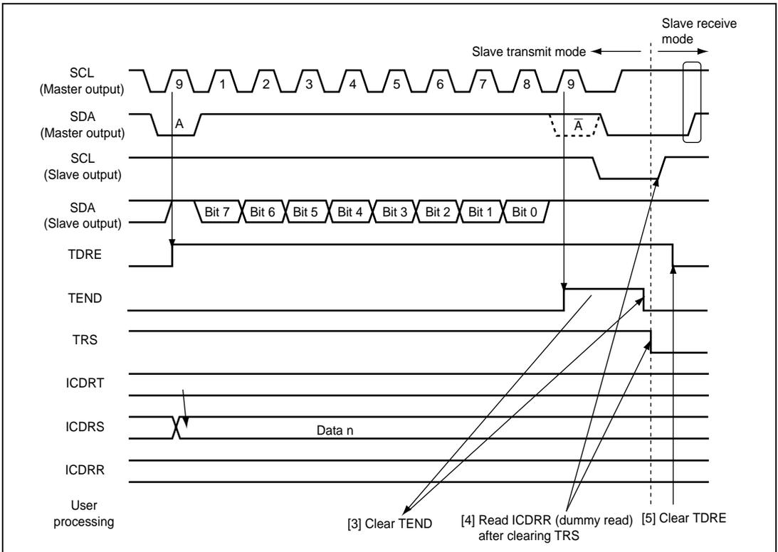
**Figure 21.10 Slave Transmit Mode Operation Timing (2)**
