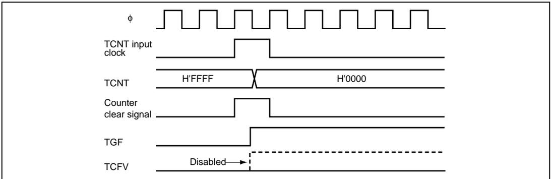
**Figure 12.36 Contention between Overflow and Counter Clearing**
