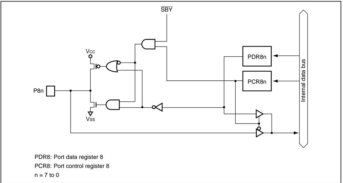
**Figure B.7 Port 8 Block Diagram**
