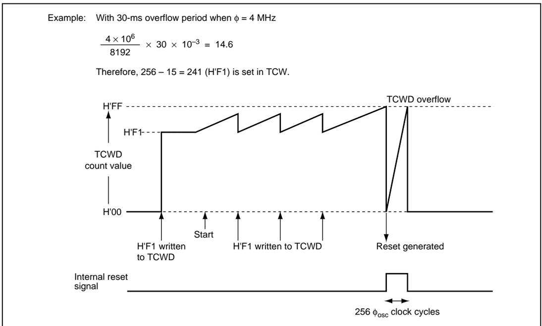
**Figure 14.2 Example of Watchdog Timer Operation**
