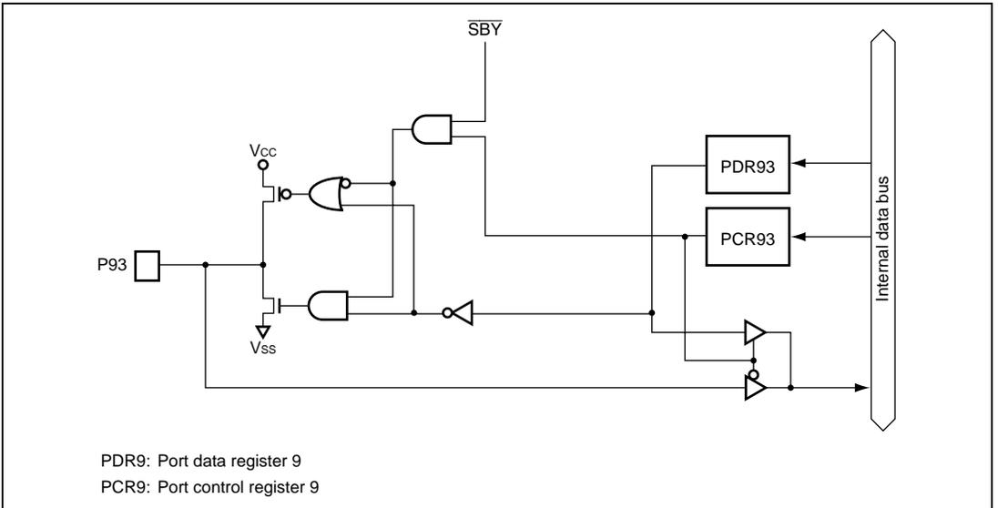
**Figure B.8 (a) Port 9 Block Diagram (P93)**
