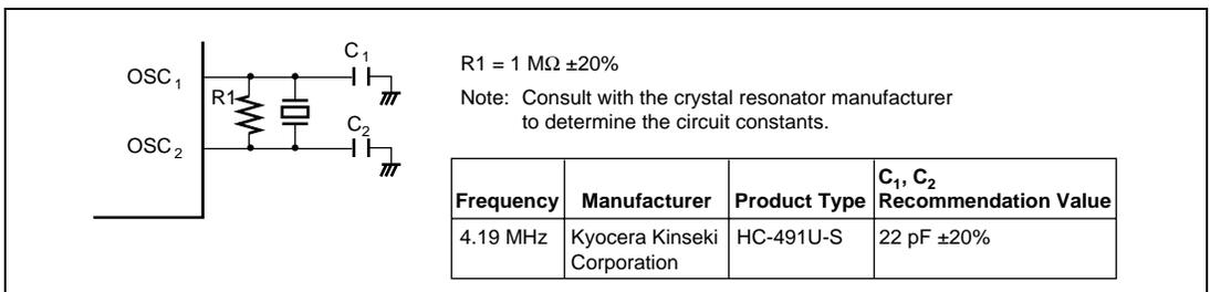
**Figure 5.2 Typical Connection to Crystal Resonator**
