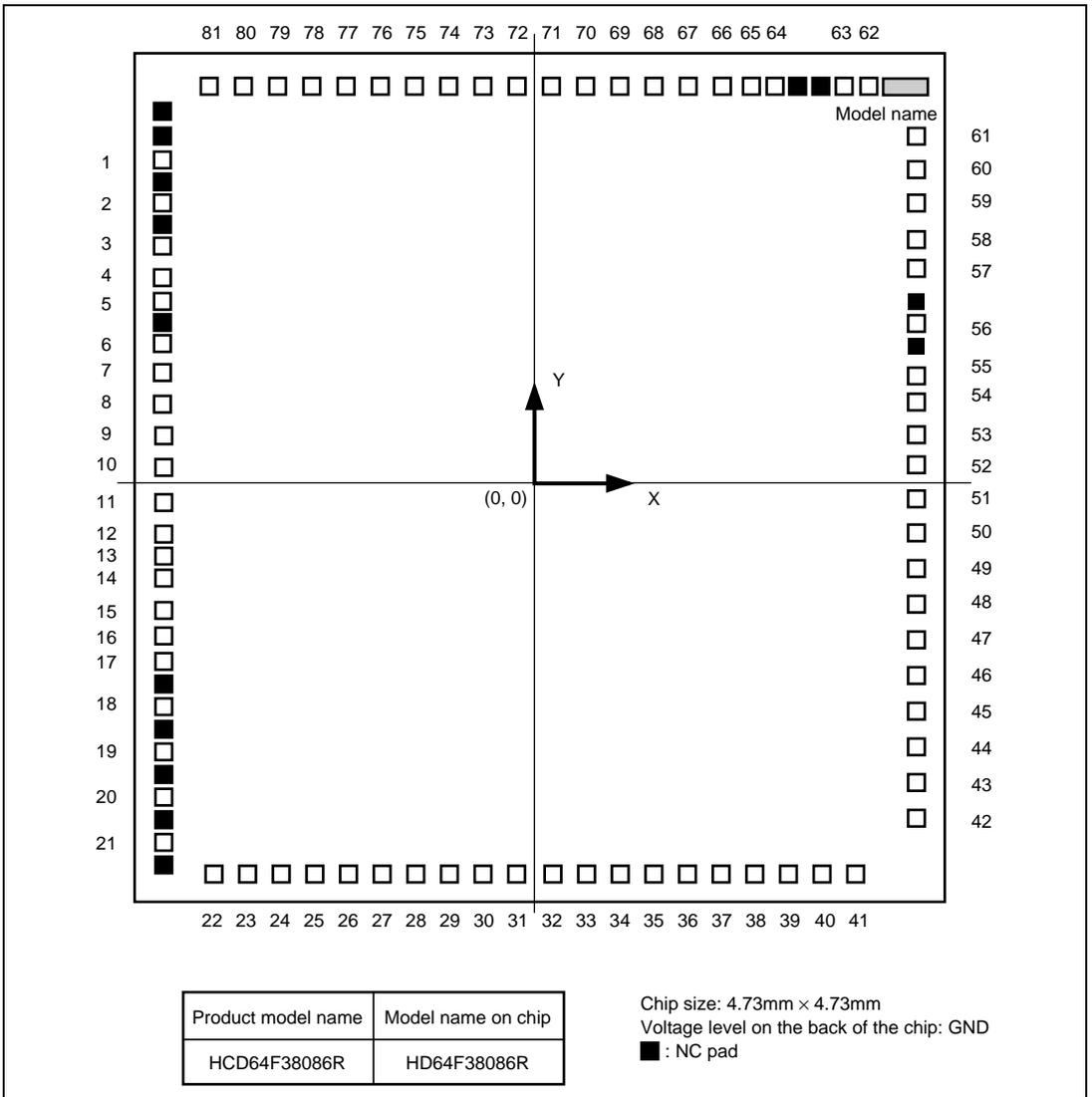
Figure 1.4 Pad Assignment of HCD64F38086R (Top View)
