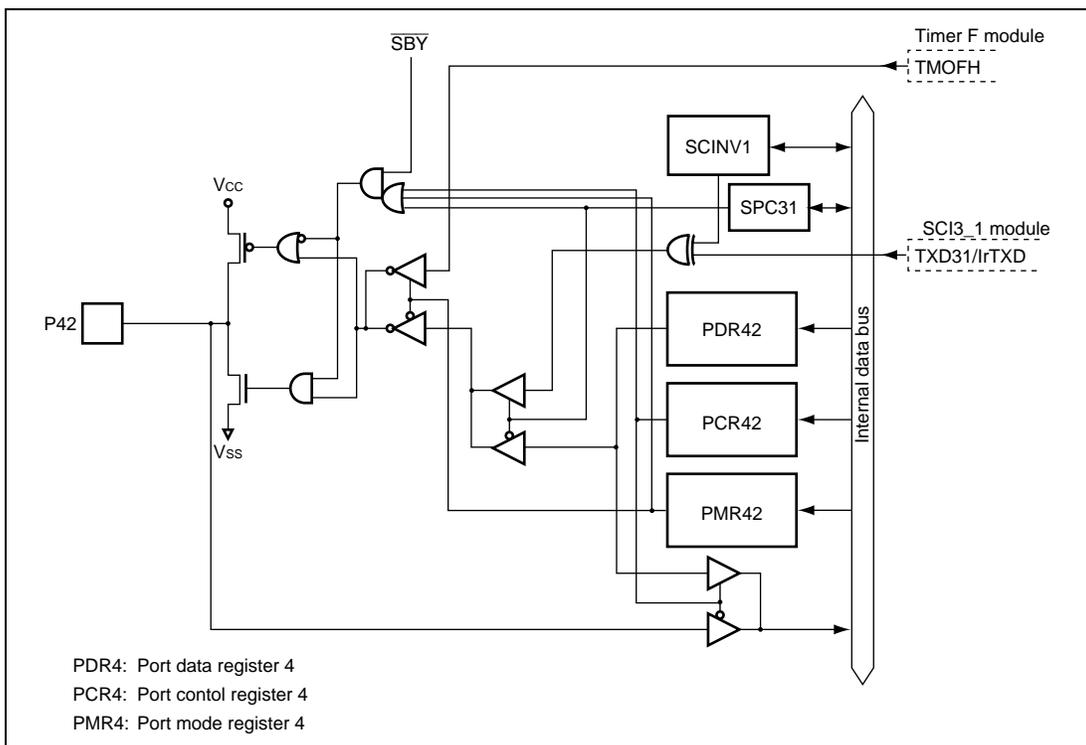
**Figure B.3 (a) Port 4 Block Diagram (P42)**
