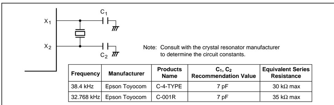
**Figure 5.5 Typical Connection to 32.768-kHz/38.4-kHz Crystal Resonator**
