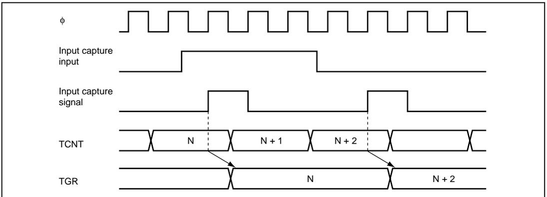
**Figure 12.24 Input Capture Input Signal Timing**
