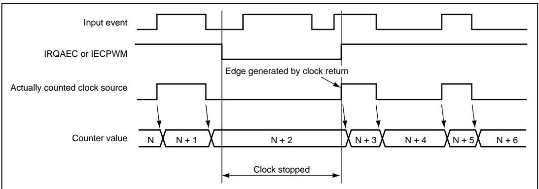
**Figure 13.5 Example of Clock Control Operation**
