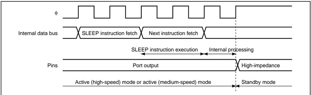
**Figure 6.2 Standby Mode Transition and Pin States**
