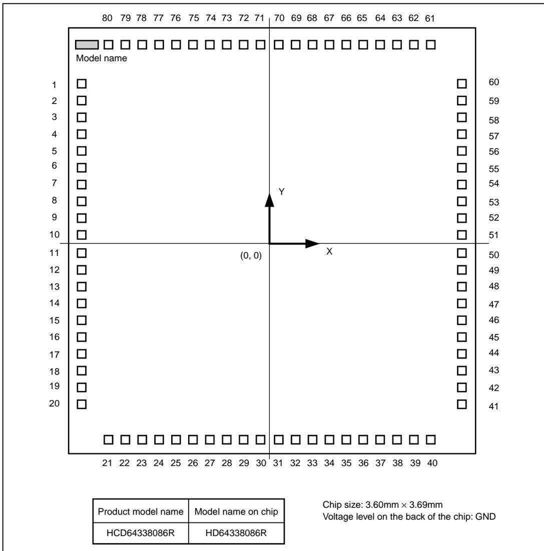
Figure 1.5 Pad Assignment of HCD64338086R (Top View)
