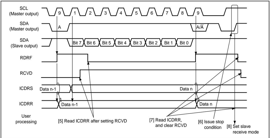
**Figure 21.8 Master Receive Mode Operation Timing (2)**
