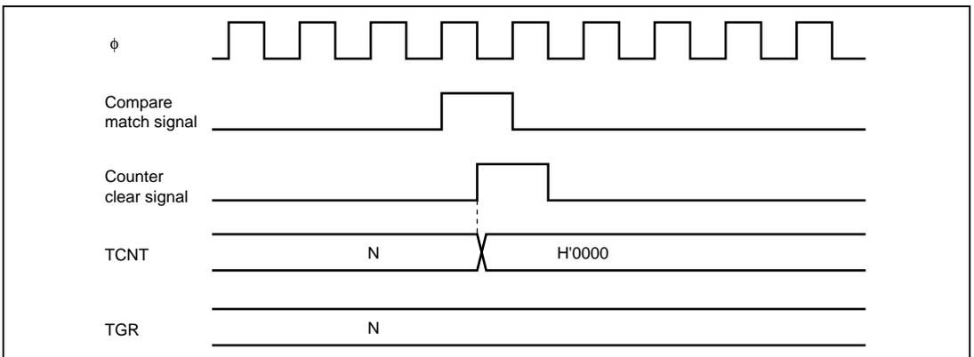
**Figure 12.25 Counter Clear Timing (Compare Match)**
