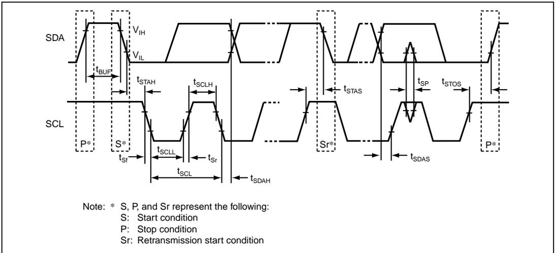
Figure 25.8 I<sup>2</sup>C Bus Interface Input/Output Timing
