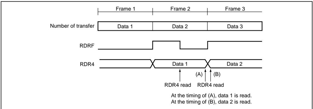
**Figure 16.9 Relationship between Reading RDR4 and RDRF**
