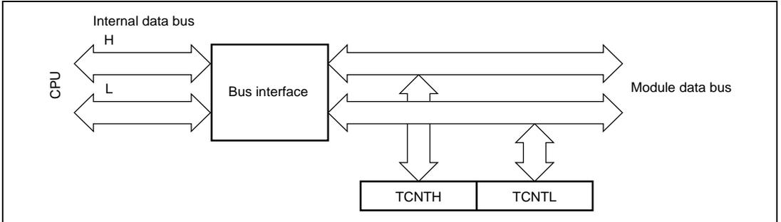
**Figure 12.2 16-Bit Register Access Operation [CPU ↔ TCNT (16 Bits)]**
