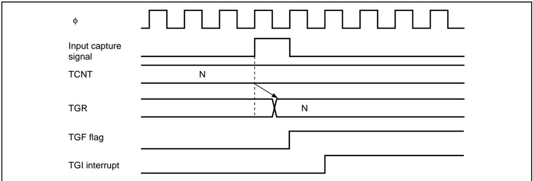
**Figure 12.28 TGI Interrupt Timing (Input Capture)**
