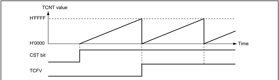
**Figure 12.6 Free-Running Counter Operation**
