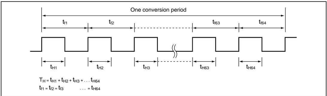
Figure 17.3 PWM Output Waveform
