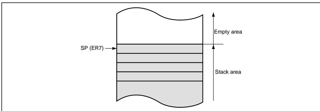
**Figure 2.4 Relationship between Stack Pointer and Stack Area**
