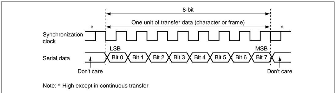
**Figure 15.9 Data Format in Clocked Synchronous Communication**
