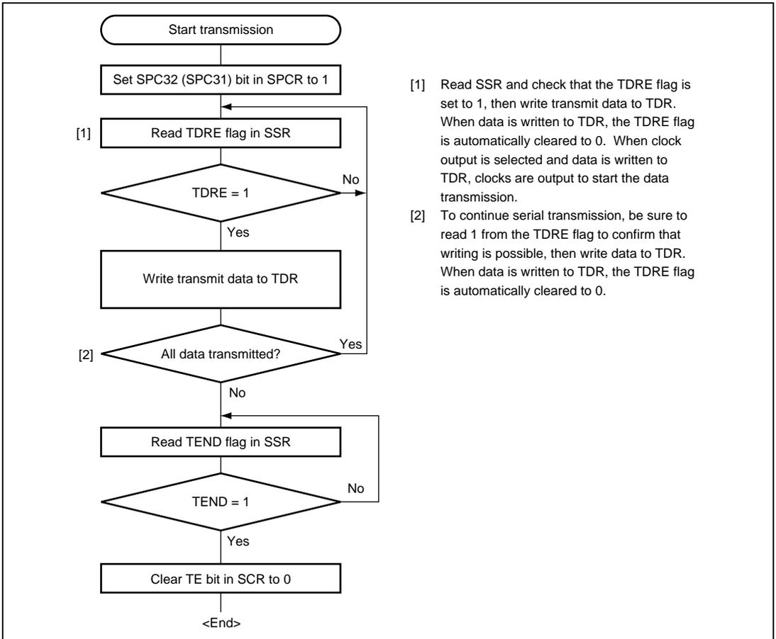
**Figure 15.11 Sample Serial Transmission Flowchart (Clocked Synchronous Mode)**
