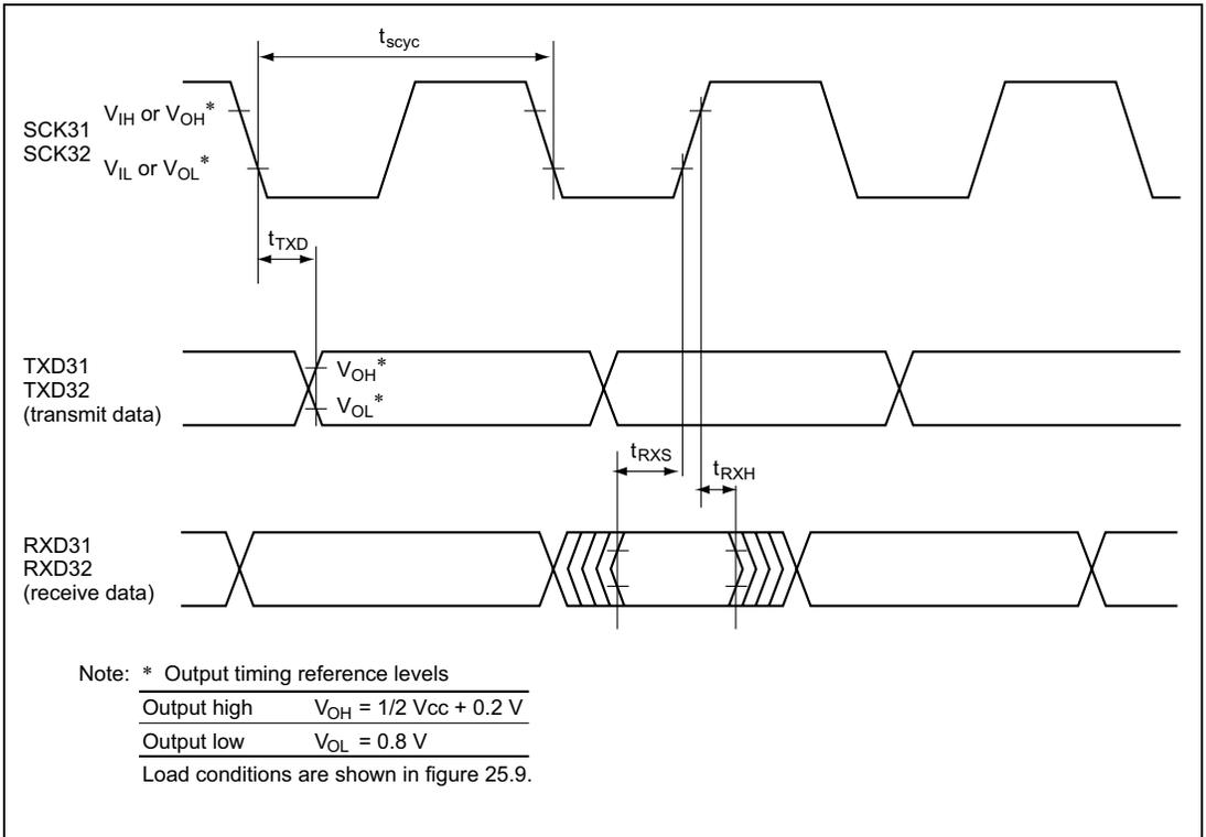
**Figure 25.6 SCI3 Input/Output Timing in Clocked Synchronous Mode**
