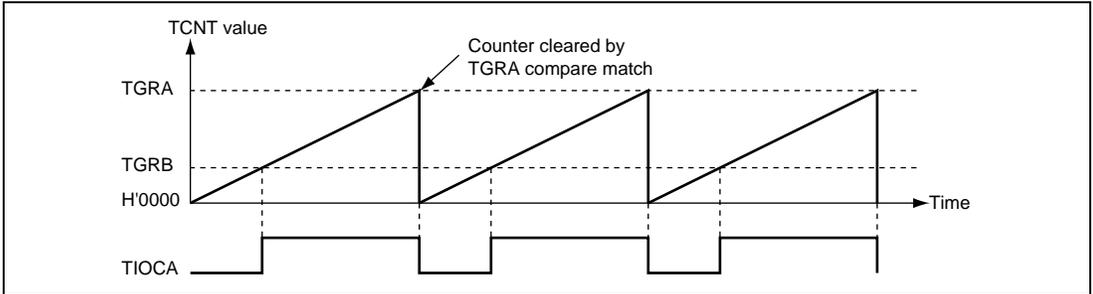
**Figure 12.18 Example of PWM Mode Operation (1)**
