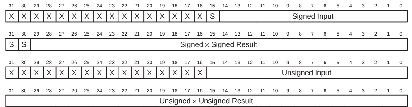
Figure 39. 16 x 16 Multiplier Data Formats
