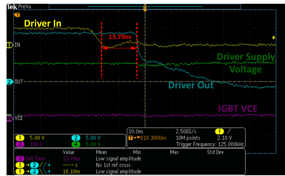
Figure 8-3. UCC27624 Used to Drive IGBT in the Boost Converter
