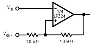
Figure 18. Non-Inverting Amplifier
