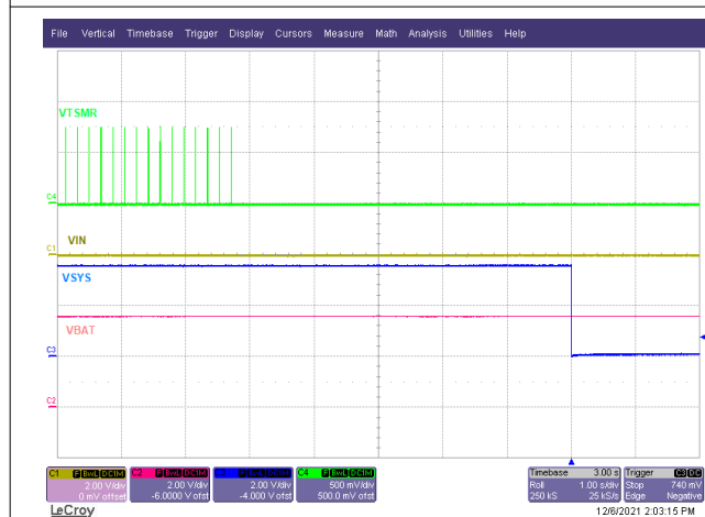
Figure 9-10. Shipmode Entry on VIN Removal
