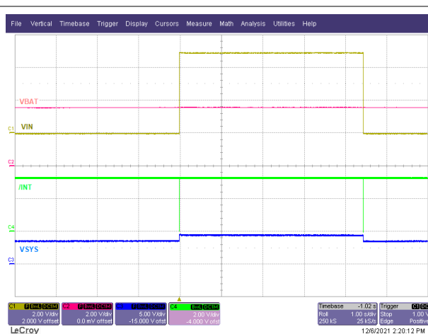
Figure 9-11. Power Good Interrupt on /INT
