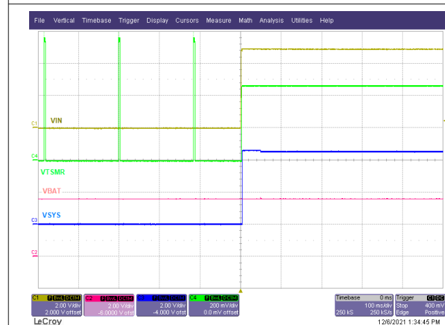
Figure 9-2. Power Up with IN Supply Insertion with No Battery
