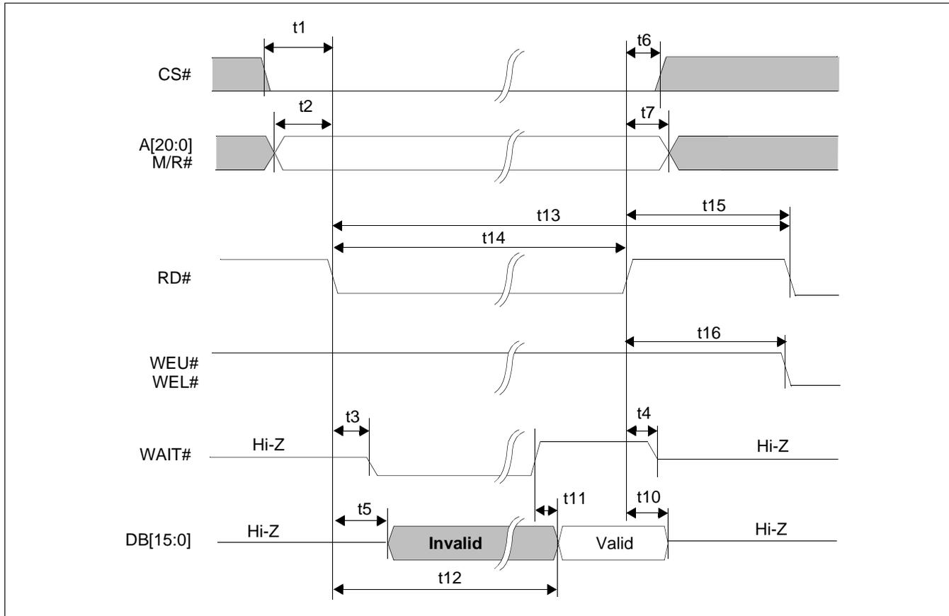
Figure 7-10: Direct/Indirect Intel 80 Type 2 Host Interface Read Timing
