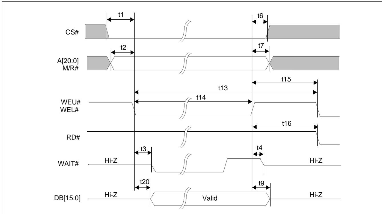
Figure 7-9: Direct/Indirect Intel 80 Type 2 Host Interface Write Timing
