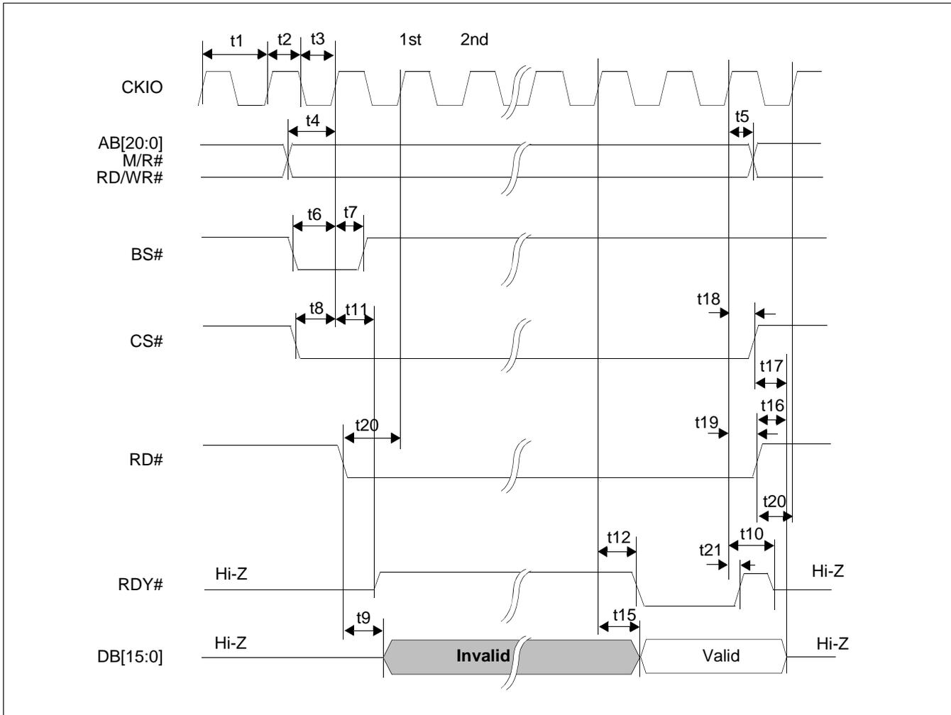
Figure 7-14: Direct/Indirect Renesas SH4 Host Interface Read Timing
