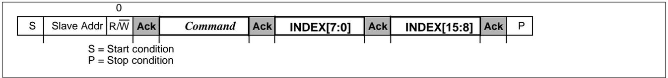
Figure 21-7: I2C Host “Write INDEX” Command Transfer Cycle
