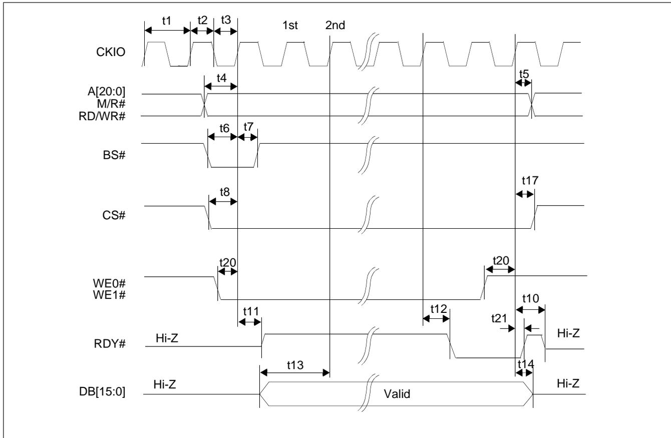
Figure 7-13: Direct/Indirect Renesas SH4 Host Interface Write Timing
