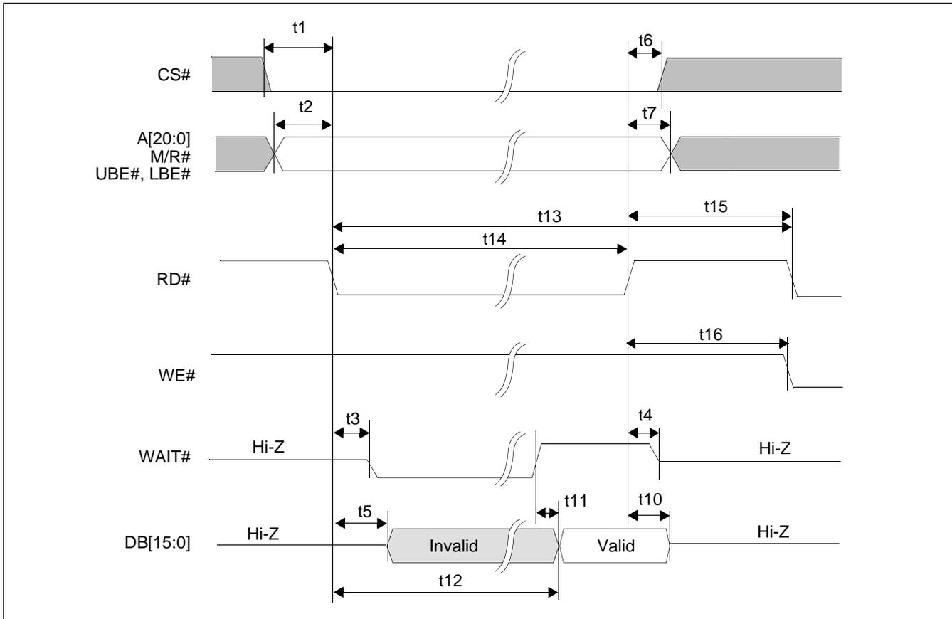
Figure 7-8: Direct/Indirect Intel 80 Type 1 Host Interface Read Timing
