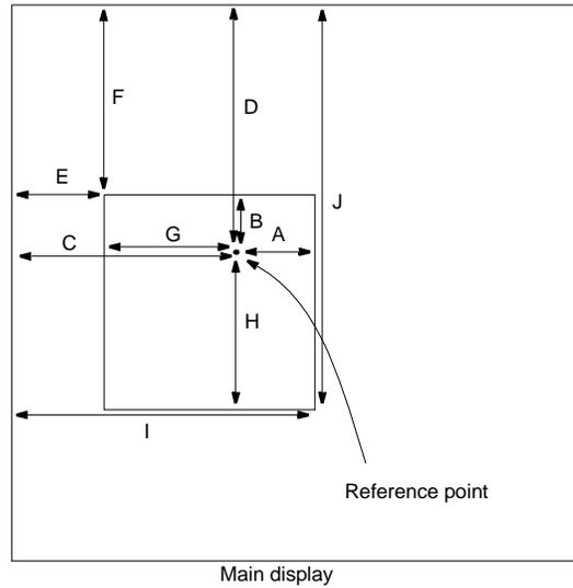
Figure 16-12: Sprite Display for Rotation 0° with Mirror Enabled
