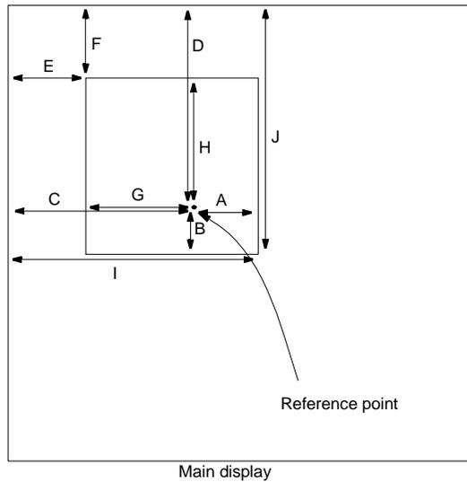
Figure 16-10: Sprite Display for Rotation 180° with Mirror Disabled
