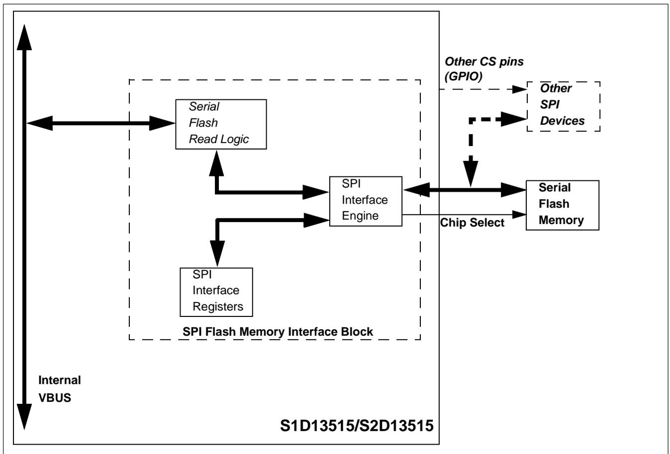
Figure 25-1: SPI Flash Memory Interface Block Diagram
