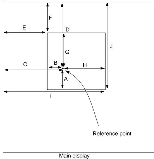
Figure 16-11: Sprite Display for Rotation 270° with Mirror Disabled
