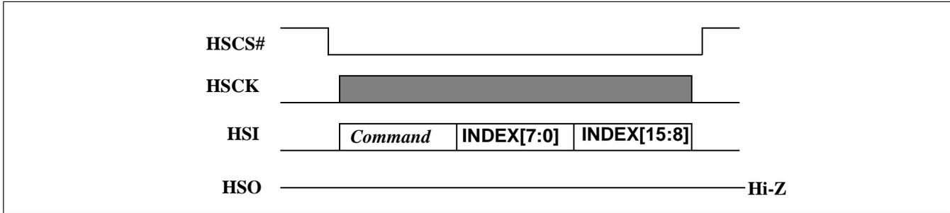
Figure 21-1: SPI Host “Write INDEX” Command Transfer Cycle
