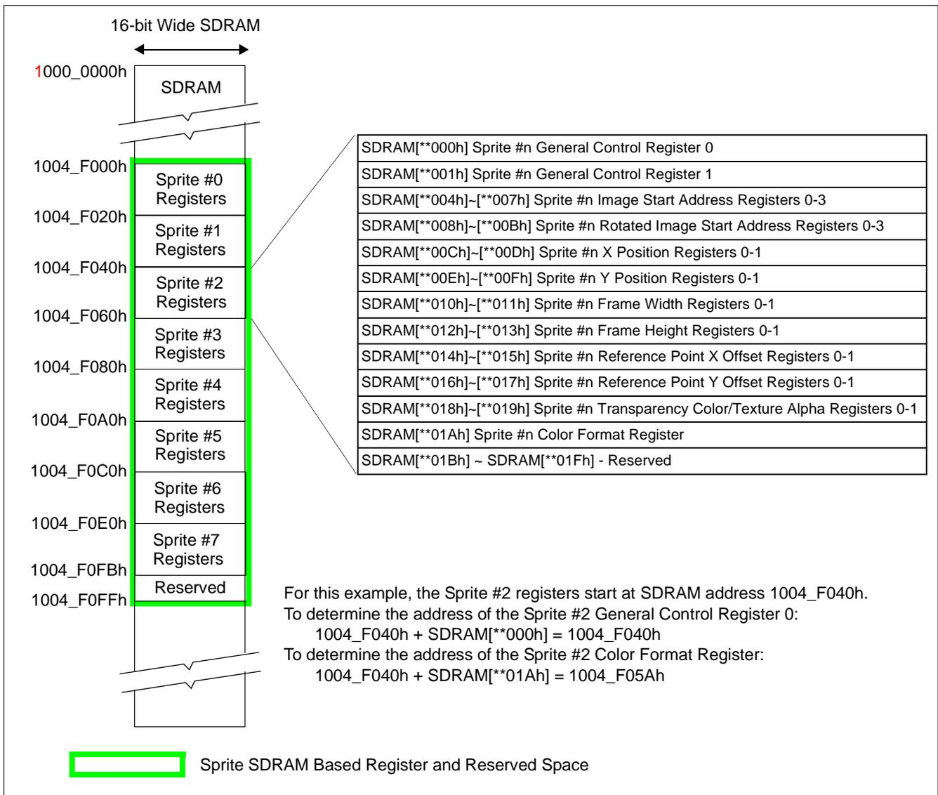
Figure 10-4: Sprite SDRAM Based Register Mapping Example
