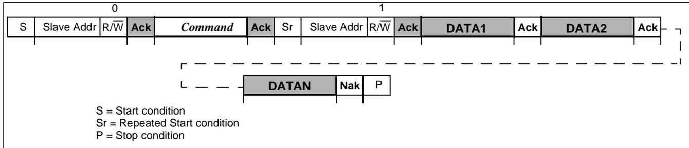
Figure 21-12: I2C Host “Read DATA” Command Transfer Cycle
