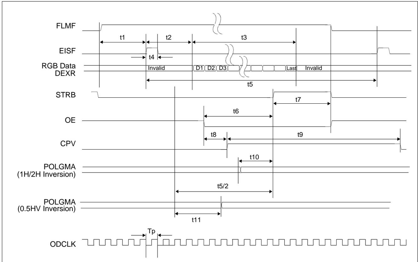
Figure 7-44: EID Double Screen Panel Horizontal Timing
