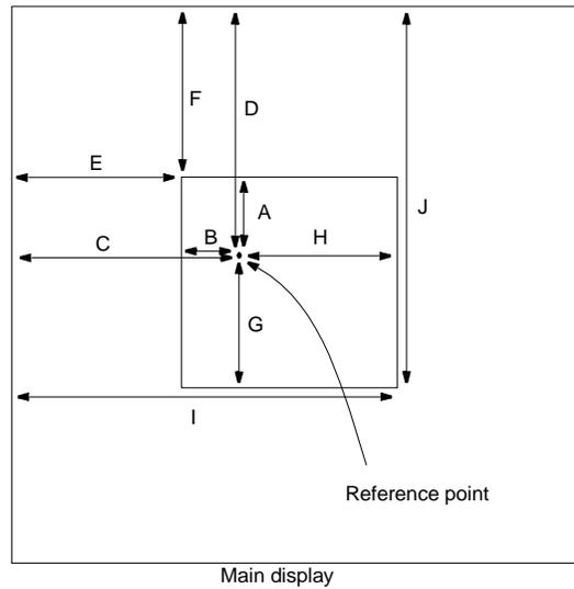
Figure 16-13: Sprite Display for Rotation 90° with Mirror Enabled
