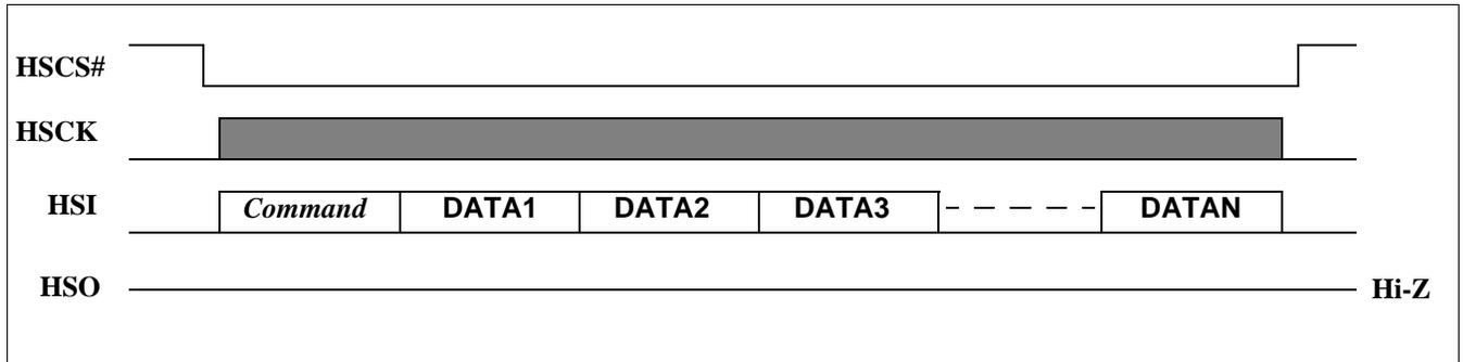
Figure 21-5: SPI Host "Write DATA" Command Transfer Cycle
