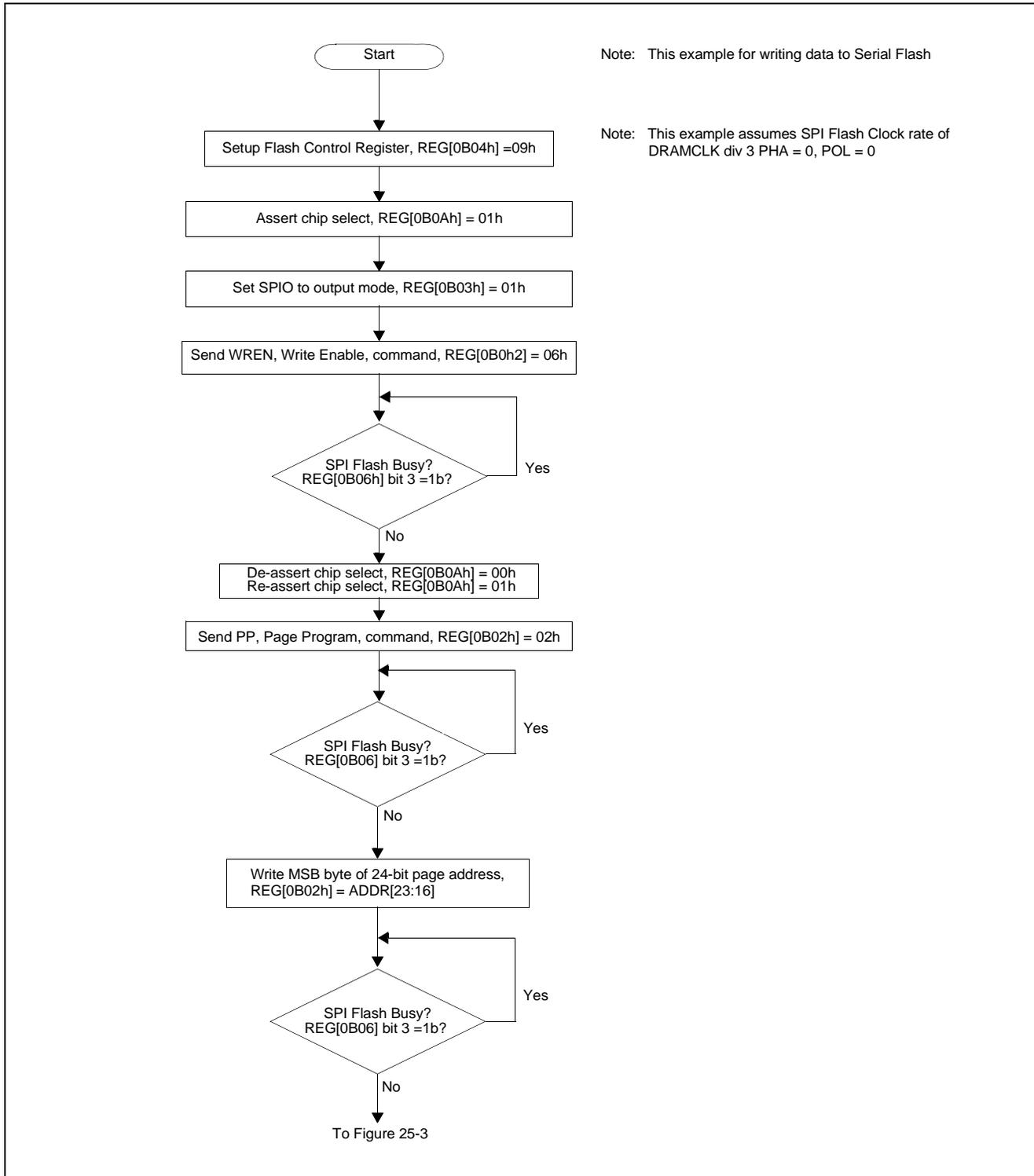
Figure 25-2: Typical SPI Interface Write Operation Flow
