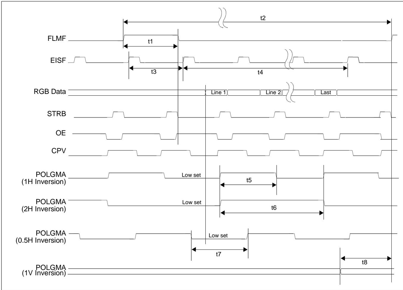
Figure 7-45: EID Double Screen Panel Vertical Timing
