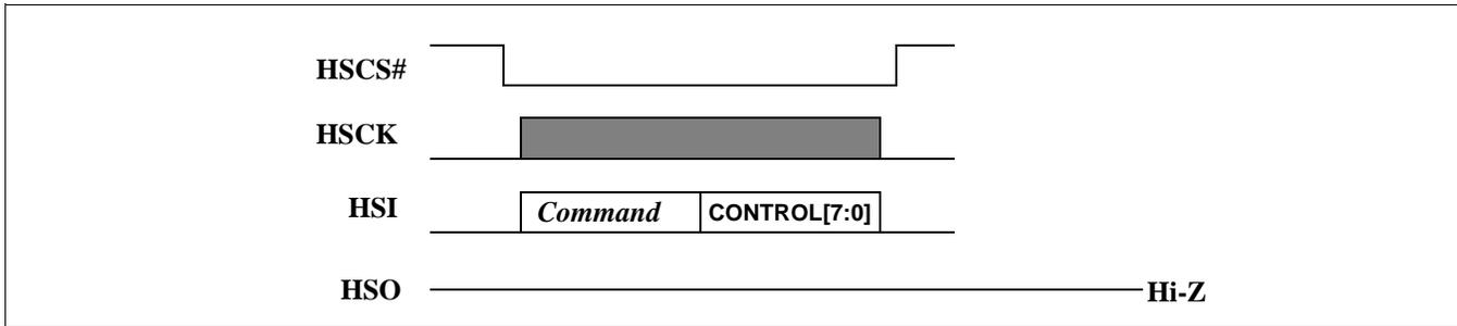
Figure 21-3: SPI Host “Write CONTROL” Command Transfer Cycle
