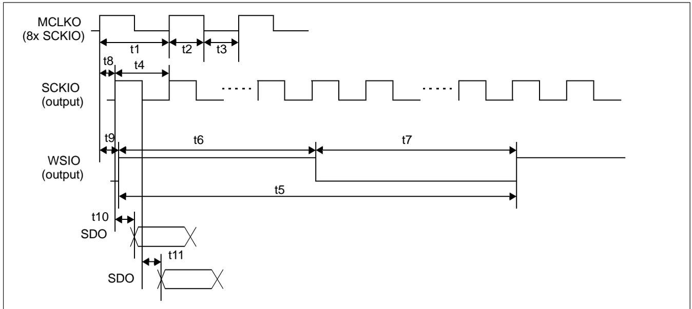
Figure 7-49 I2S Timing when SCKIO/WSIO are Outputs
