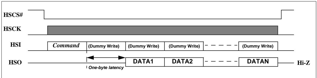
Figure 21-6: SPI Host "Read DATA" Command Transfer Cycle
