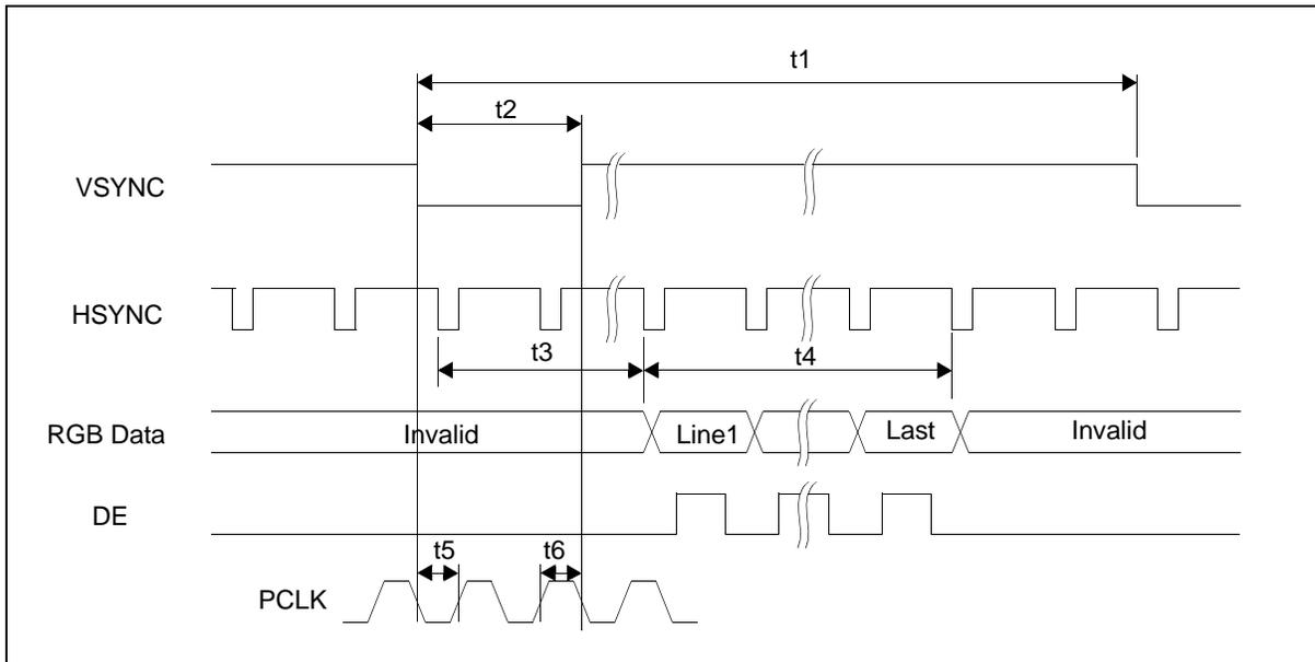
Figure 7-31: Generic RGB Type Interface Panel Vertical timing
