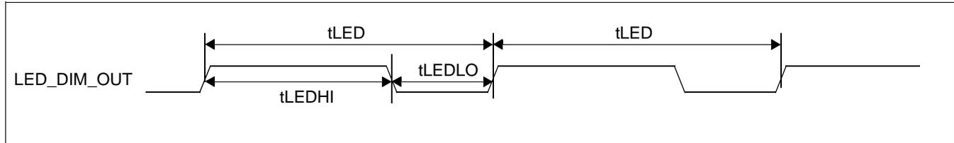
Figure 7-41: EID Double Screen Panel LED\_DIM\_OUT Timing
