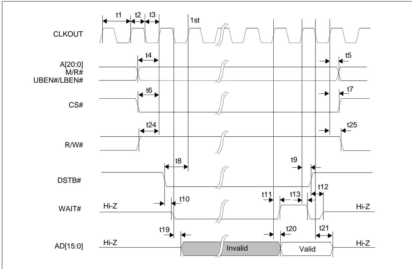
Figure 7-24: Direct/Indirect NEC V850 Type 1 Host Interface Read Timing
