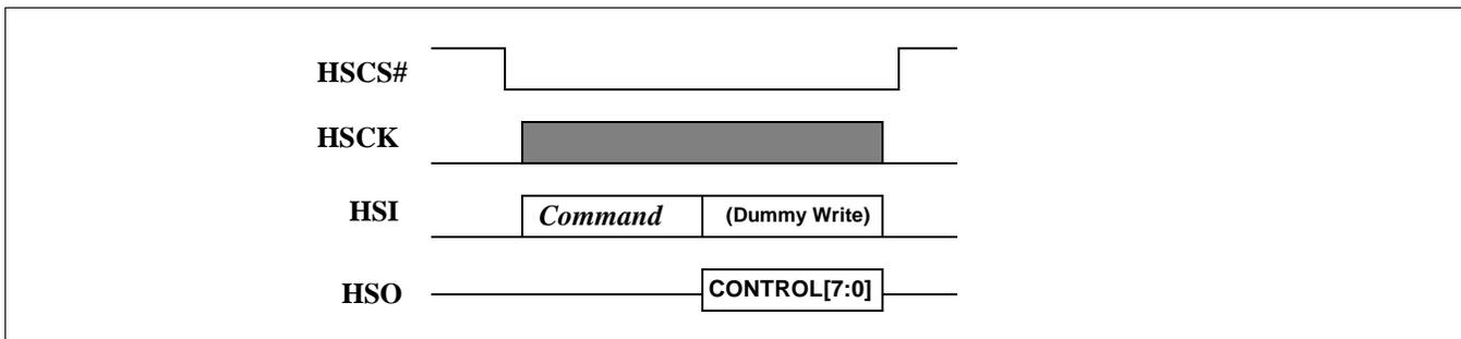
Figure 21-4: SPI Host “Read CONTROL” Command Transfer Cycle
