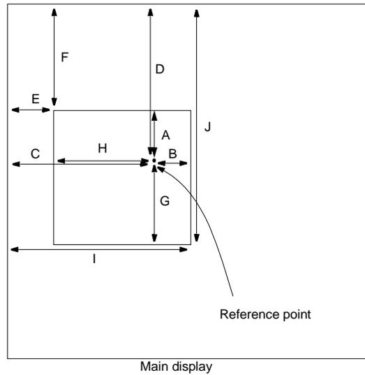
Figure 16-9: Sprite Display for Rotation 90° with Mirror Disabled
