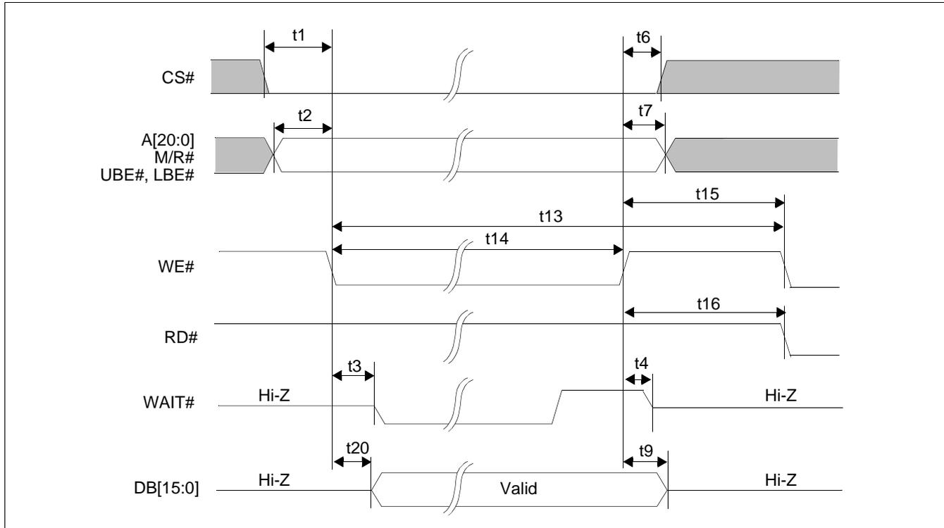
Figure 7-7: Direct/Indirect Intel 80 Type 1 Host Interface Write Timing
