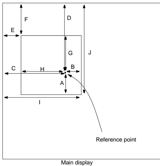
Figure 16-15: Sprite Display for Rotation 270° with Mirror Enabled
