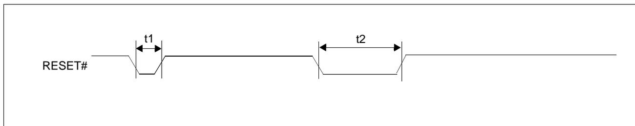
Figure 7-6 RESET# Timing
