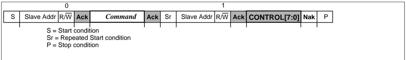
Figure 21-10: I2C Host “Read CONTROL” Command Transfer Cycle
