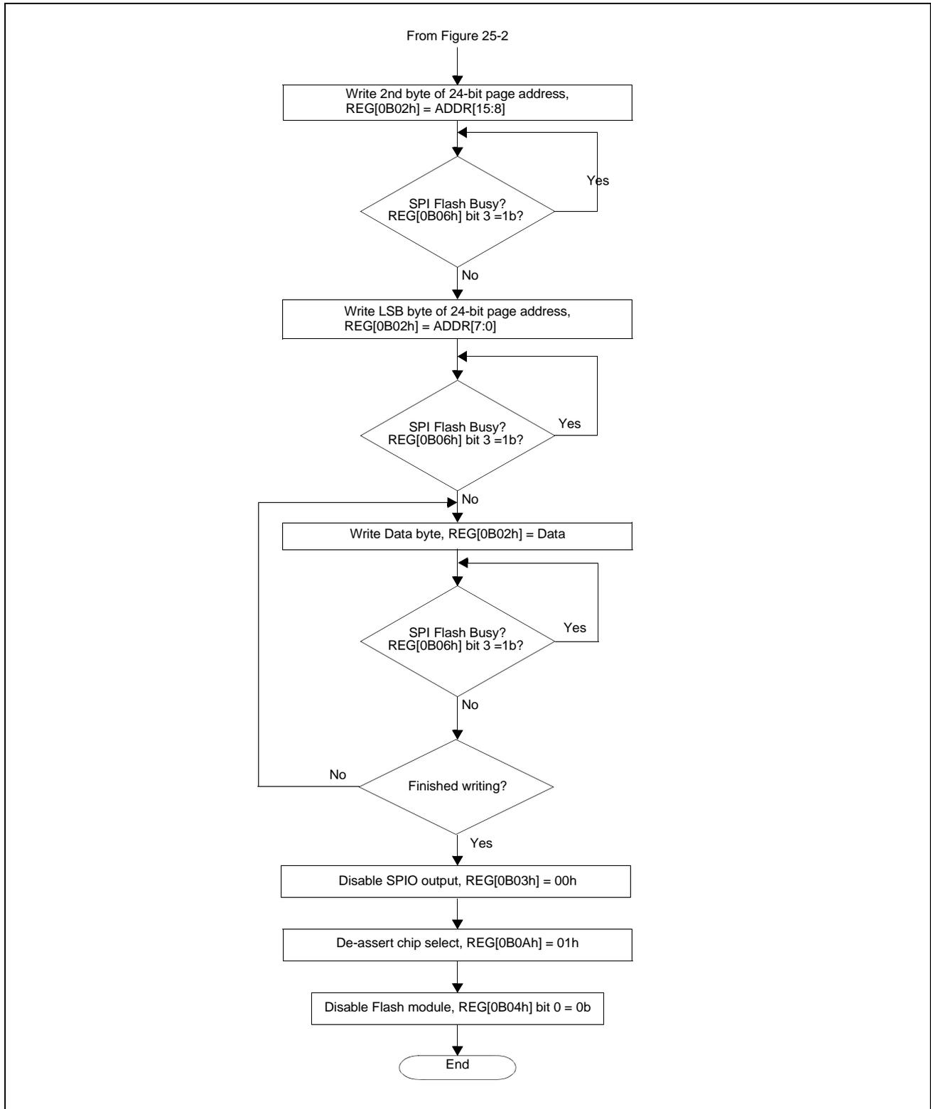
Figure 25-3: Typical SPI Interface Write Operation Flow (Continued)
