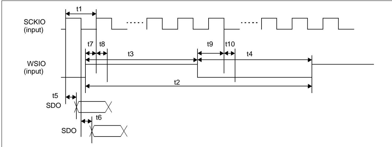
Figure 7-50 I2S Timing when SCKIO/WSIO are Inputs
