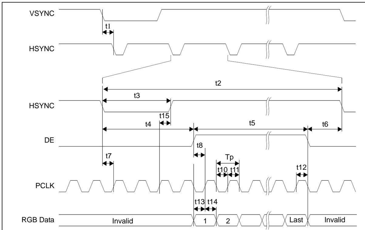
Figure 7-30: Generic RGB Type Interface Panel Horizontal Timing
