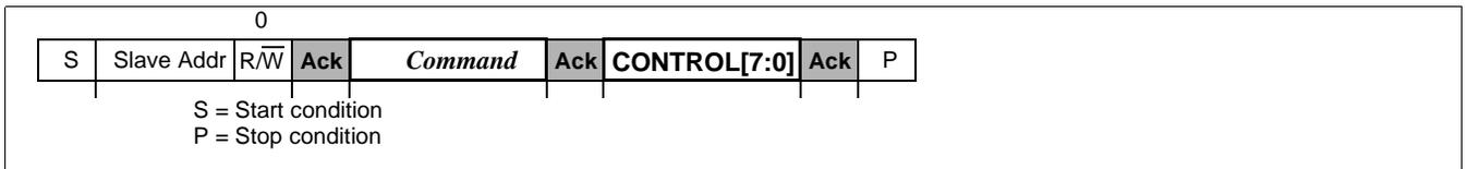
Figure 21-9: I2C Host “Write CONTROL” Command Transfer Cycle
