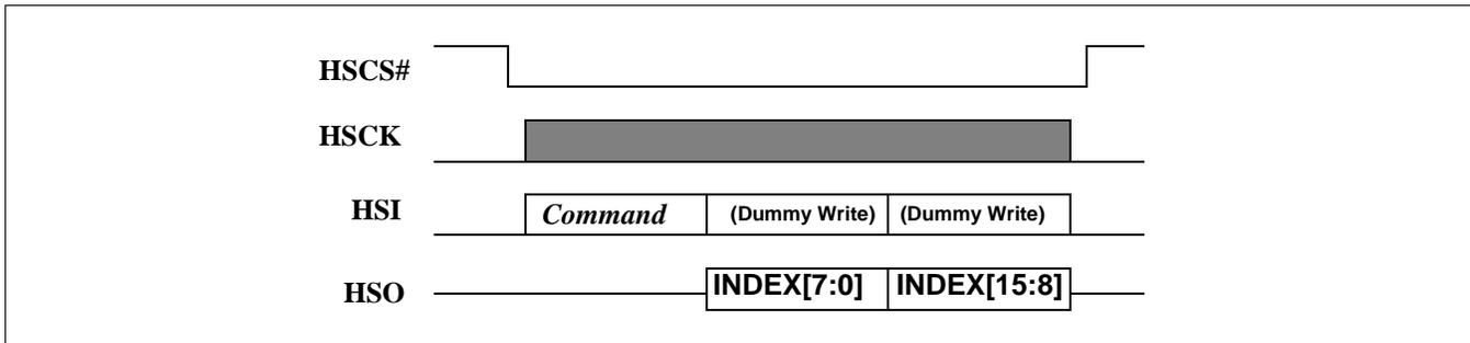
Figure 21-2: SPI Host “Read INDEX” Command Transfer Cycle
