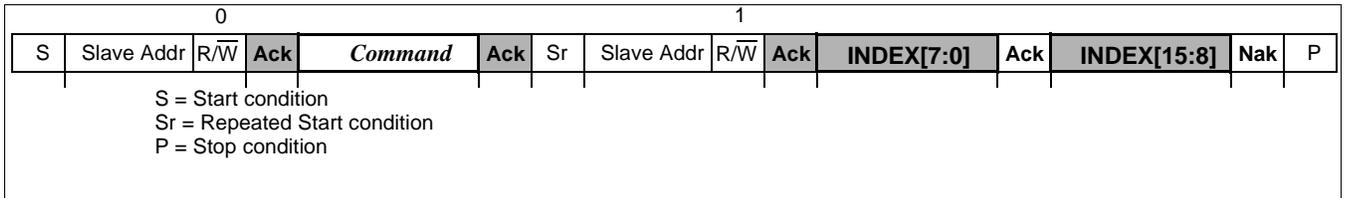
Figure 21-8: I2C Host “Read INDEX” Command Transfer Cycle
