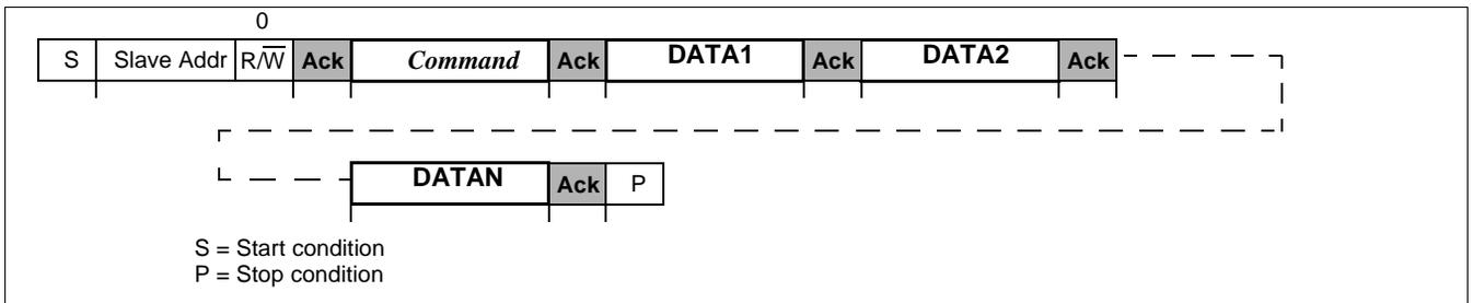
Figure 21-11: I2C Host “Write DATA” Command Transfer Cycle
