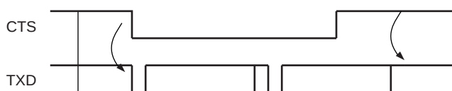
Figure 36-28. Transmitter Behavior when Operating with Hardware Handshaking
