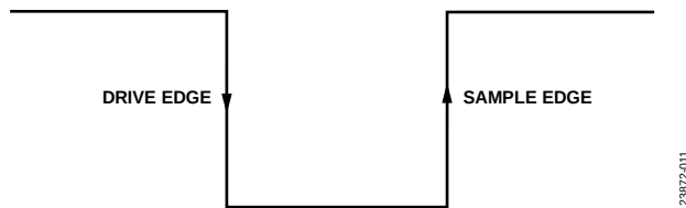
Figure 21. SPI Mode 3 SCLK Edges
