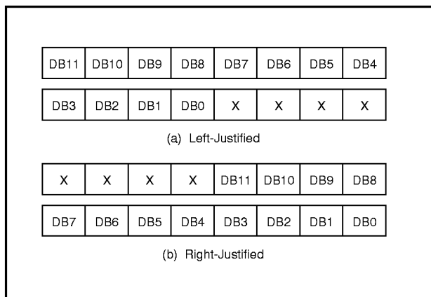
FIGURE 9. 12-Bit Data Formats for 8-Bit Systems.
