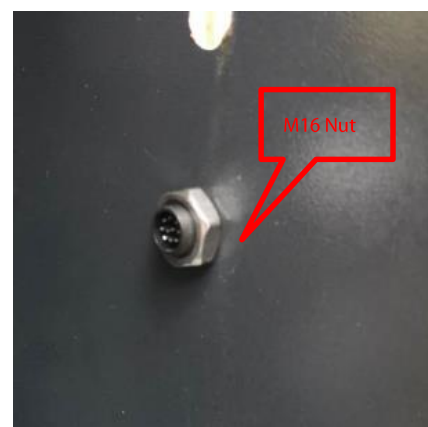
(b) The wiring connection passes through the gasket and nut
