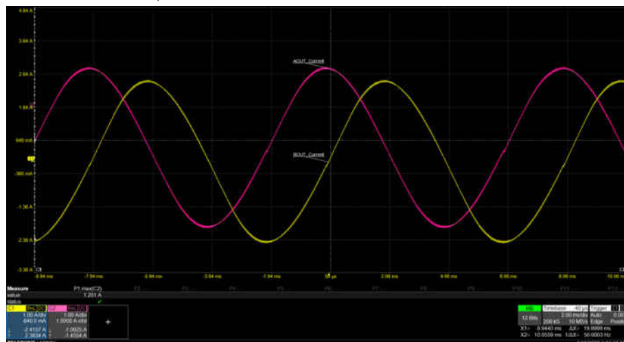
Figure 7-20. Coil Current Waveform with Silent Step Decay
