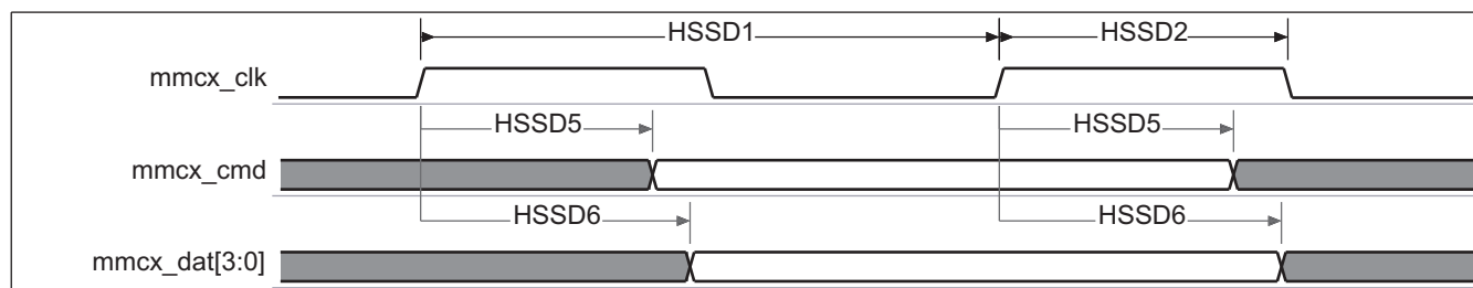
Figure 6-66. MMC/SD/SDIO – High-Speed SD Mode – Data/Command Transmit
