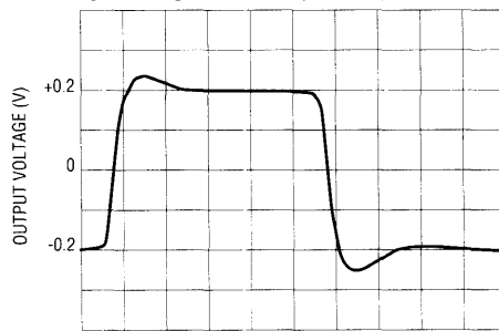
Small Signal Pulse Response (Split Supply) V_S = \pm 2.5V , R_L = 150\Omega to 0V , R_F = 1K\Omega , A_V = +2
