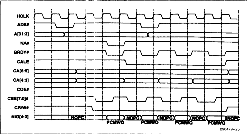
Figure 23. Burst Write to Second Level Cache with Dual-Byte Select Standard SRAMs (82434LX)
