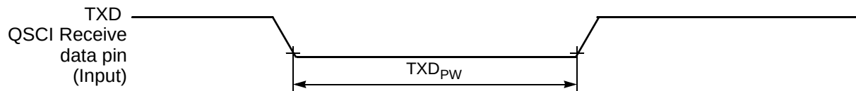
Figure 10-13 TXD Pulse Width
