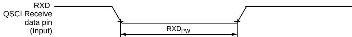
Figure 10-12 RXD Pulse Width
