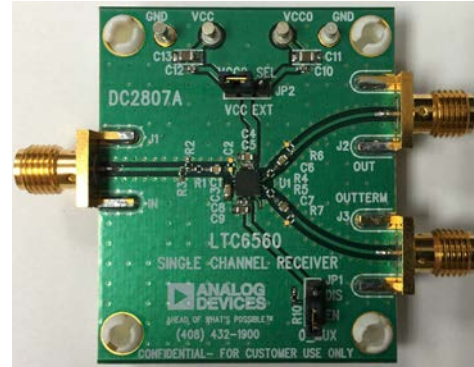
Figure 16. DC2807A Single Channel Electrical Evaluation Board
