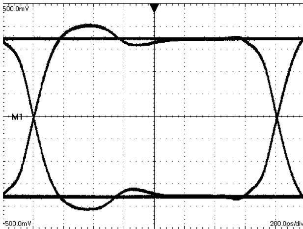
Figure 10. A 622 Mbps NRZ PRBS-7 Output Eye Diagram
