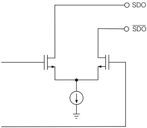
Figure 2-6: Serial Digital Output (GS1560A only)
