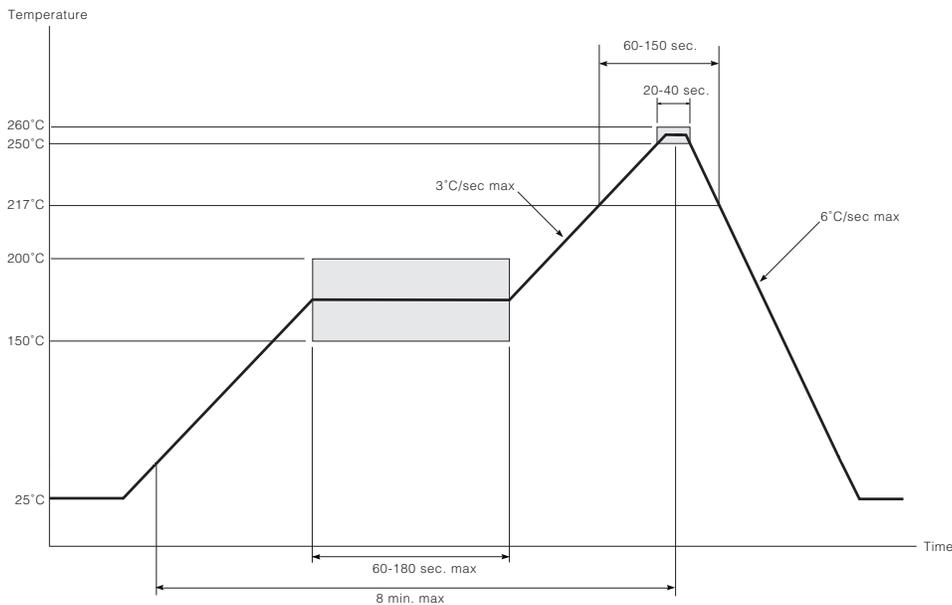
Figure 2-2: Maximum Pb-free Solder Reflow Profile (Pb-free package)
