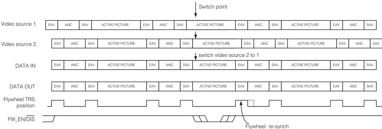
**Figure 3-2: Switch Line Locking**
