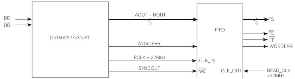
Figure 3-4: DVB-ASI FIFO Implementation Using The GS1560A
