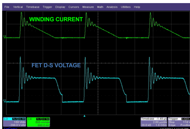
FIGURE 14. QUASI-RESONANT NEAR-ZVS SWITCHING
